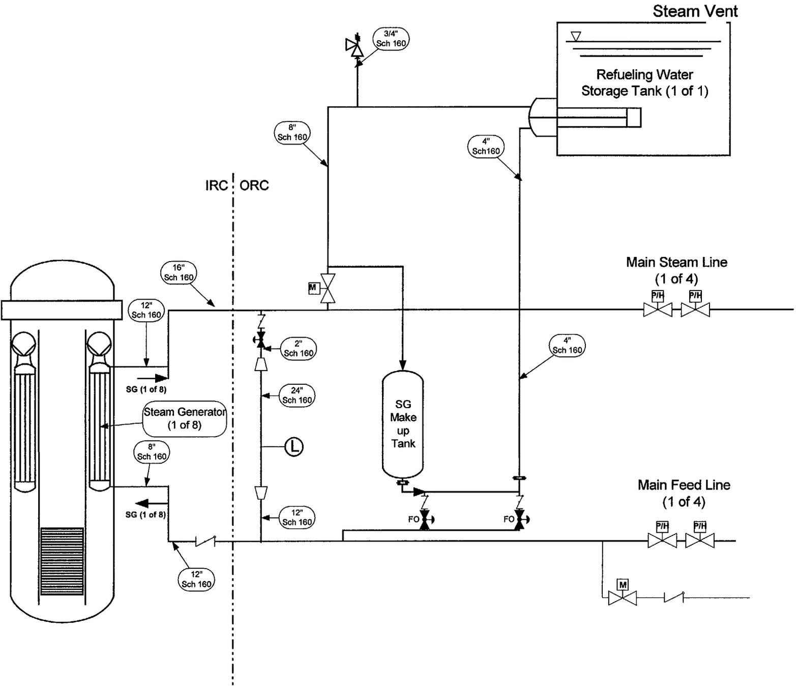
Figure 4.2-1 IRIS Emergency Heat Removal System (EHRS) Simplified Sketch
