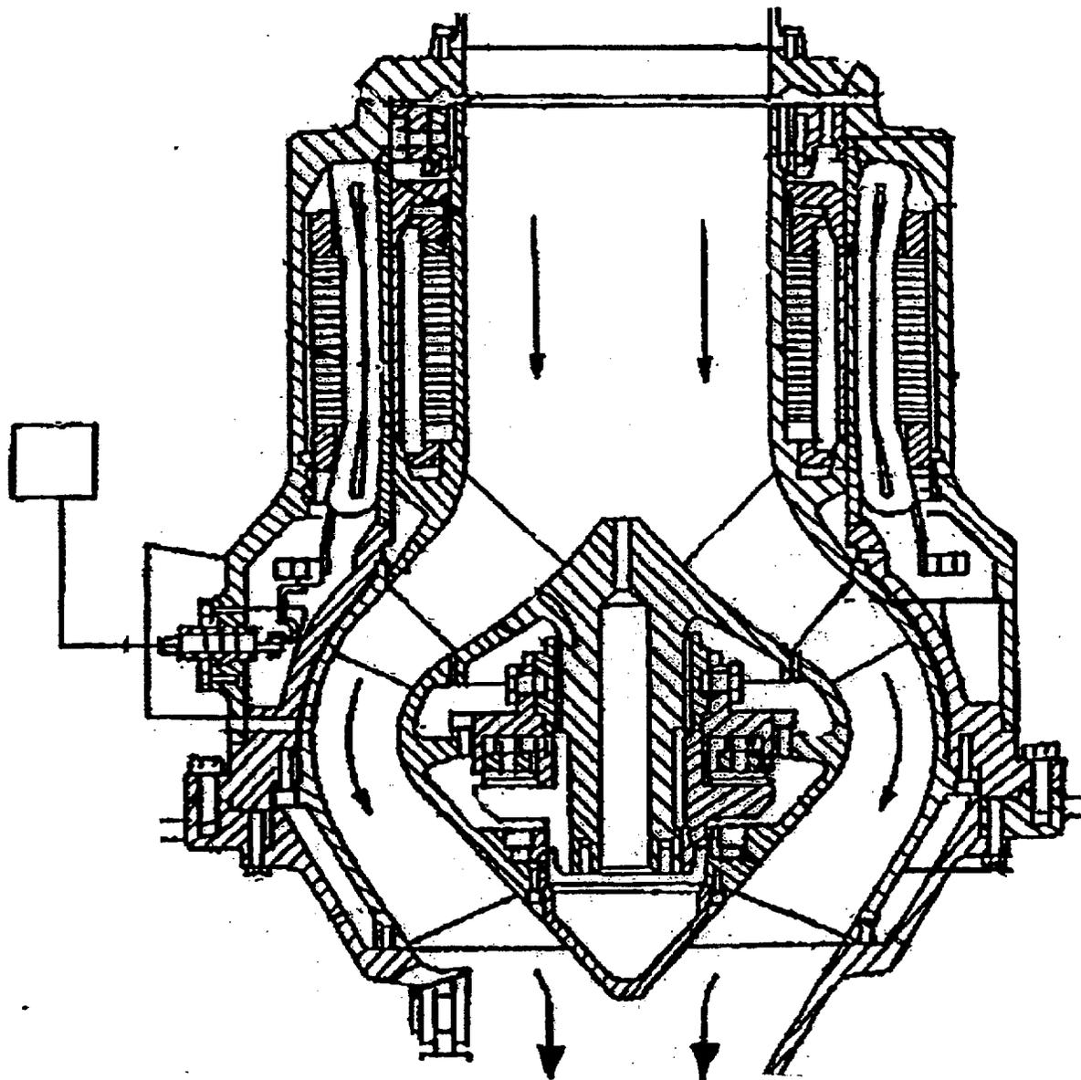
**Figure 3.4-3 Example of Spool-type Pump with Mixed Flow Hydraulics**
