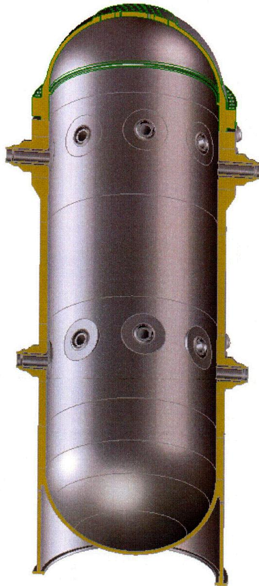
**Figure 3.3-13 Upper Core Support Structure**
