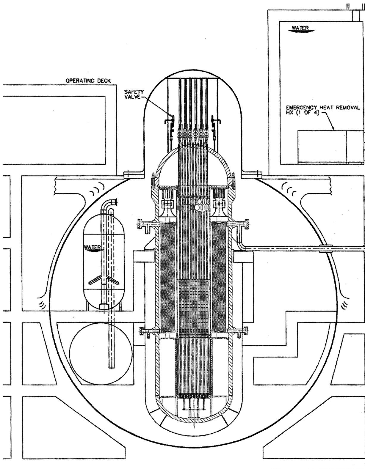
Figure 1.1-1 IRIS Spherical Steel Containment and Major Components
