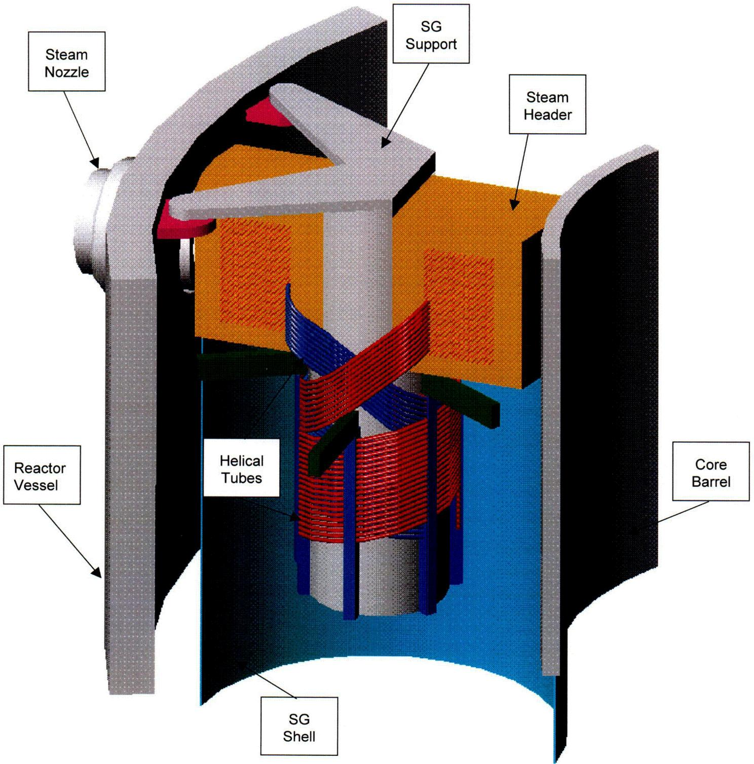
Figure 3.5-3 3D Representation of an IRIS SG module
