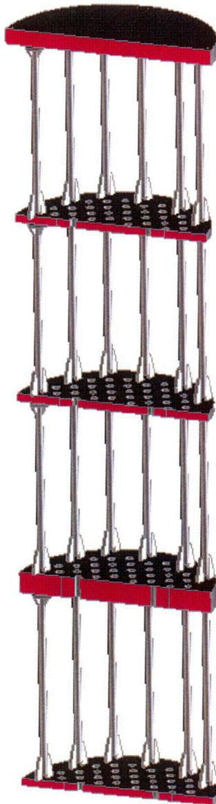
**Figure 3.3-12 Upper Core Support Structure**
