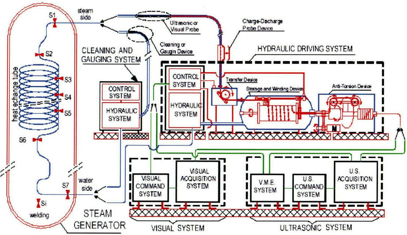
Figure 3.5-4 Helical Coil Steam Generator Inspection System
