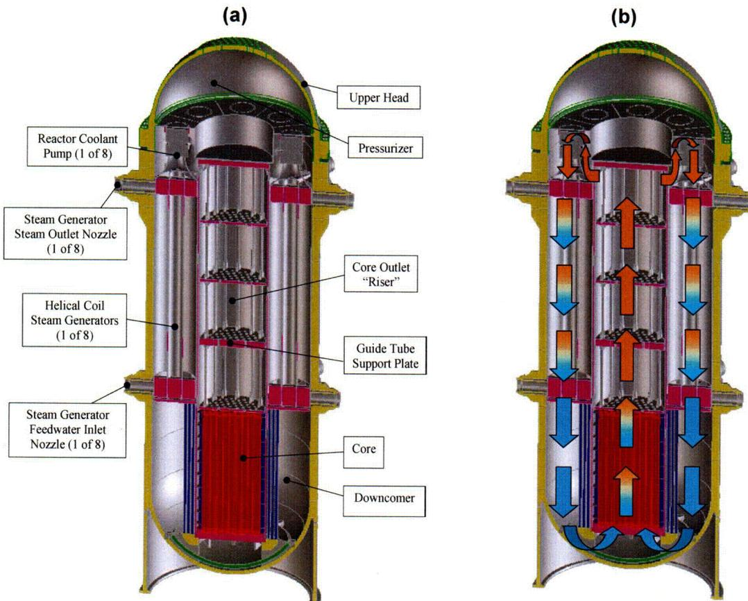
**Figure 3.1-1: IRIS integral layout: (a) main components; (b) main flow path**
