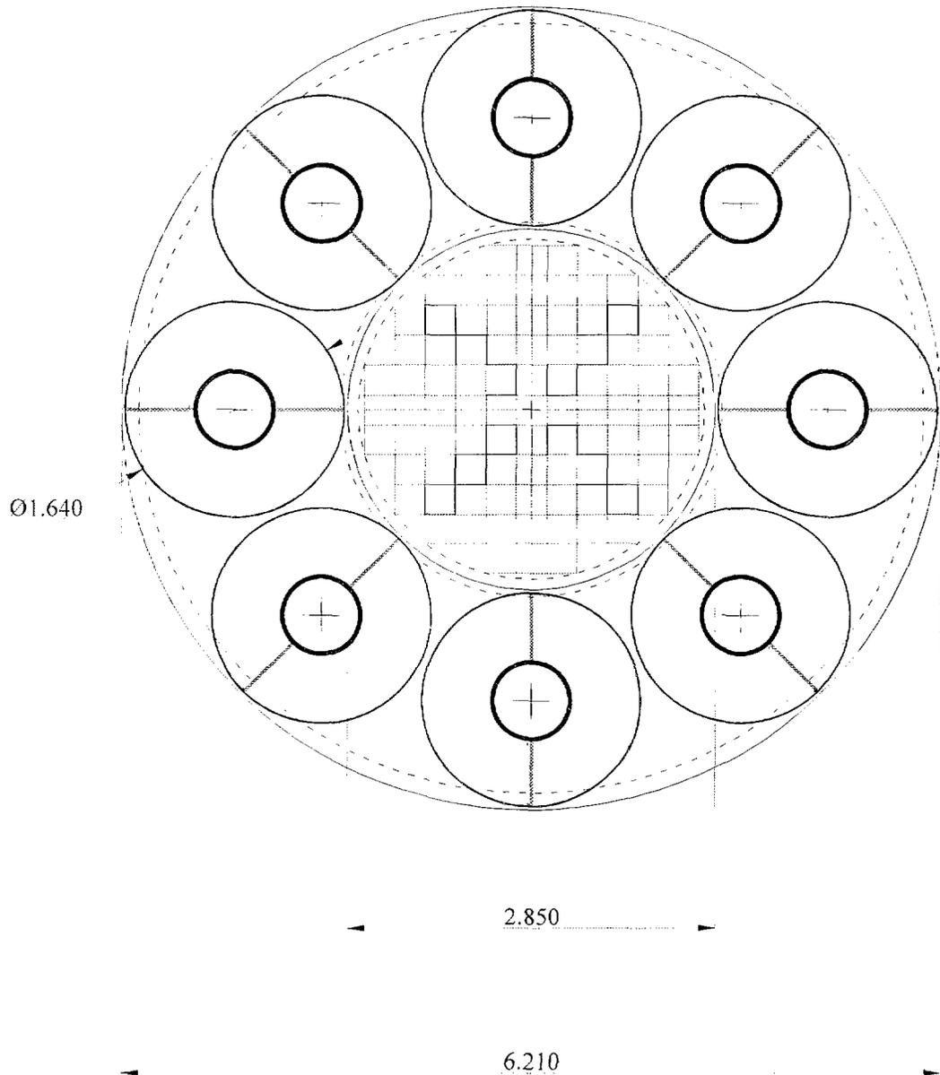
**Figure 3.5-1 IRIS SGs layout in the Integral Reactor Coolant System**
