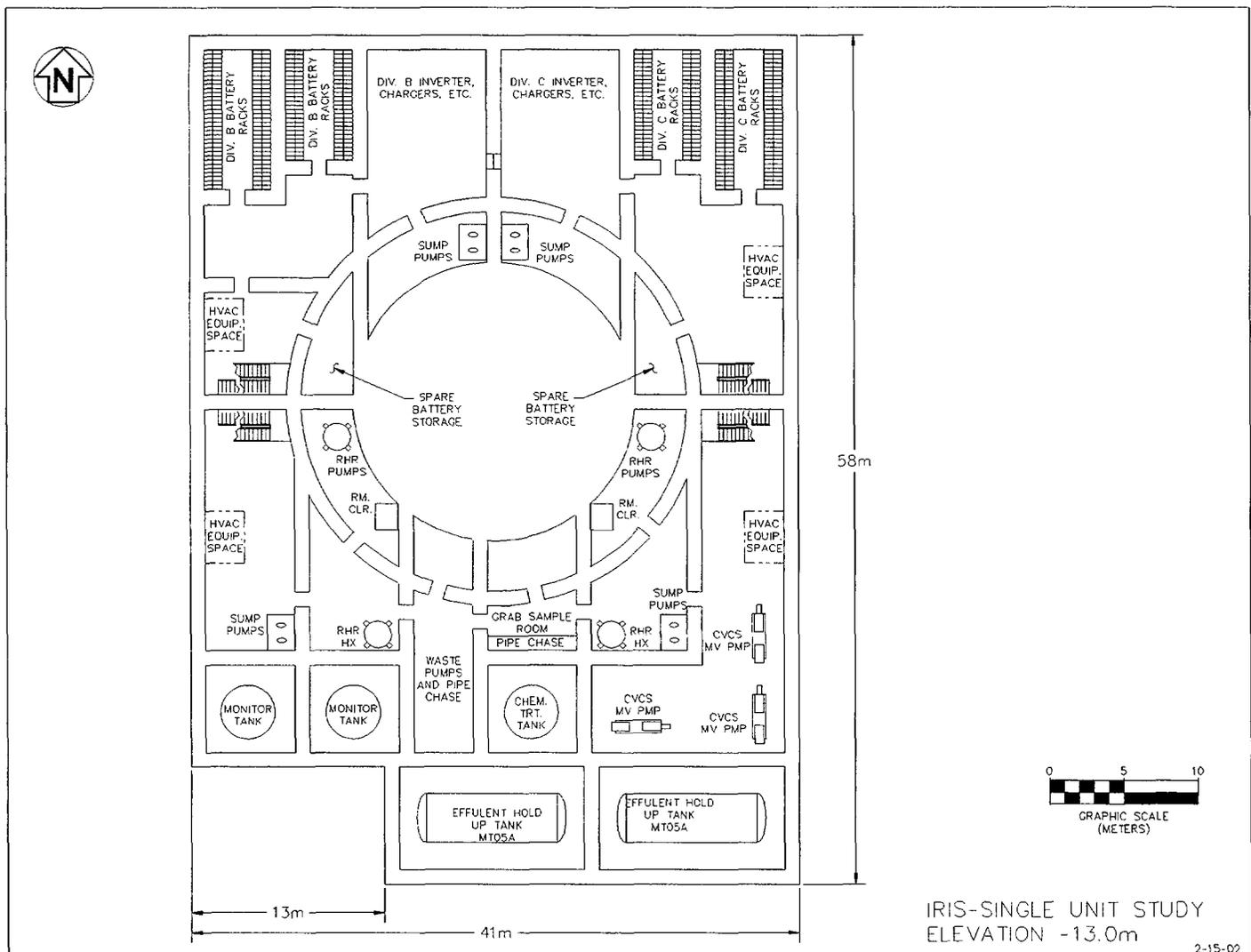
**Figure 6.3-1, IRIS Auxiliary Building General Arrangement at Elevation -13 Meters**
