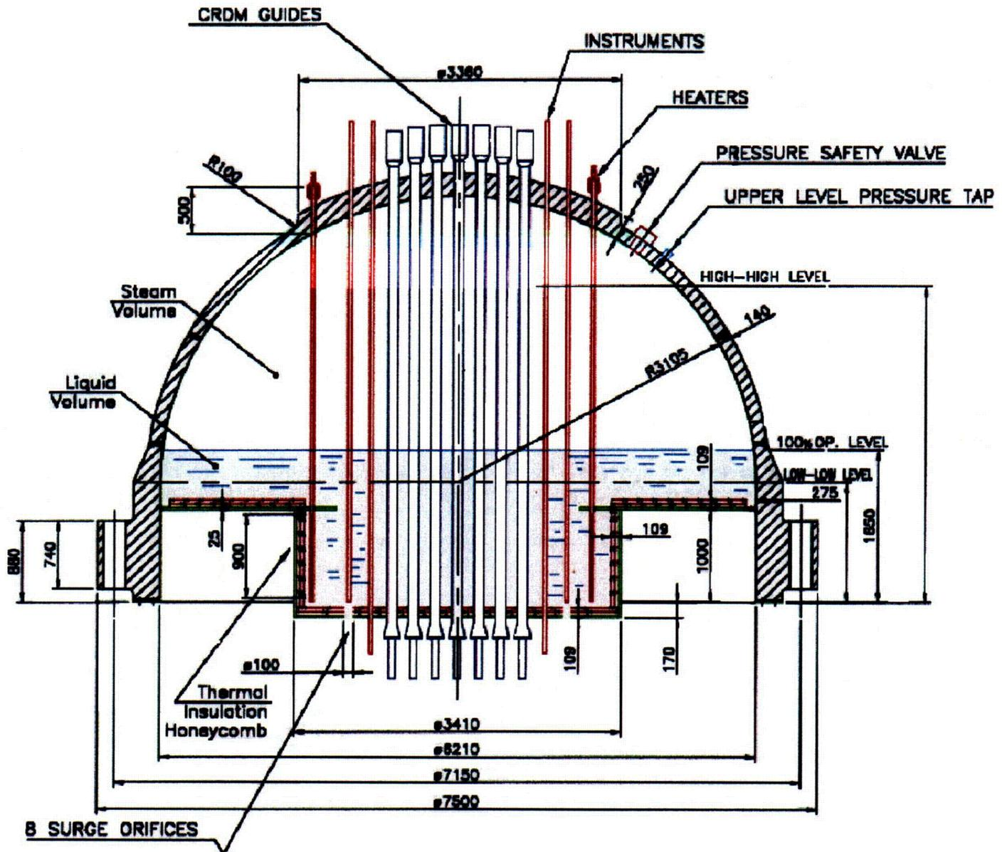
Figure 3.6-2 IRIS Pressurizer simplified drawing
