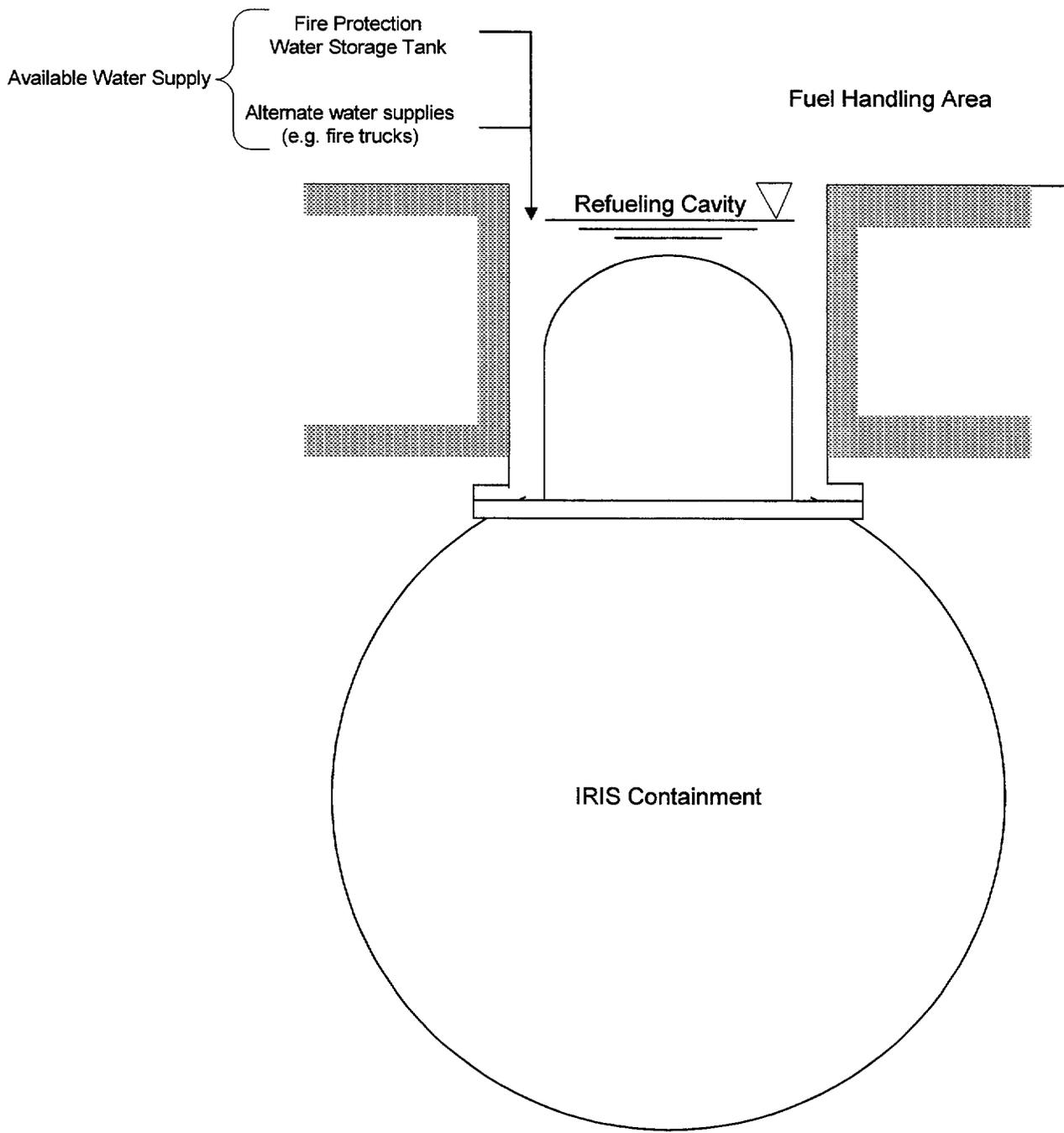
**Figure 4.7-1 IRIS Passive Containment Cooling System Simplified Sketch**
