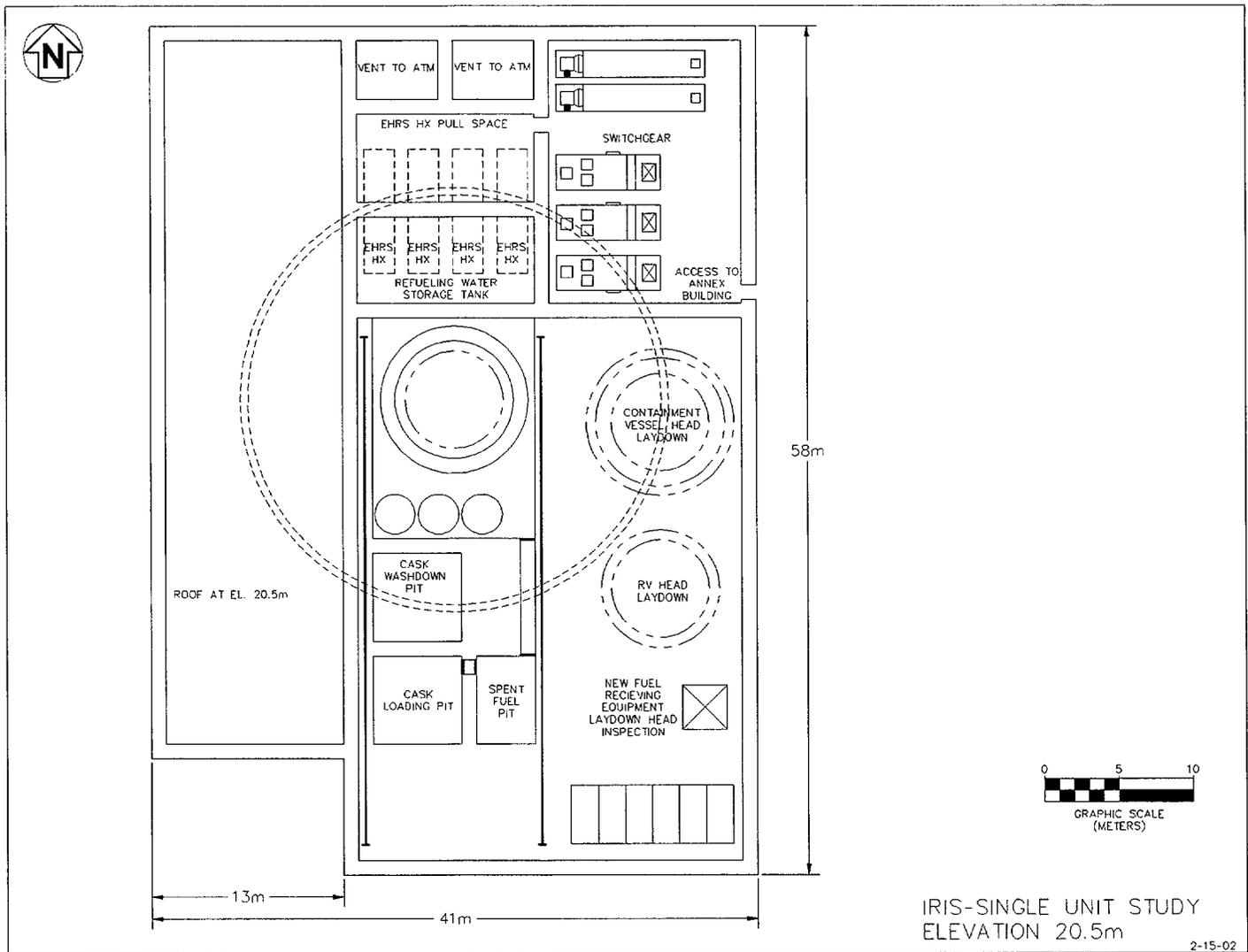
**Figure 6.3-2, IRIS Auxiliary Building General Arrangement at Elevation +20.5 Meters**
