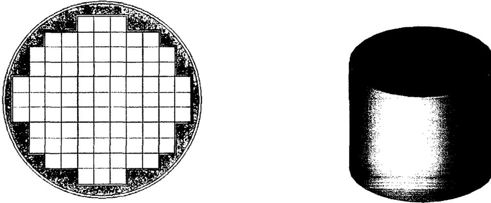
**Figure 3.2-3 IRIS radial neutron reflector assembly (conceptual)**
