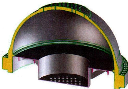
**Figure 3.3-10 IRIS Reactor Vessel Upper Head and Pressurizer volume**
