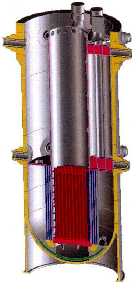
Figure 3.3-11 Lower Core Support Structure
