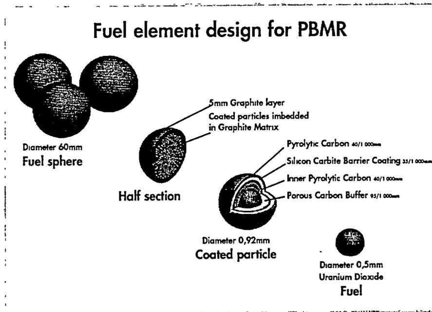
The PBMR fuel is based on proven high quality German moulded graphite sphere and triple coated particles (TRISO). Essentially, the fuel elements are multi-layer spheres consisting of enriched uranium and various forms of carbon.
