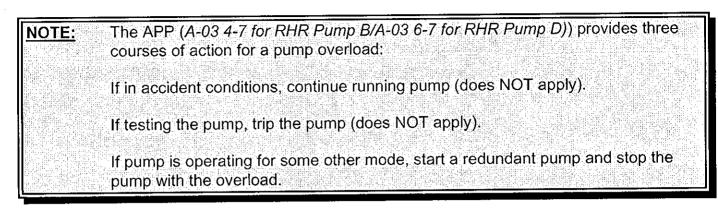
Step 12 – Refer to APP for RHR Pump (B or D) overload Refers to APP for RHR Pump (B or D) overload
