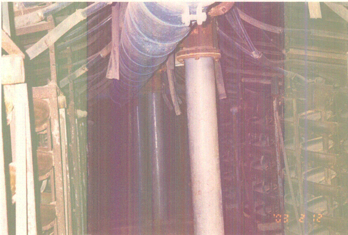
Wet Mill - Second deck, spiral feed hoses, iron vertical feed lines and horizontal manifold.
