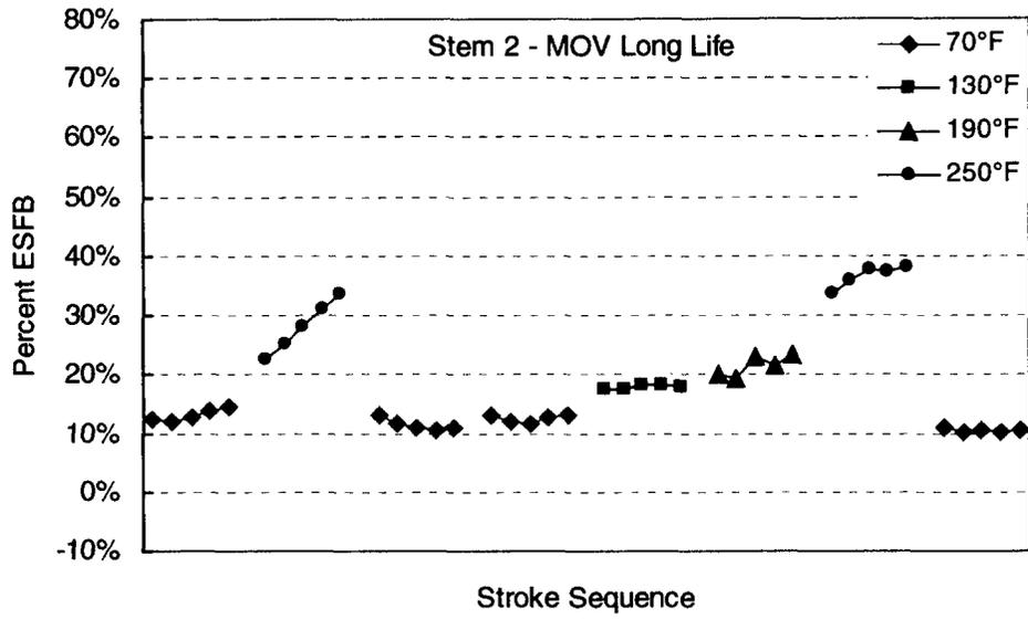
Figure 15. End-of-stroke friction behavior at elevated temperature for Stem 2 with MOV Long Life.
