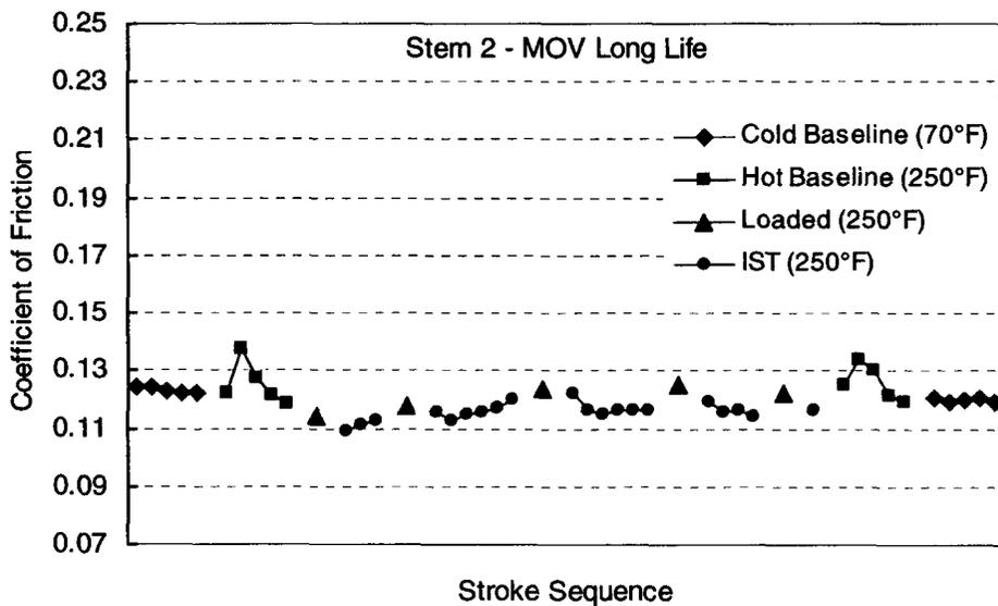
Figure 16. Aging test stroke sequence for Stem 2 with MOV Long Life.
