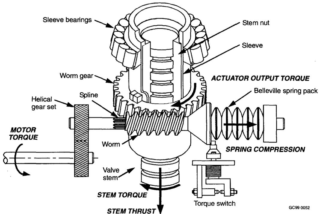
Figure 1. Diagram of the main components inside an actuator gearbox.
