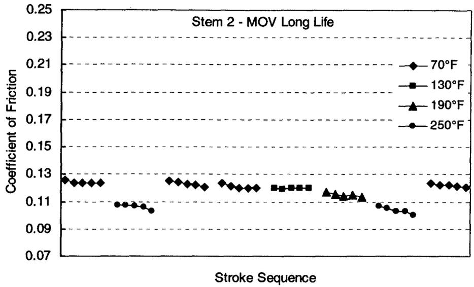
Figure 13. Running stem nut friction at elevated temperature for Stem 2 with MOV Long Life.
