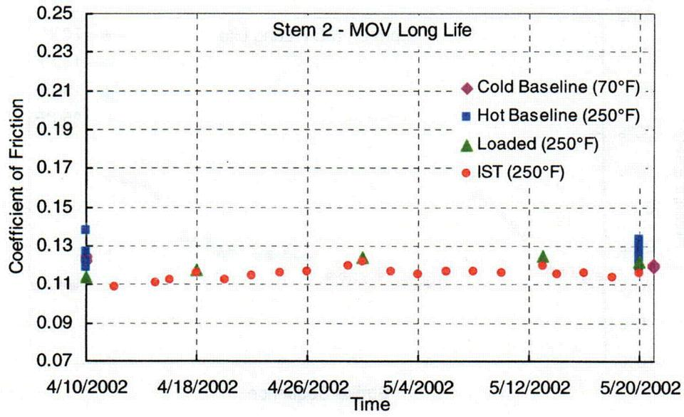
Figure 17. Aging test time line for Stem 2 with MOV Long Life.
