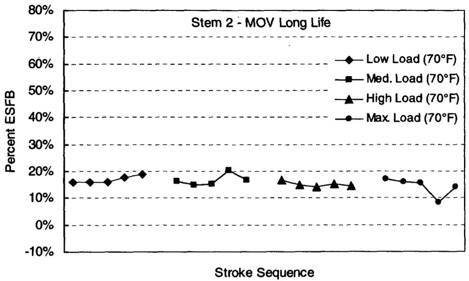
Figure 12. End-of-stroke friction behavior at various loads for Stem 2 with MOV Long Life.
