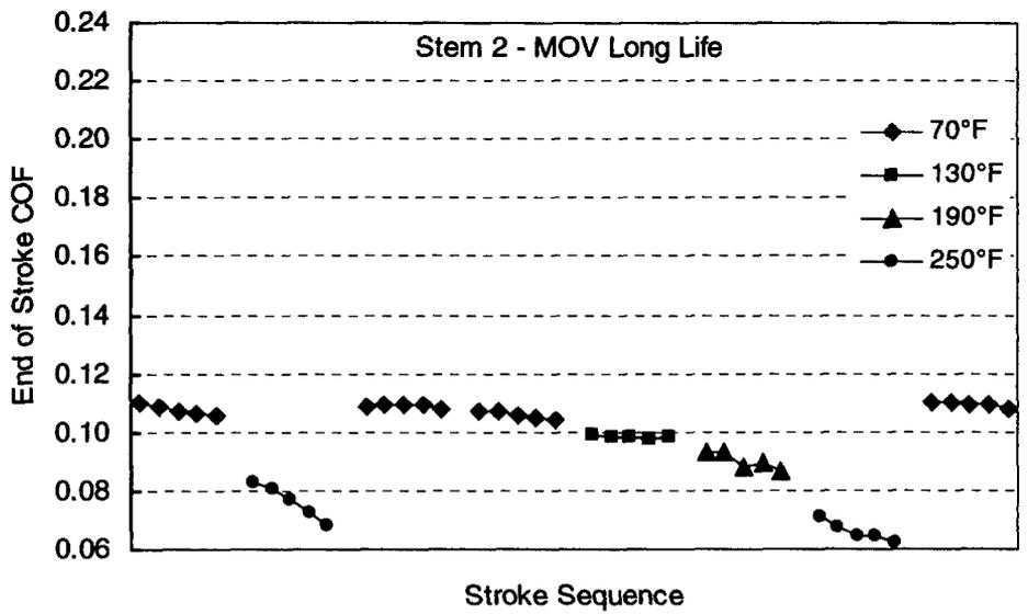
Figure 14. End-of-stroke stem nut friction at elevated temperature for Stem 2 with MOV Long Life.
