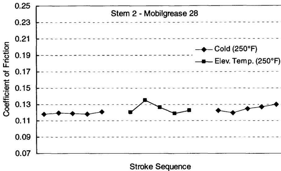
Figure 10. Elevated temperature test for Stem 2 with Mobil Mobilgrease 28.
