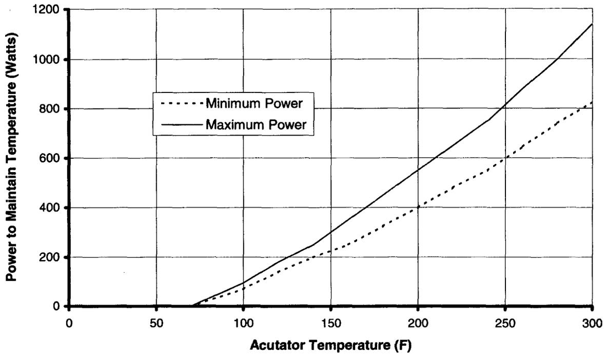
Figure 4. Power requirements to maintain actuator temperature.
