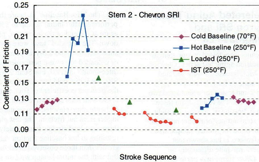
Figure 5. Aging test stroke sequence for Stem 2 with Chevron SRI.
