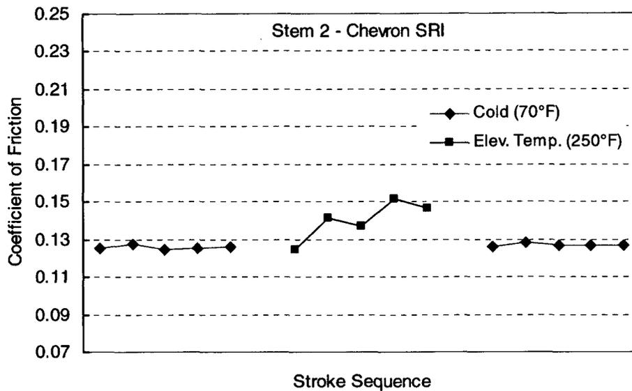
Figure 7. Elevated temperature test for Stem 2 with Chevron SRI.
