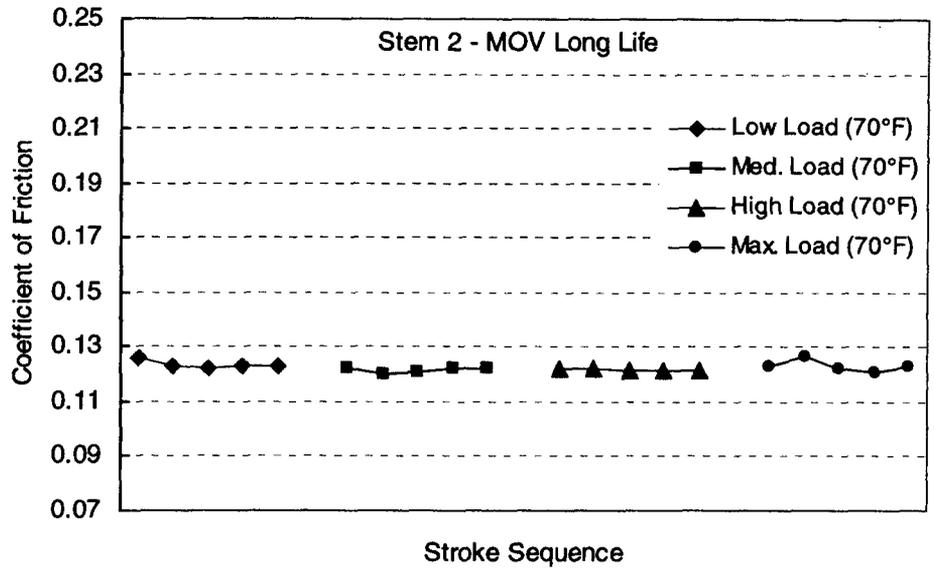
Figure 11. Stem nut friction at various stem loads for Stem 2 with MOV Long Life.
