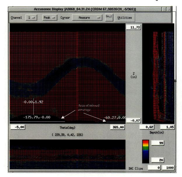
Figure 1: Typical RPV Nozzle UT Inspection "C" Scan with area of missed coverage identified by arrows and above the white horizontal line.
