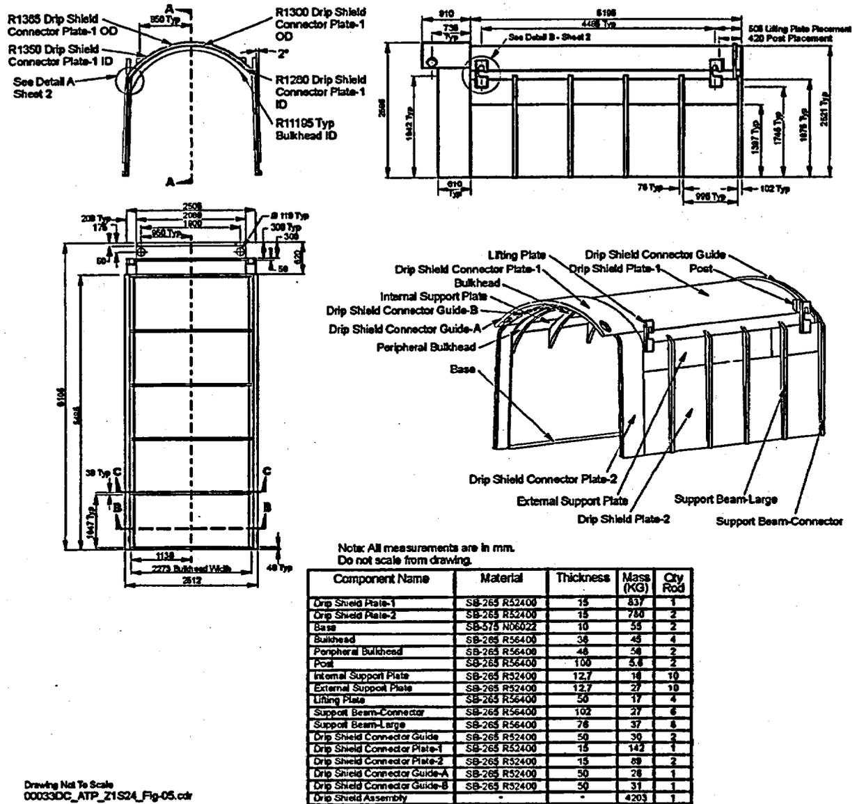
Figure 2-75. Drip Shield Structural Components
