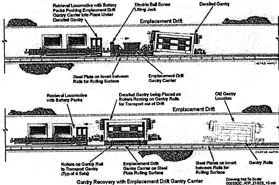
**Figure 2-60. Gantry Recovery with Emplacement Drift Gantry Carrier**
