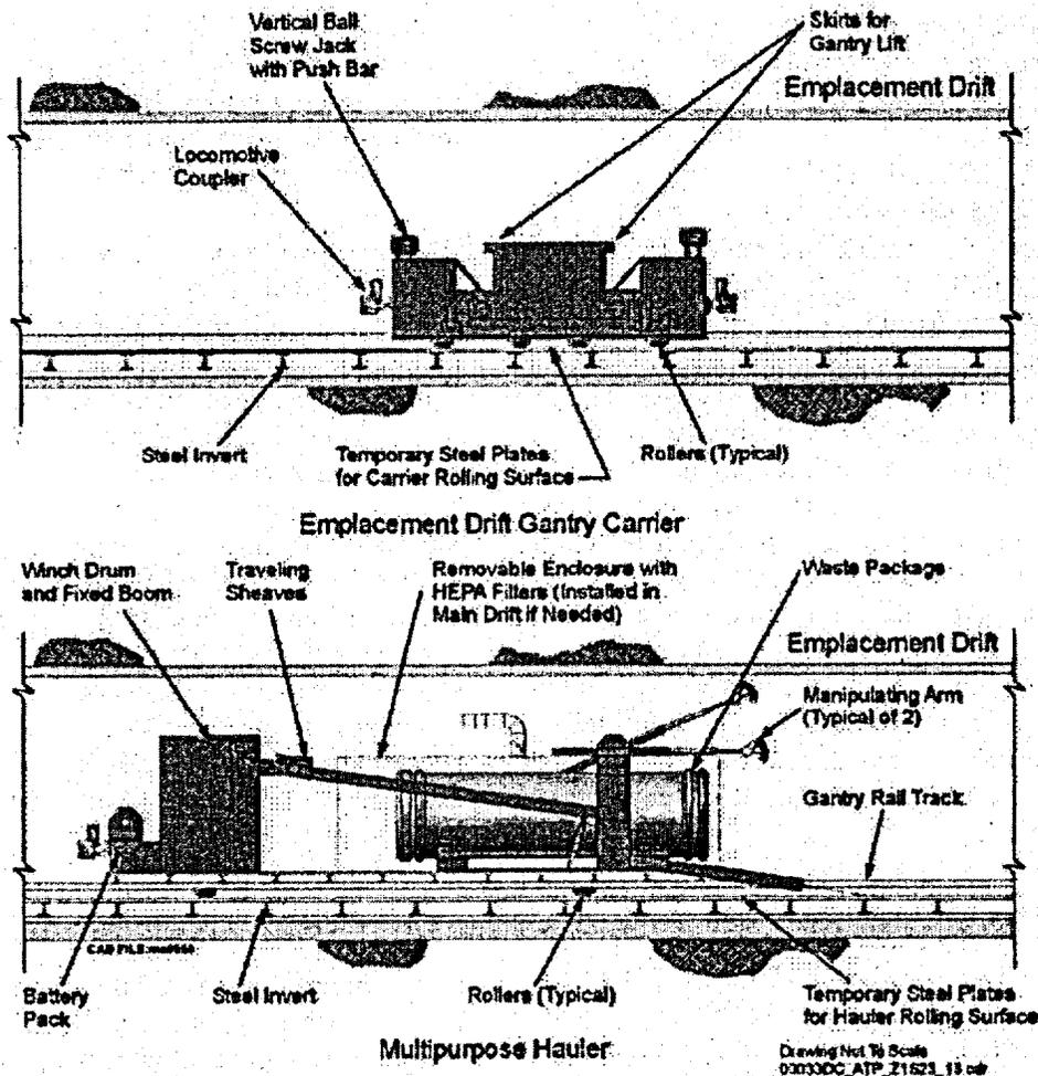
Figure 2-58. Emplacement Drift Gantry Carrier and Multipurpose Hauler
