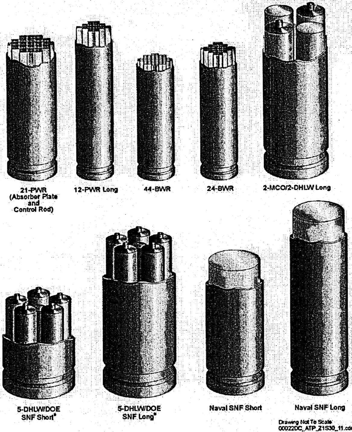
Figure 3-5. Waste Package Designs with Waste Forms
