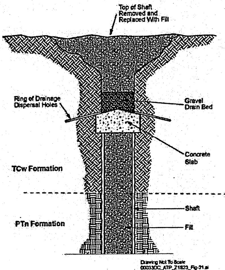
Figure 2-63. Conceptual Arrangement of Shaft Plug
