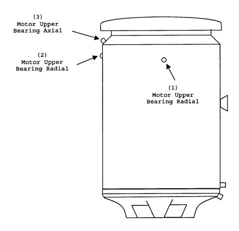
Hold vibrometer probe tip firmly against the survey point marker, perpendicular to the surface. Locations of markers are depicted above.
