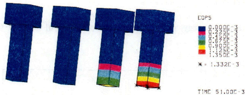
Figure 11. Equivalent plastic strain in closure lid bolts for 96 kph [60 mph] CG-over-corner impact.
