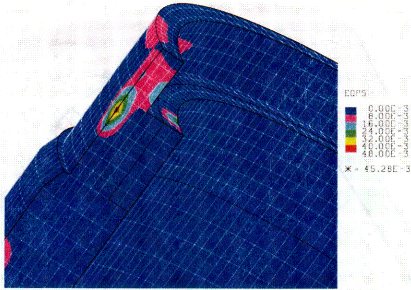
Figure 27. Equivalent Plastic Strain in cask for the CG-over-corner orientation after a 120 kph [75 mph] impact onto a rigid target.
