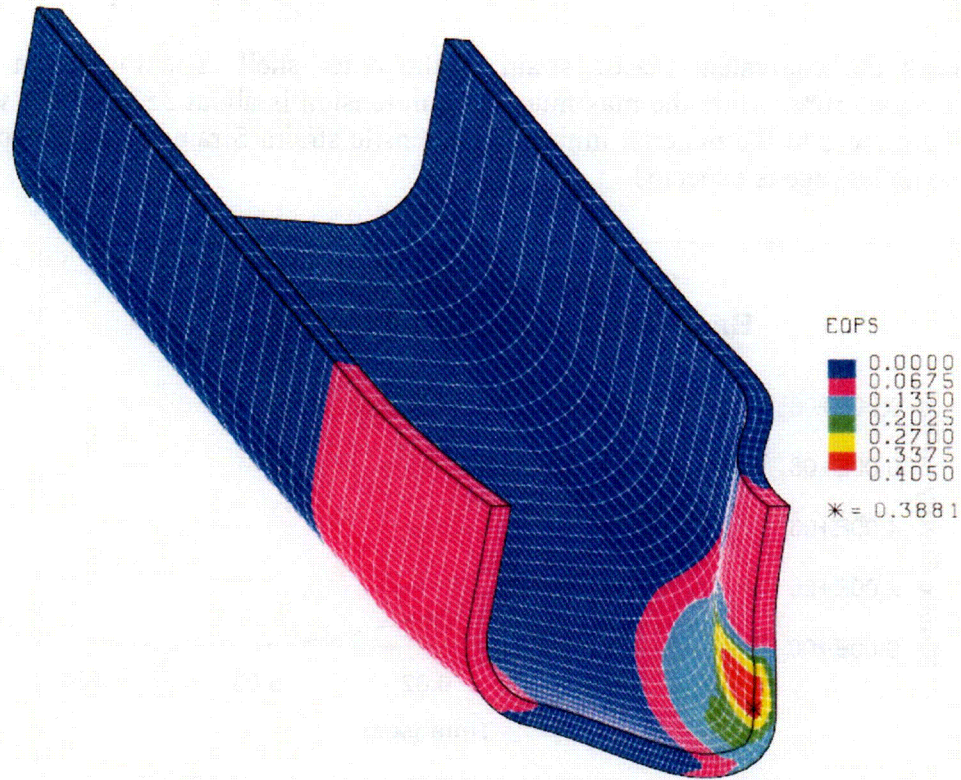
Figure 45. Section view of the GA-4 Cask after a 96 kph [60 mph] back-break impact showing equivalent plastic strain in containment boundary, modeled with fractured DU segments.
