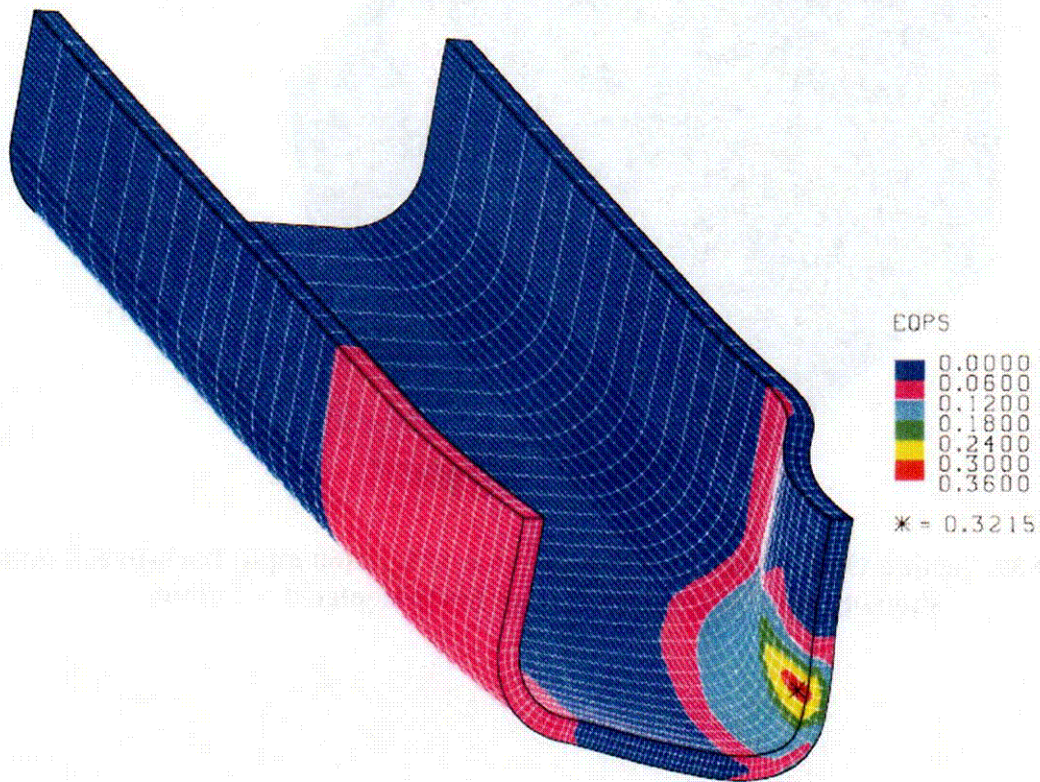
Figure 38. Section view of the GA-4 Cask after a 96 kph [60 mph] back-break impact showing equivalent plastic strain in containment boundary.
