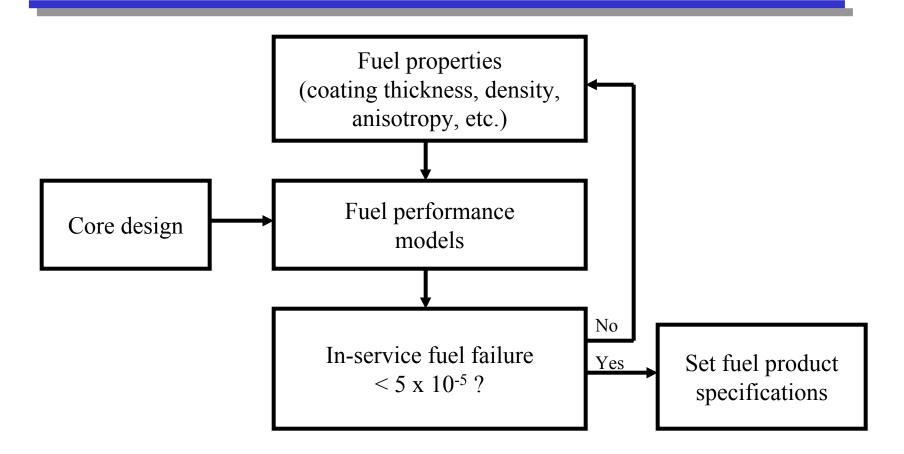
Fuel performance models establish link between inservice fuel failure and measurable fuel properties
