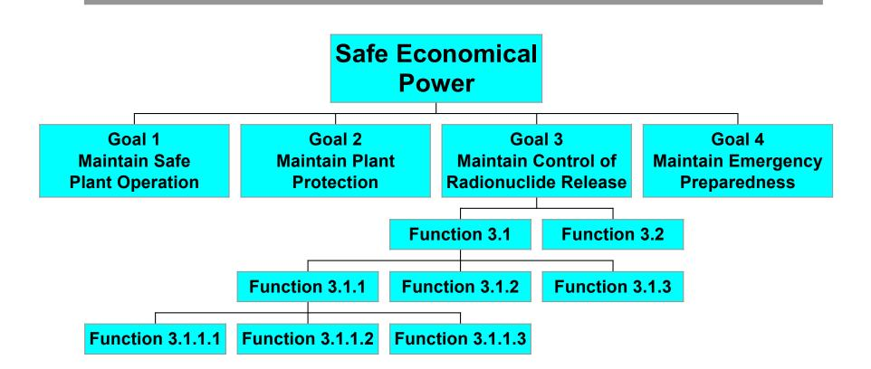
Requirements Are Specified and Design Selections Made for Each Function; These Requirements and Design Selections Cascade Downward until the Design Basis Is Completely Defined
