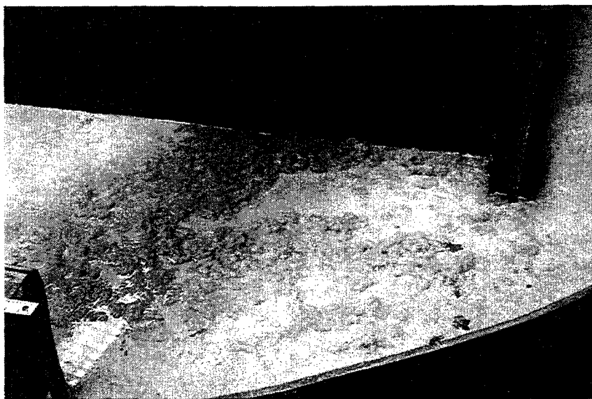
Figure 3-4 Typical Placement of Debris on Floor Before the Tank Is Filled
