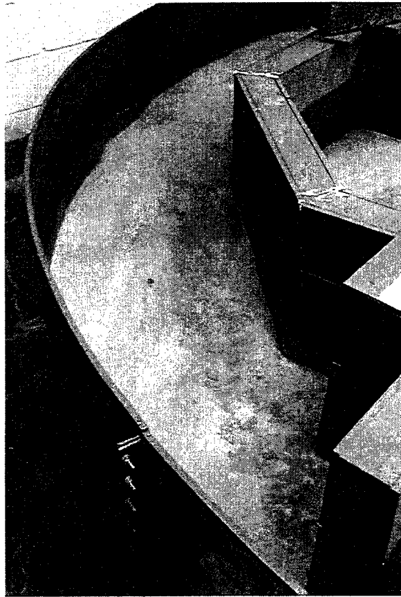
Figure 6-3 Debris Trapped in the Annulus Away from the Inlet
