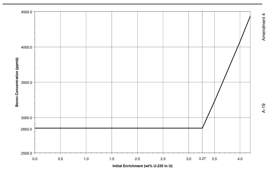
Figure 4 - W 15x15 Assembly Class Minimum Required Soluble Boron
