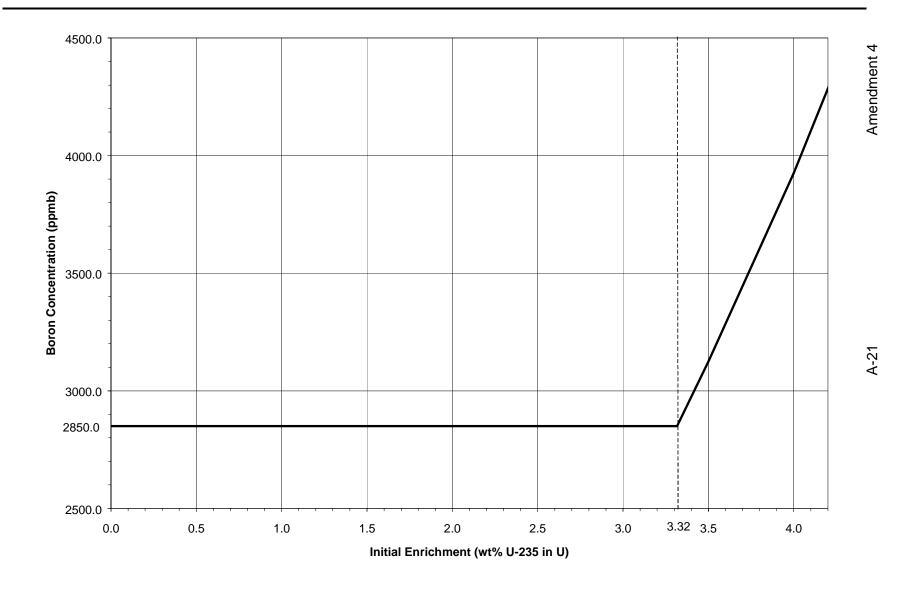
Figure 6 - CE 15x15A Assembly Class Minimum Required Soluble Boron
