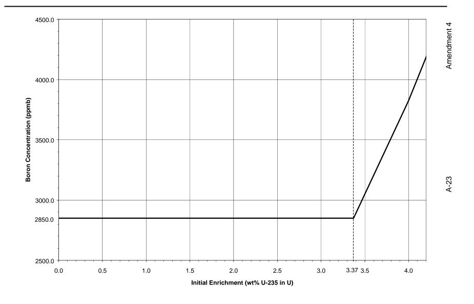
Figure 8 - CE 15x15C Assembly Class Minimum Required Soluble Boron
