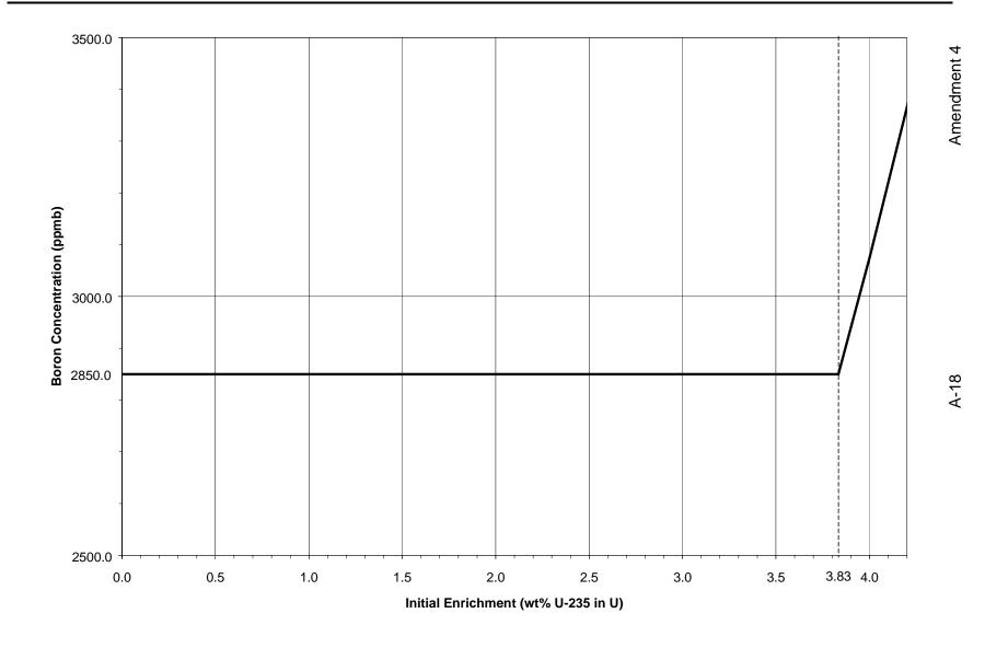
Figure 3 - W 14x14 Assembly Class Minimum Required Soluble Boron
