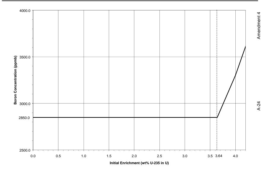
Figure 9 - CE 16x16 Assembly Class Minimum Required Soluble Boron
