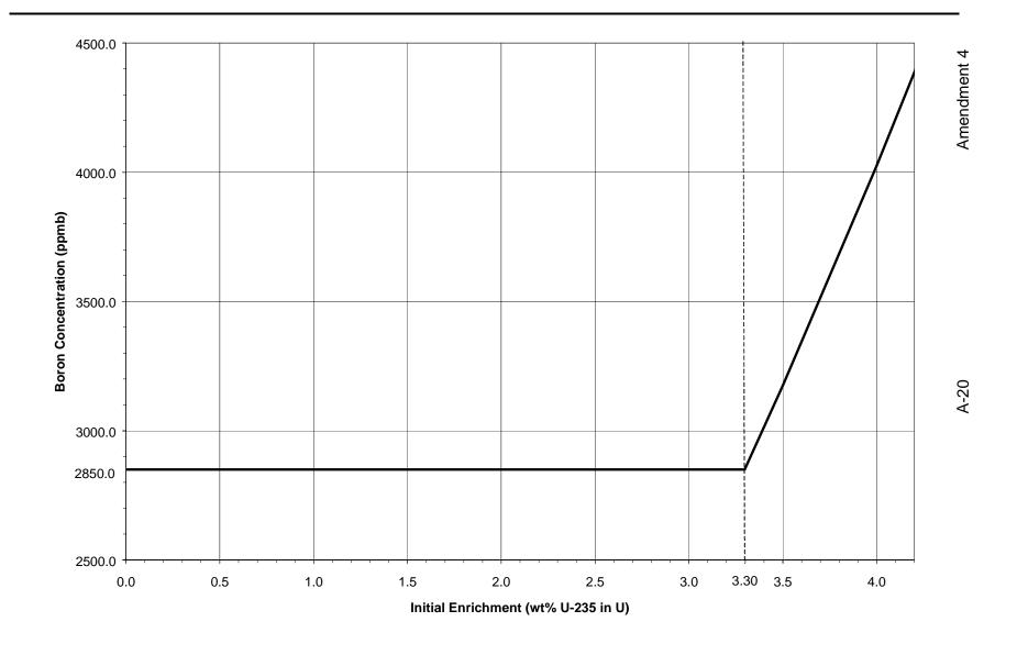
Figure 5 - W 17x17 Assembly Class Minimum Required Soluble Boron
