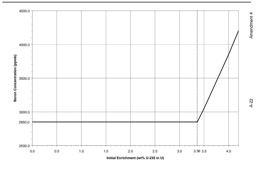
Figure 7 - CE 15x15B Assembly Class Minimum Required Soluble Boron
