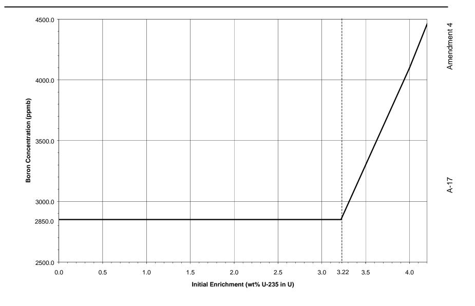
Figure 2 - B&W 15x15 Assembly Class Minimum Required Soluble Boron
