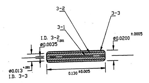
Note: Both ends are crimped
