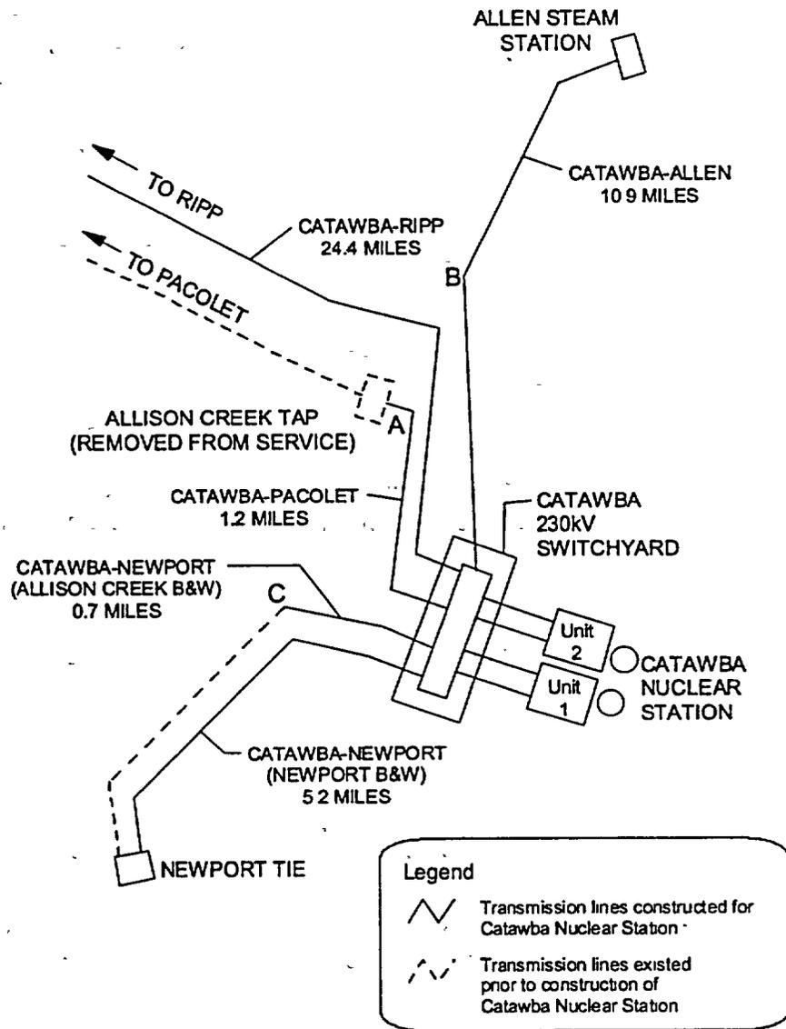
Figure 2-4. Catawba Transmission Lines and Rights-of-Way (Duke 2001a)
