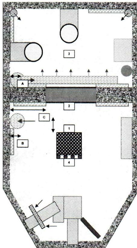
*Figure 1: Reactor Pool Schematic Showing Temperature Probe Locations*
