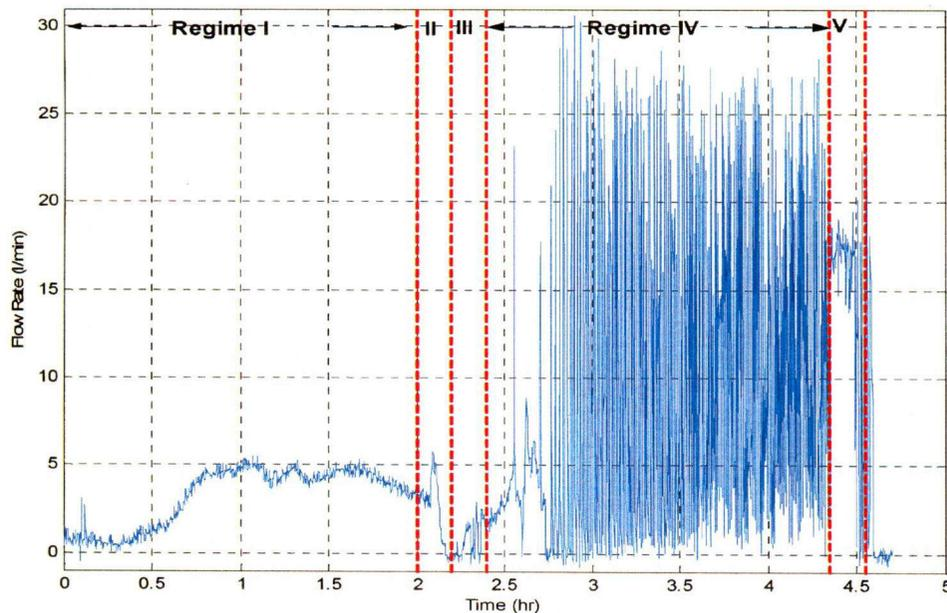
Fig. 4. Variation of flow rate throughout the entire test loop operation. The effect of system depressurization can be seen around 2<sup>nd</sup> hour. Regime I: single phase heating; Regime II: draining a portion of the system inventory; Regime III: system reheat; Regime IV: flow oscillations in two-phase region; Regime V: stable two-phase flow behavior.
