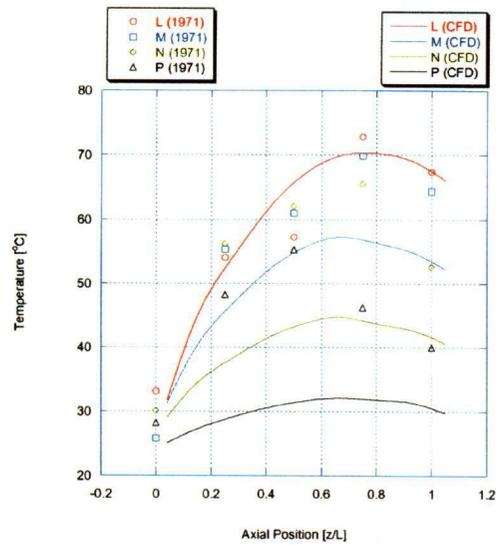
Figure 8 – Temperature profile along the coolant channel
