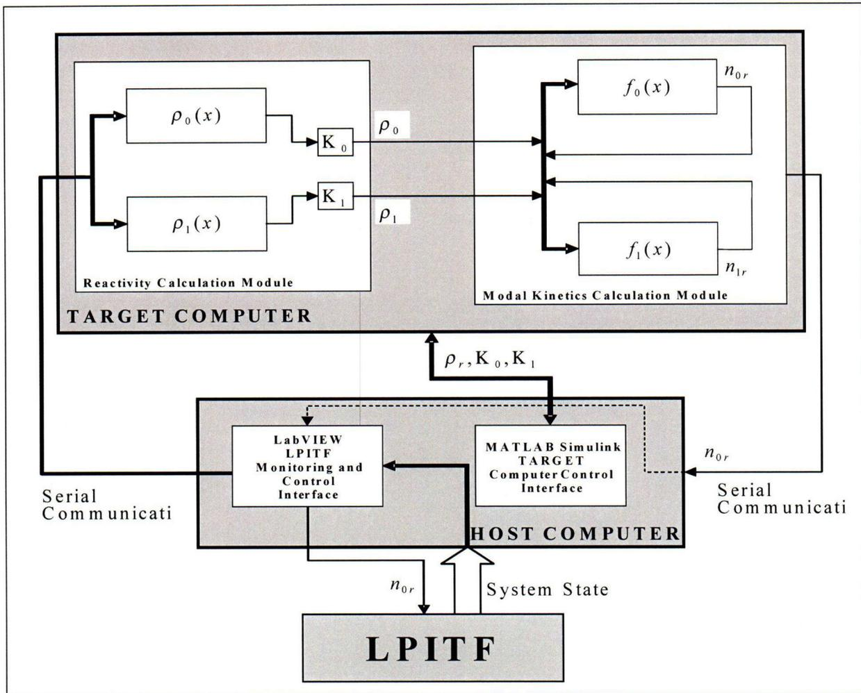
Fig. 1. The general structure of the hybrid loop simulator.
