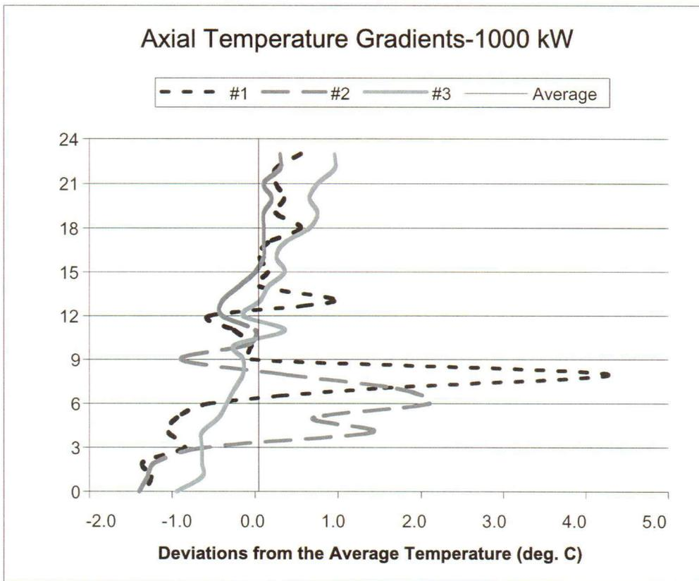
Figure 2: Axial Temperature Profile along the Pool Centerline.
