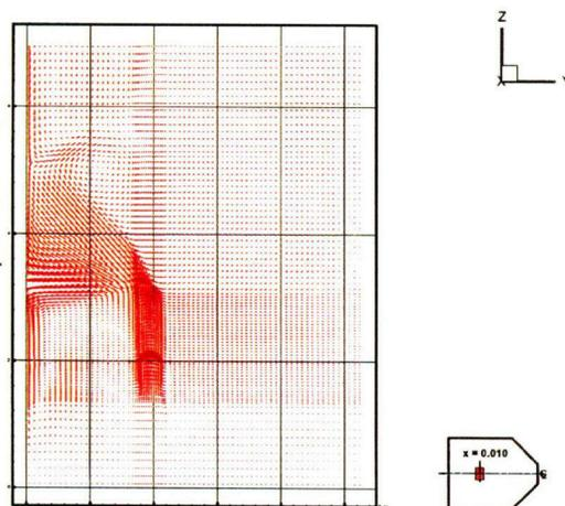
Figure 5 – Velocity distribution on the center plane of the PSBR pool
