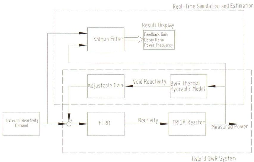
Fig. 9: Setup for Testing the Core-Wide Stability Monitor
