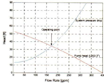
Figure 6 – Performance curve of the N-16 pump and system pressure drop
