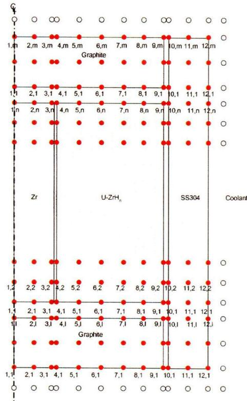
Figure 3 – Noding scheme of a stand-alone fuel rod model
