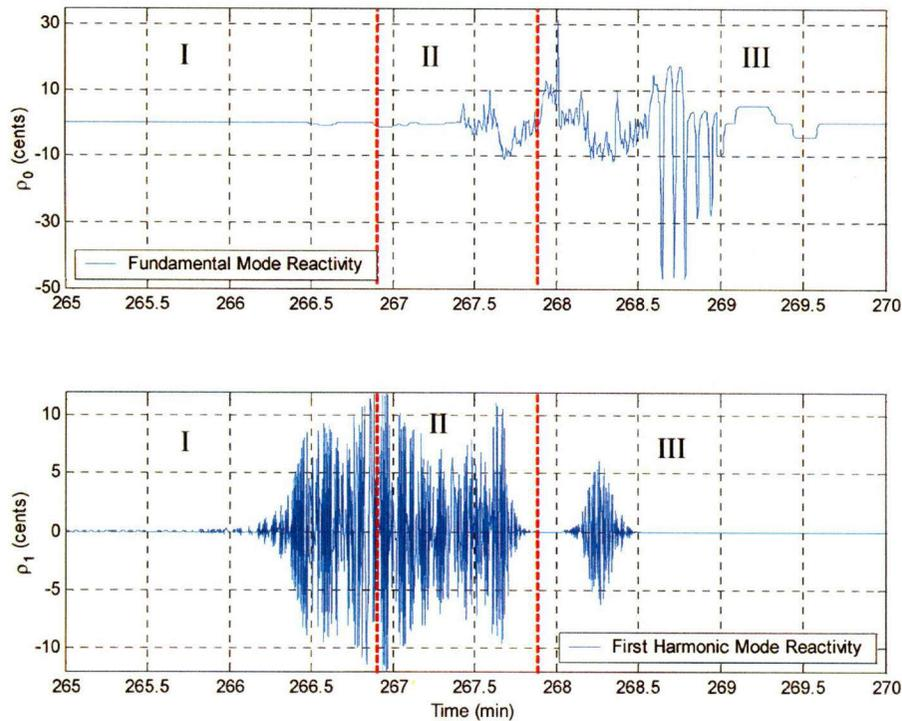
Fig. 8. Response of the reactor due to Doppler and void reactivity feedbacks in terms of fundamental and first harmonic reactivities.
