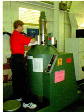
Figure 1. Candace Davison inserts a sample into the GammaCell 220 Dry Irradiator
