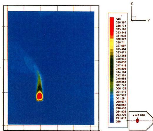
Figure 4 – Temperature distribution on the center plane of the PSBR pool (temperature in Kelvin)
