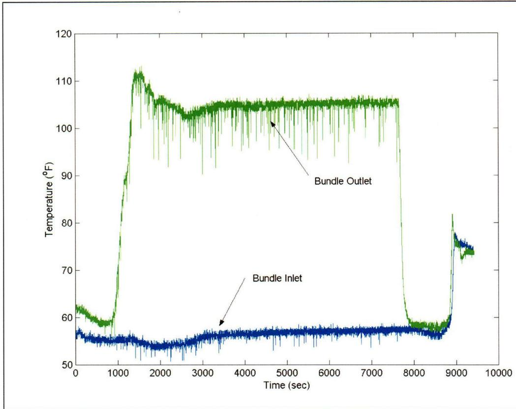
*Figure 7 – History of the core mean temperatures during a single-phase flow.*
