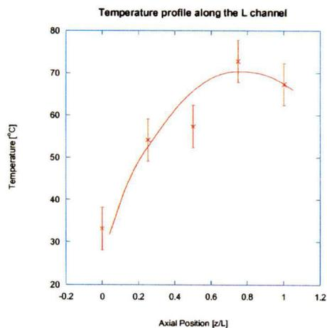
Figure 7 – Comparison of temperature profile near the PSBR core between the measured data and the FLOW-3D result
