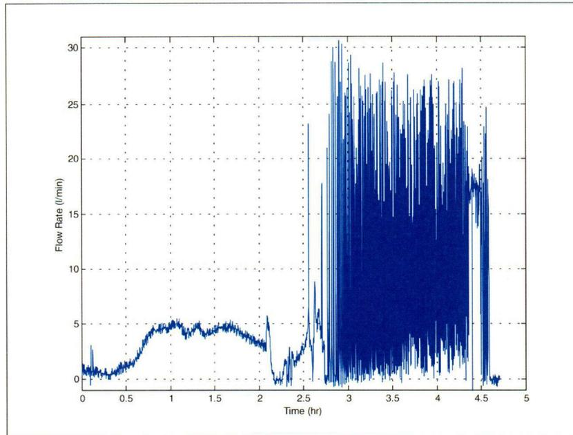
*Figure 12 – Flow rate during the two-phase natural circulation experiment.*
