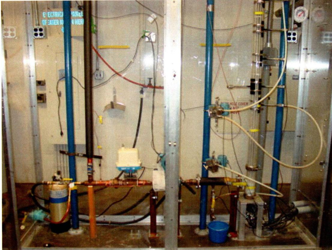
**Figure 3** – Front view of the test loop core section. The core is located on the basement of the Cobalt-60 irradiation facility.
