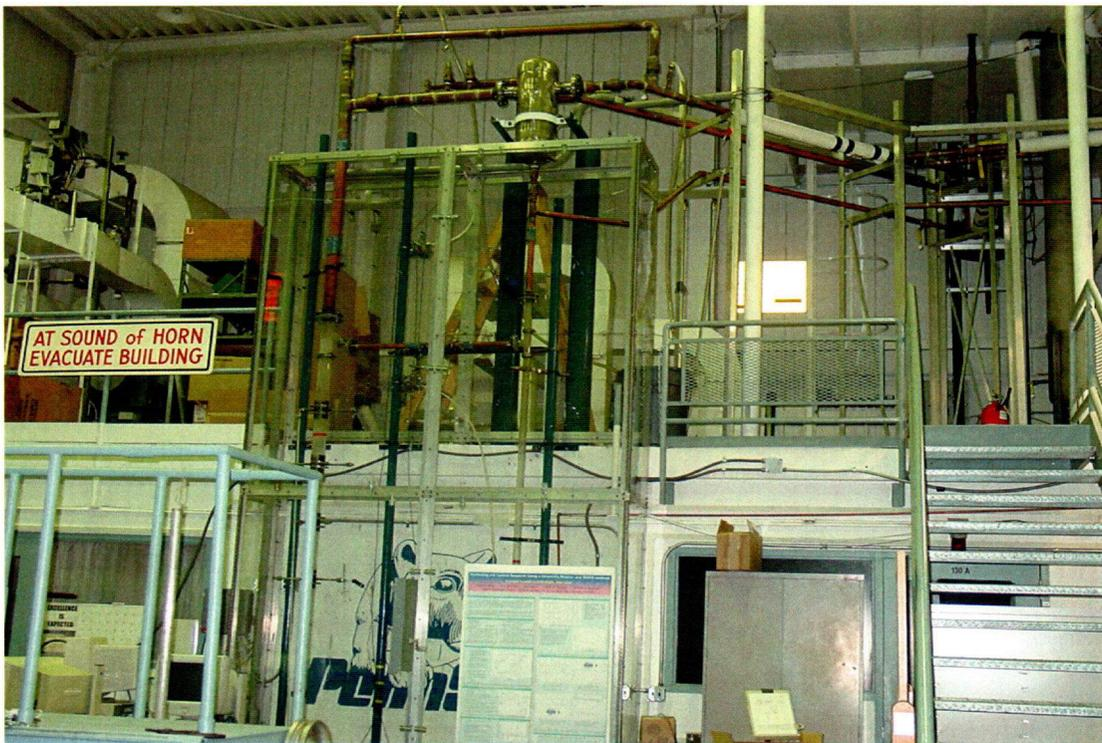
*Figure 13 – The riser, chimney sections of the core; crossover leg, and steam separator.*
