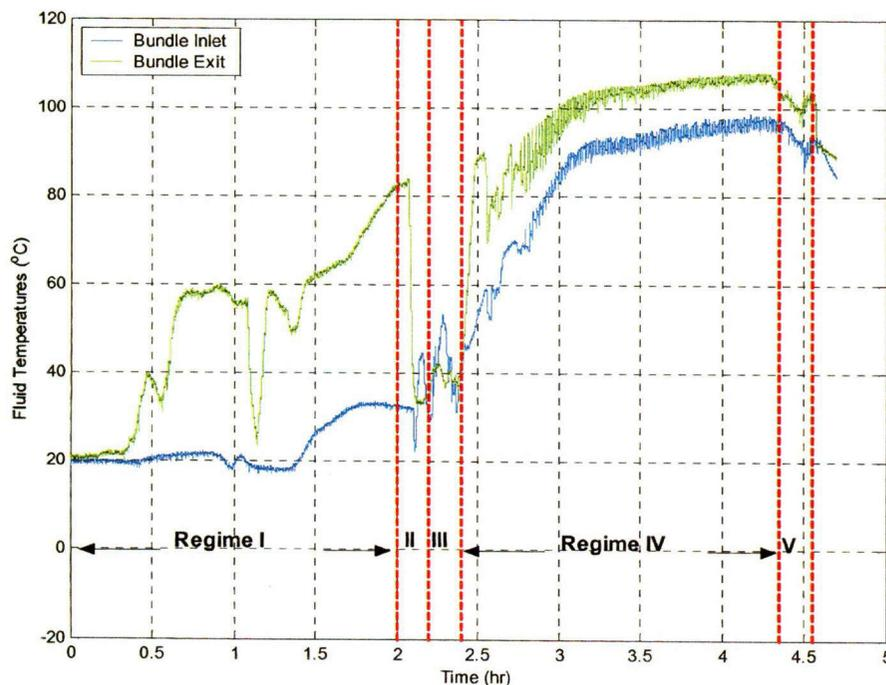
Fig. 5. The variation of average fluid temperatures at bundle inlet and bundle exit.
