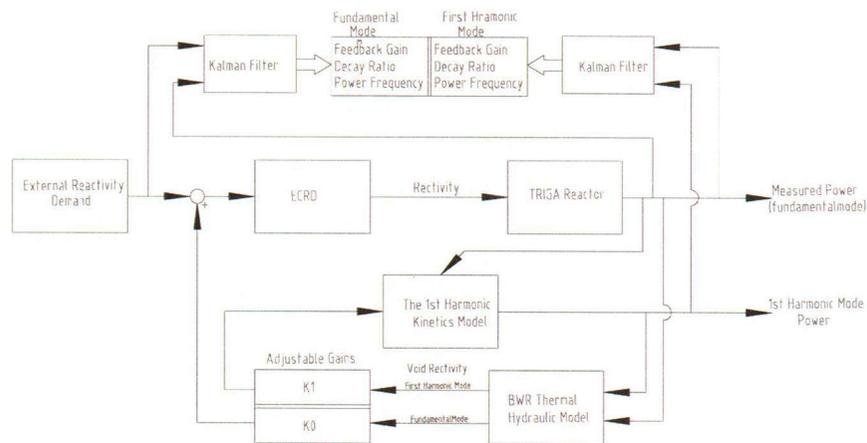
Fig. 11: Setup for Testing In-Phase and Out-of-Phase Stability Monitors
