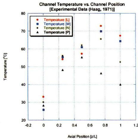
Figure 1 – Measured temperature profile along the coolant channels [Reproduced from Haag (1971)]
