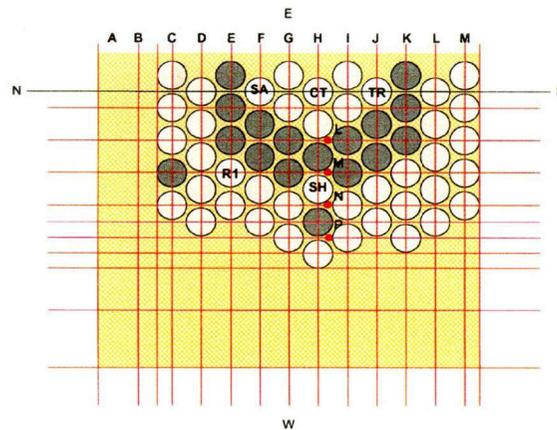
Figure 9 – Top view of the current fuel loading (bright circles are 8.5 w/o fuel rods and dark circles are 12.0 w/o fuel rods)
