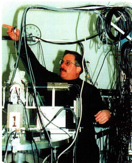
Prof. Catchen inserts a sample into a high-temperature sample furnace, which is mounted in the center of the four-detector array of the perturbed-angular-correlation spectrometer
