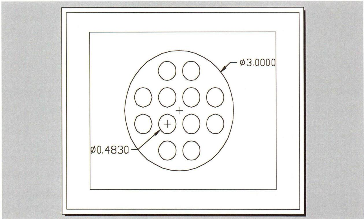
Figure 2 – Core rod layout.
