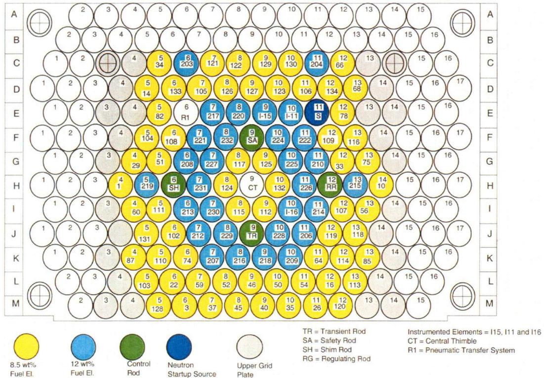
Figure 3-2 Layout of the PSBR Grid Plate (3/6/01)
