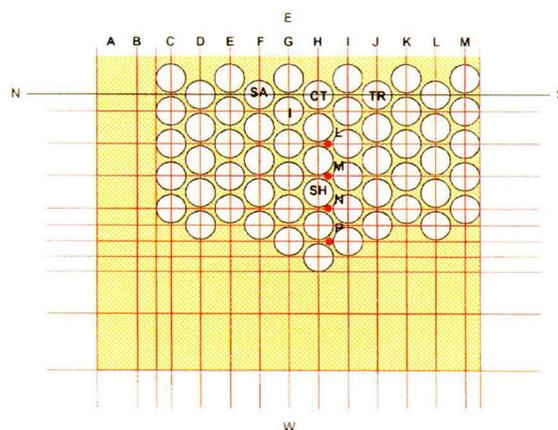
Figure 2 – Top view of the early 1970s fuel loading (gray circles are 8.5 w/o fuel rods)
