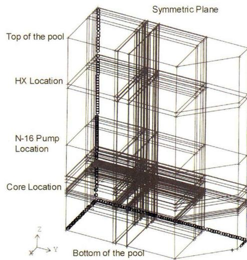
Figure 2 – Volume blocks for grid generation in GAMBIT
