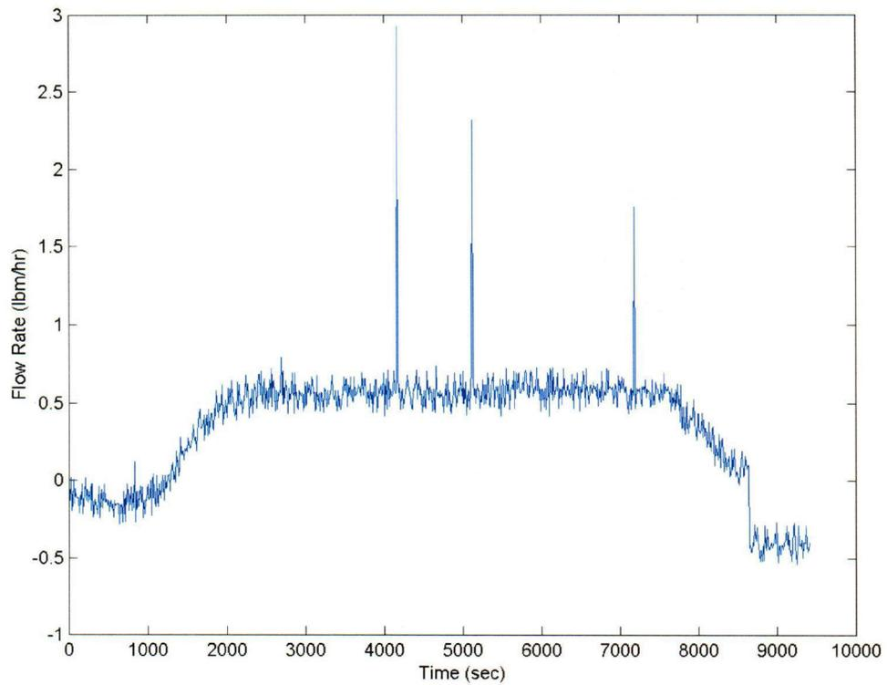
Figure 9 – Single-phase natural circulation flow rate.
