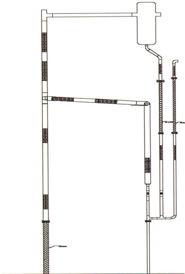
Figure 1 – Detail of the modifications to the downcomer line and crossover leg.
