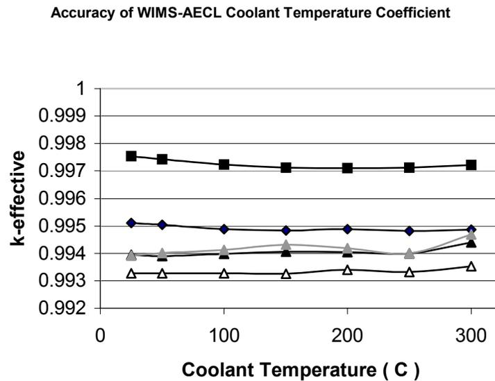
**Figure 1. Accuracy of WIMS-IST Coolant-Temperature Reactivity Coefficient**
