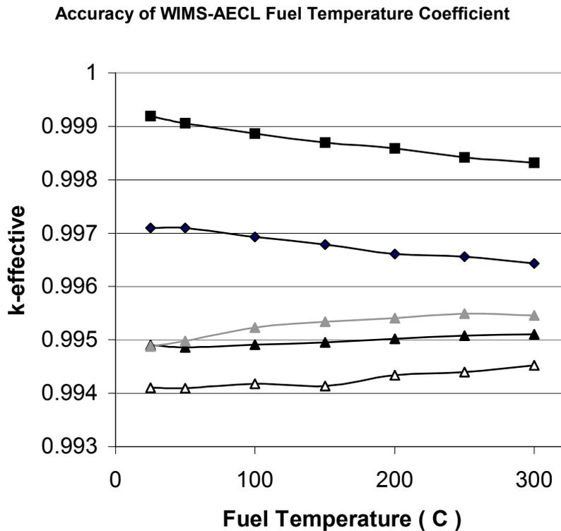
**Figure 3. Accuracy of WIMS-IST Fuel Temperature Coefficient**
