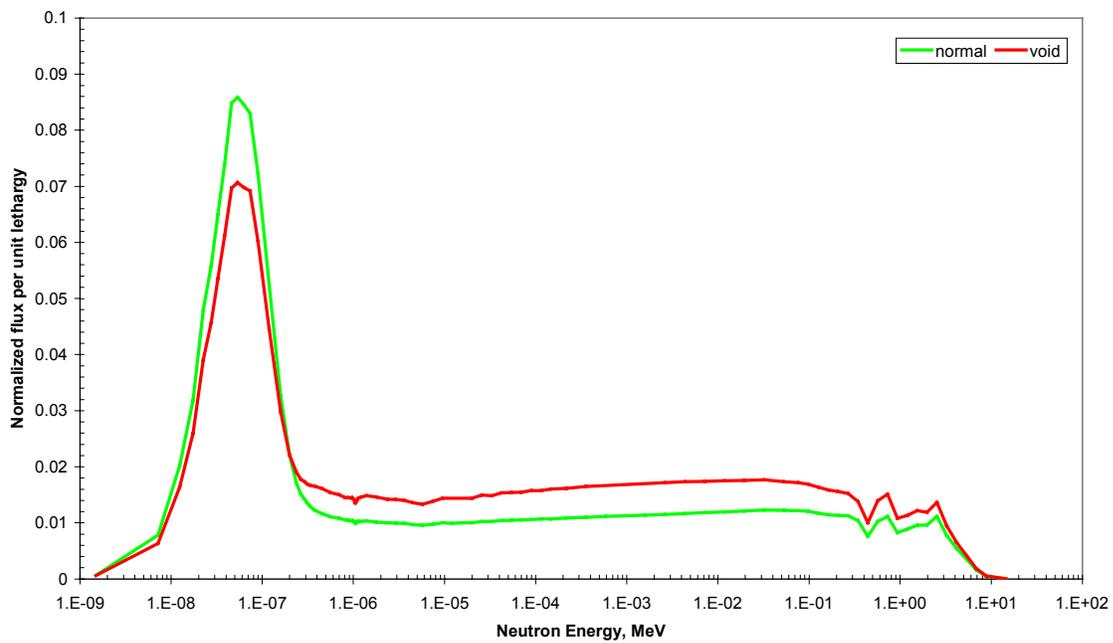
**Figure 5** Neutron Flux Averaged over D<sub>2</sub>O Moderator Region (MCNP Model)
