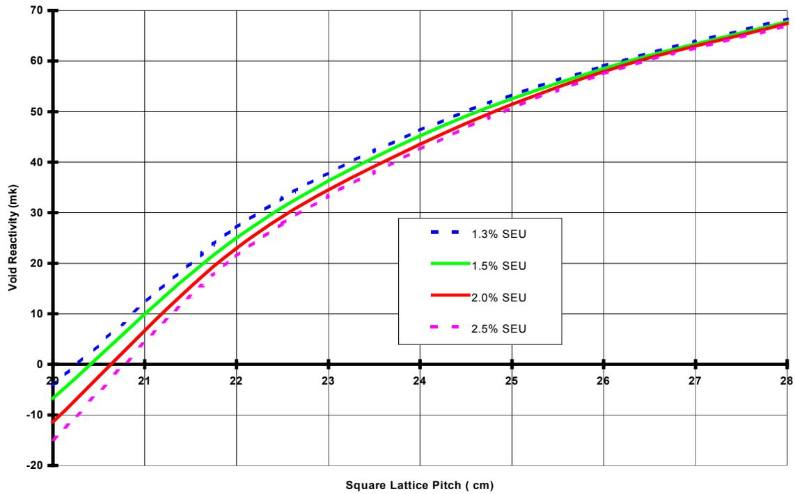
**Figure 1: Coolant (H<sub>2</sub>O) Void Reactivity Vs Fuel Enrichment and Lattice Pitch with D<sub>2</sub>O Moderator and Current Pressure Tube and Calandria Tube Dimensions**
