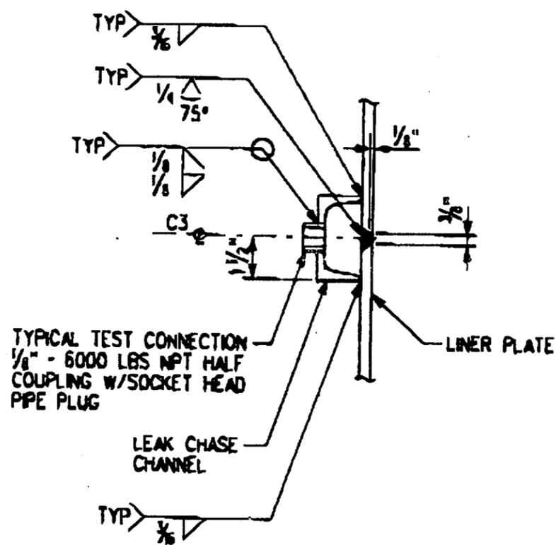
DETAIL FOR LINER PLATE WELDING
