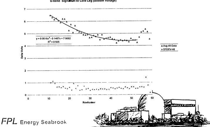
U-bend Signal Set to Cold Leg (Bobbin Voltage)
