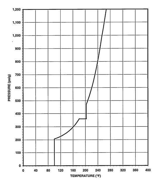
NMP-1 Pressure and Temperature Limits Core Critical Conditions (COOLDOWN) ≤ 28 EFPY
