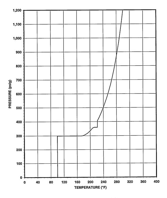
Figure 3-8. Revised Heatup Core Critical P-T Curve for 28 EFPY
