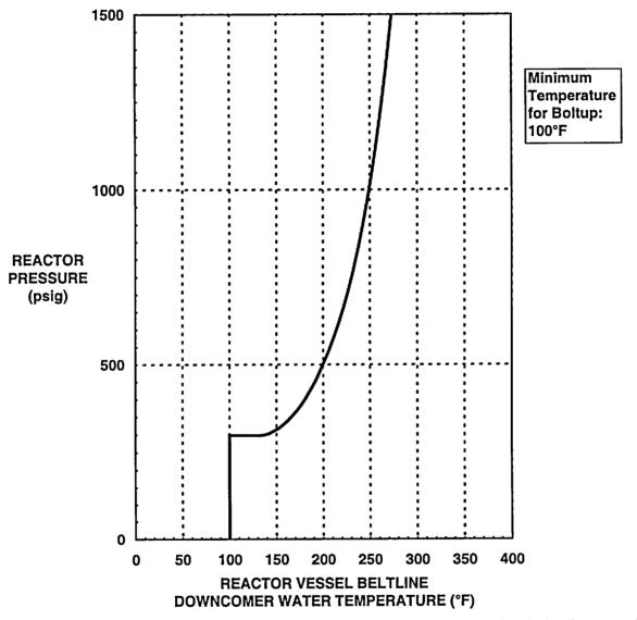
(reactor vessel beltline downcomer water temperature is measured at recirculation loop suction) (instrument uncertainties have been included in this figure)
