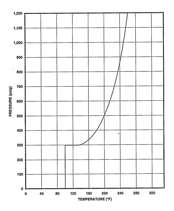
Figure 3-6. Revised Heatup Core Not Critical P-T Curve for 28 EFPY
