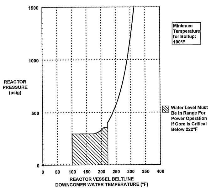
(reactor vessel beltline downcomer water temperature is measured at recirculation loop suction) (instrument uncertainties have been included in this figure)
