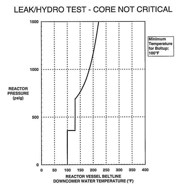
(reactor vessel beltline downcomer water temperature is measured at recirculation loop suction) (instrument uncertainties have been included in this figure)
