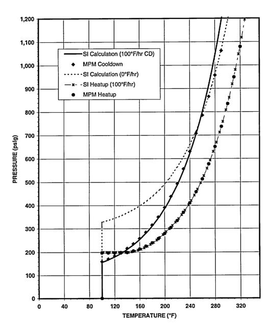
Figure 3-2. Benchmark Core Not Critical Curve
