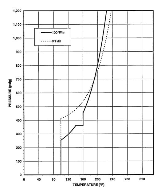
NMP-1 Pressure and Temperature Limits Core Not Critical Conditions (COOLDOWN) ≤ 28 EFPY
