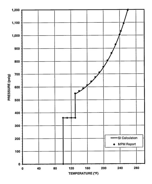
Figure 3-1. Benchmark Pressure Test P-T Curve
