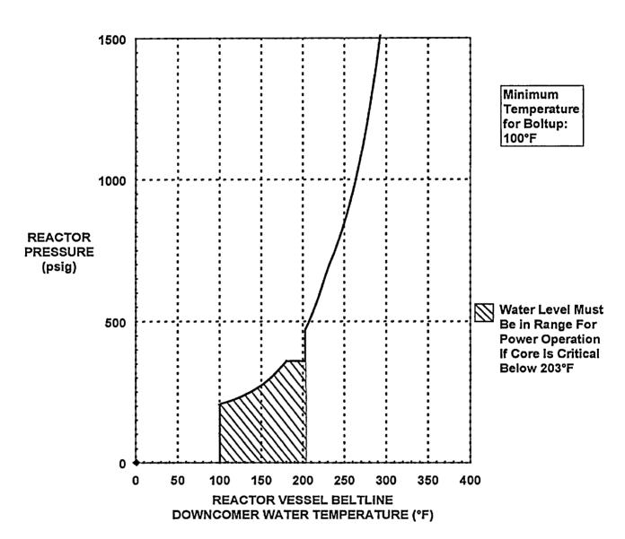
(reactor vessel beltline downcomer water temperature is measured at recirculation loop suction) (instrument uncertainties have been included in this figure)
