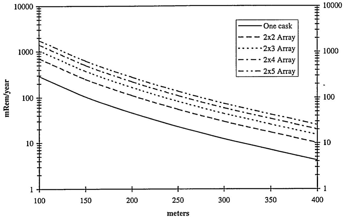
FIGURE 5.1.3; ANNUAL DOSE VERSUS DISTANCE FOR VARIOUS CONFIGURATIONS OF THE MPC-24 FOR 47,500 MWD/MTU AND 3-YEAR COOLING (8760 HOUR OCCUPANCY ASSUMED)
