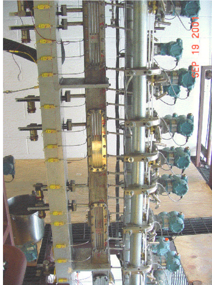
Flow Housing Instrumentation
