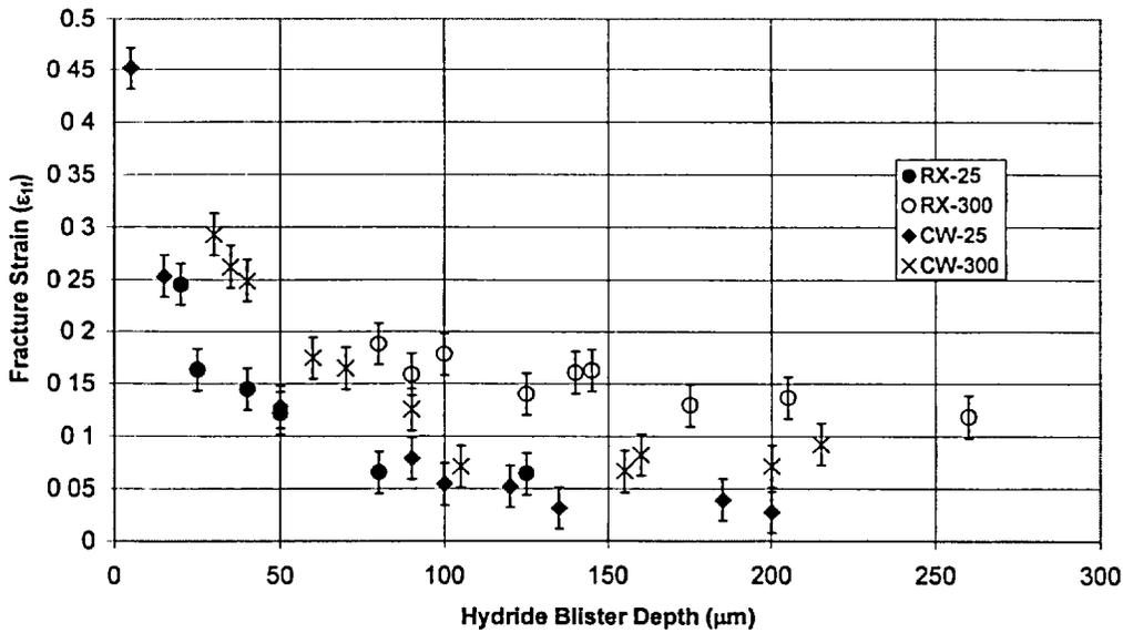
Figure 2. The local fracture strain as a function of hydride blister thickness for both cold worked and stress relieved (CWSR) and recrystallized (RX) Zircaloy-4 sheet tested at either 25°C or 300°C. All data are for 3 mm blisters.
