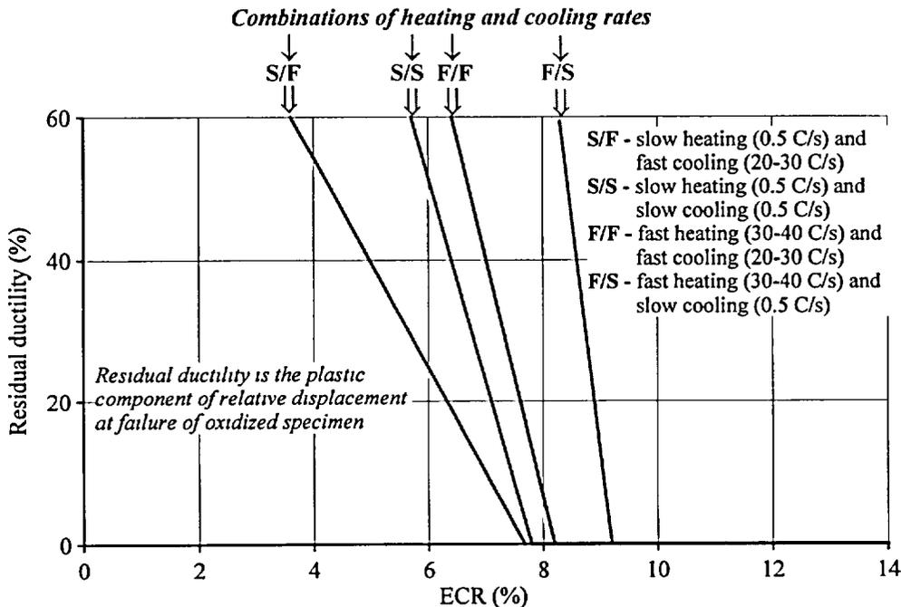
Fig. 1. Residual ductility of unirradiated E110 cladding oxidized at 1100 C as a function of ECR for various heating and cooling rates.
