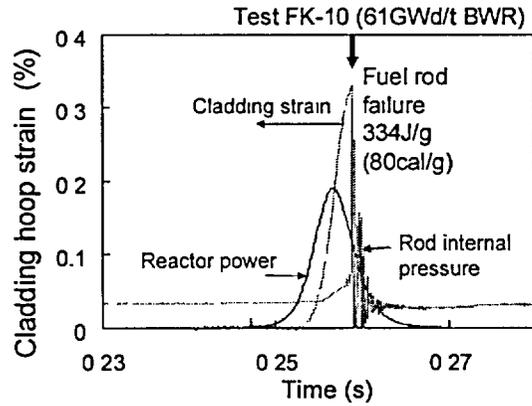
Fig. 1 Cladding deformation history measured in a RIA test with a high burnup BWR fuel rod. The rod failed at a fuel enthalpy of 80 cal/g with cladding hoop strain below 0.4%.
