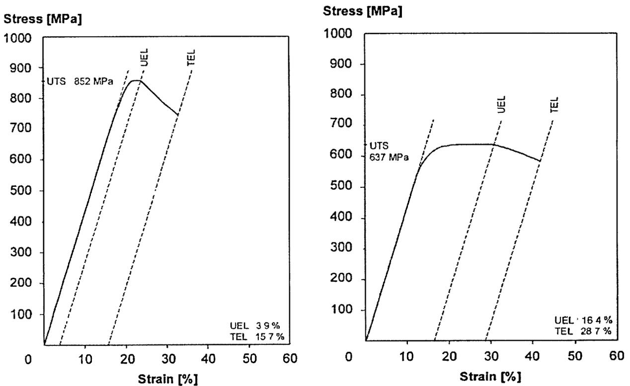
Figure 1. Stress strain curves generated from room temperature tensile testing of clad from a fuel rod exposed to in-pile dry-out from (a) unaffected zone and (b) dry-out zone (PCT<850°C).
