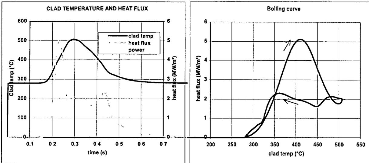
Calculations with the TH2D computer code (two-phase and 2D code designed for computing thermal-hydraulics during a RIA and developed within an IRSN/Kurchatov Institute cooperation) allows to estimate the topology of the flow during the transient. The next figure shows that most of the coolant is not affected by the clad heating: the thermal gradient only concerns a small fluid layer in the vicinity of the wall. The vapor film reaches approximately 5% of the channel.
