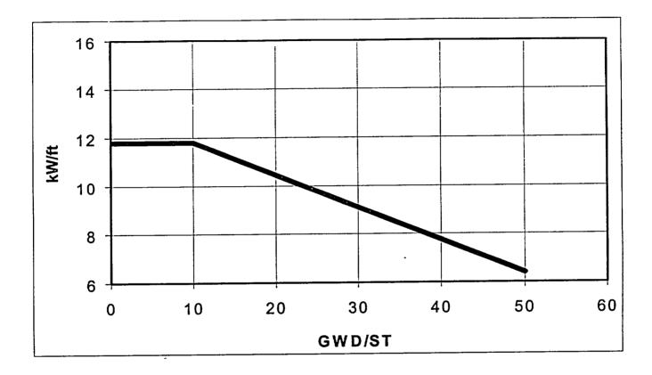
Technical Specification LCO 3.2.3, Linear Heat Generation Rate (LHGR)
