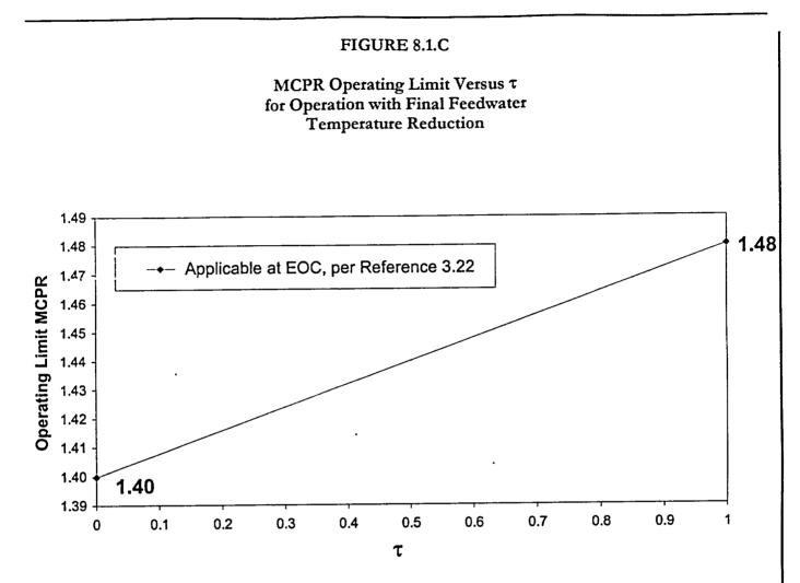
Technical Specification LCO 3.2.2, Minimum Critical Power Ratio (MCPR)
