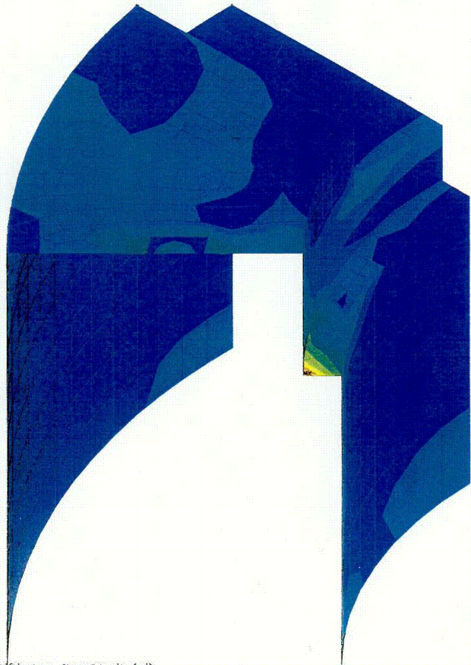
Figure 3.D.4. Top End Lift at the Lifting Lugs - Stress Intensity (psi)
