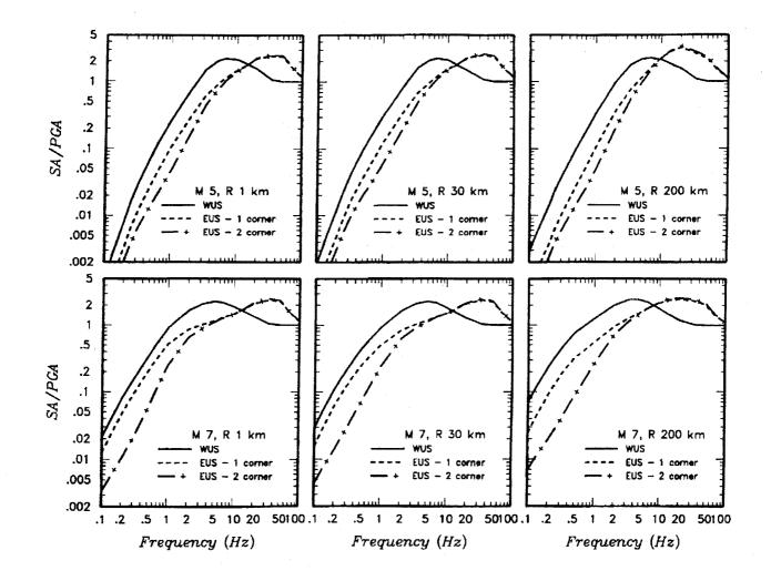
Figure 3. Recommended spectral shapes by scaling WUS records to CEUS hard rock conditions.
