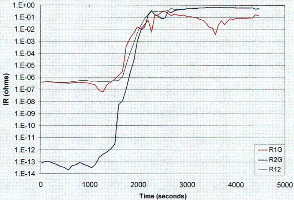
Figure 5-49. Leakage currents resulting from IR changes between Conductors 1 and 2 during Test 12.
