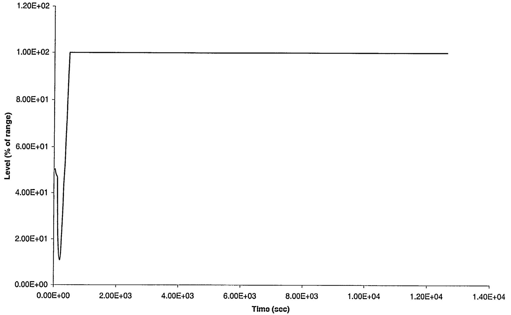
Figure A.7-7: PORV Falsely Lifts and Sticks Open - PORV Flow
