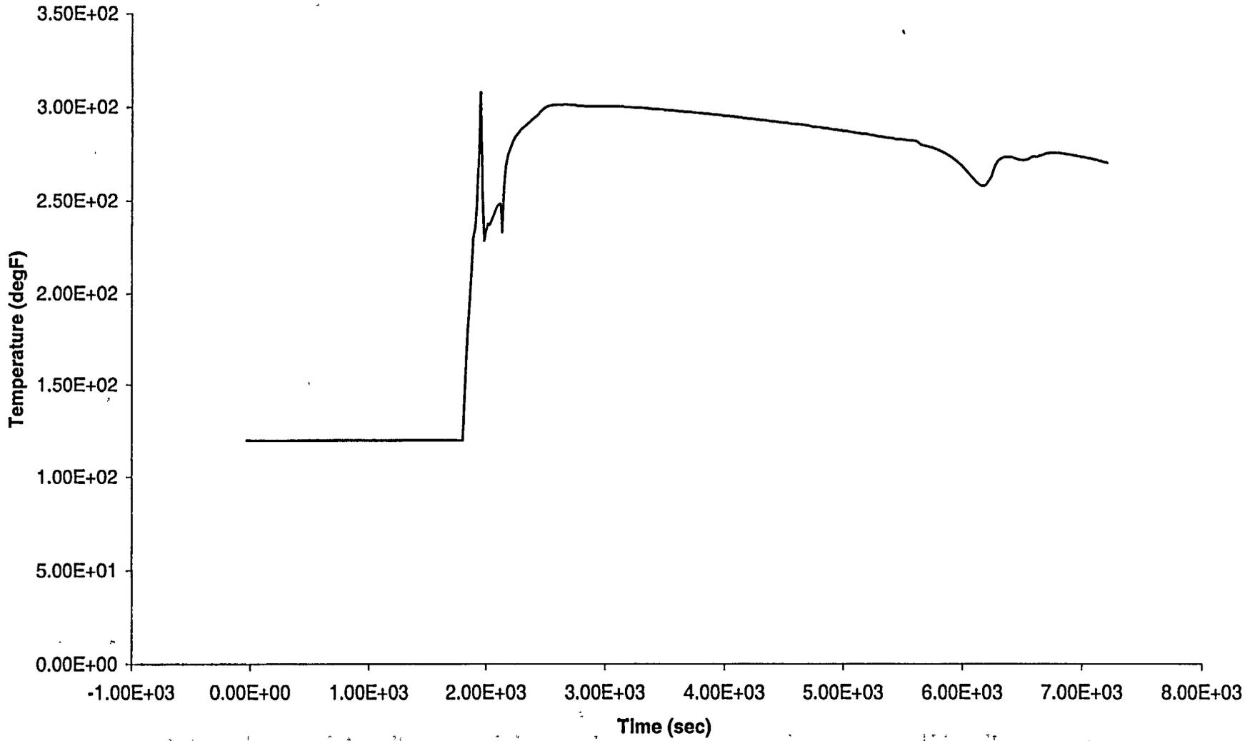
Figure A.6c-1: LOSP with Subsequent AFW Failure, No Operator Action for 2 hrs 30 min - Core Power
