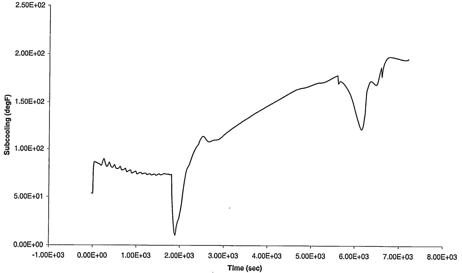
Figure A.6b-13: LOSP with Subsequent AFW Failure, Aggressive Cooling at 30 min - RCS
