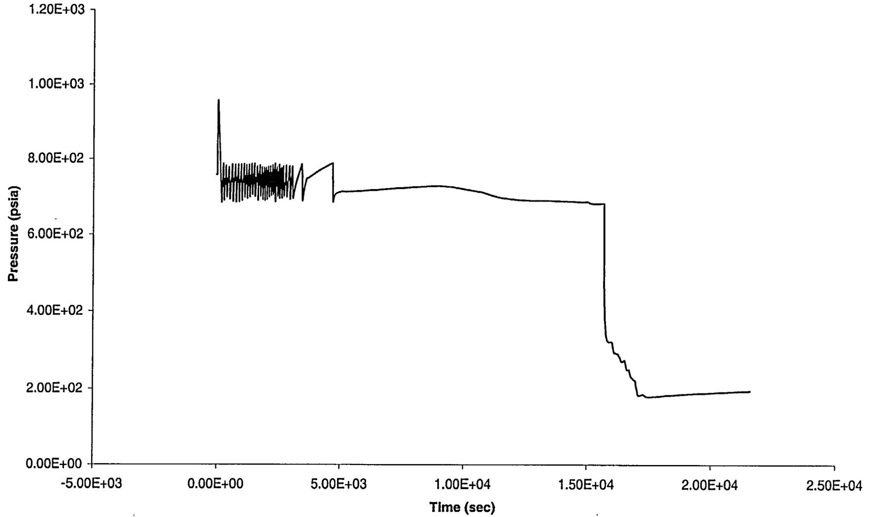
Figure A.6c-10: LOSP with Subsequent AFW Failure, No Operator Action for 2 hrs 30 min - SG
