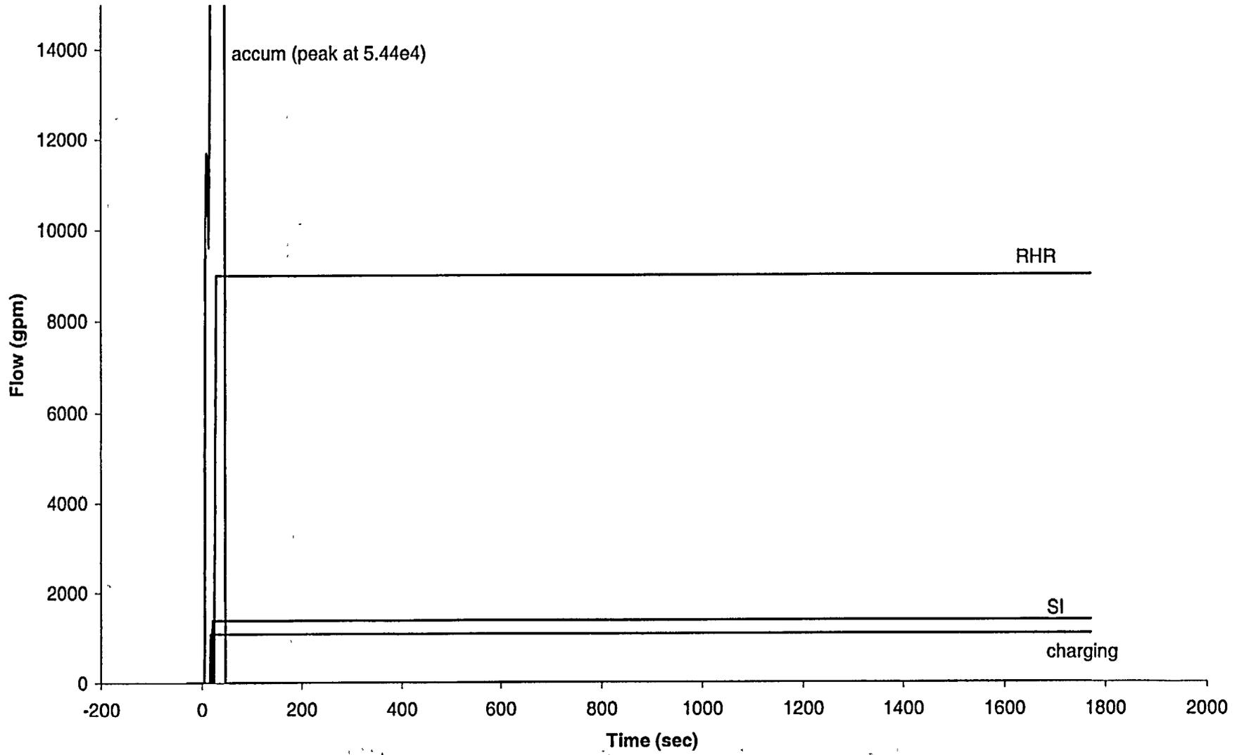
Figure A.1-6: Cold Leg DEGB - Flow Rate at the Break
