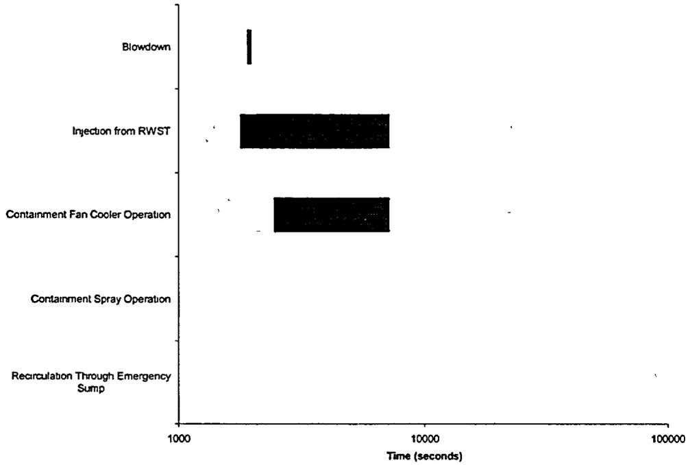
Event Timeline LOSP with LOFW, Fast Cooldown from 30 min - Ice-Condenser
