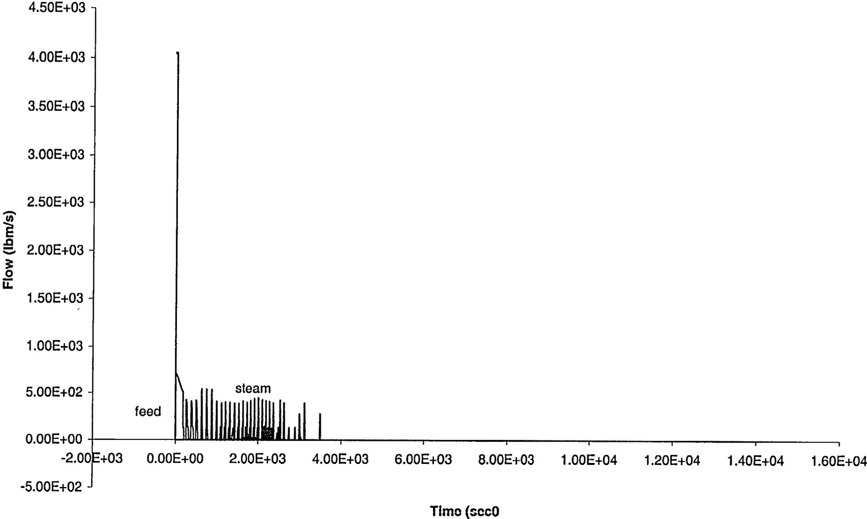
Figure A.6a-4: LOSP with Subsequent AFW Failure, 1 PORV Held Open when it First Lifts - Charging and SI Flows
