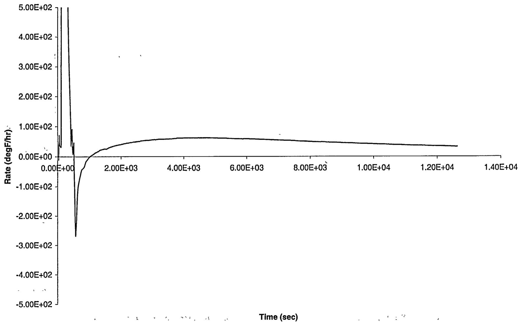
Figure A.7-14: PORV Falsely Lifts and Sticks Open - Cumulative Charging + SI Flow
