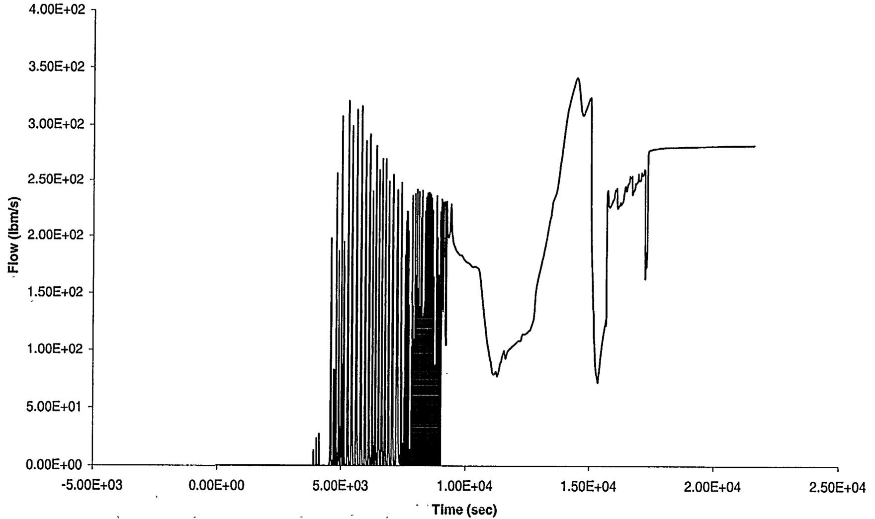
Figure A.6c-8: LOSP with Subsequent AFW Failure, No Operator Action for 2 hrs 30 min - SG
