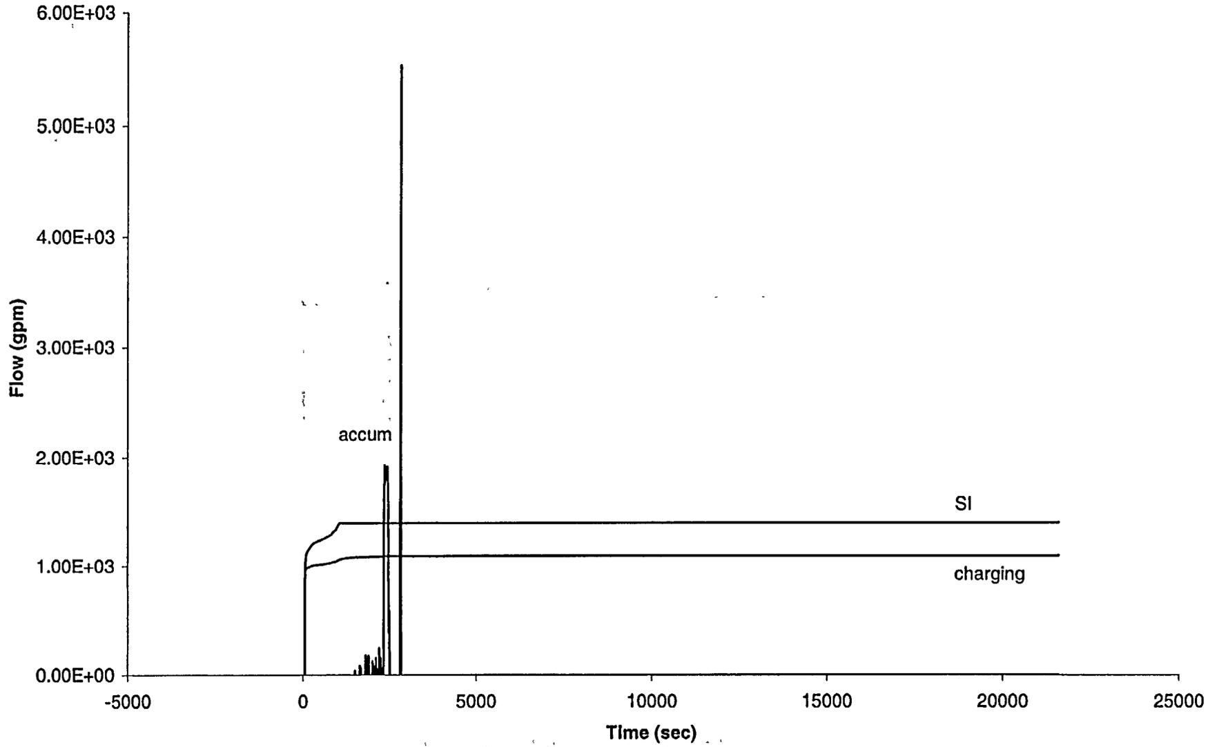
Figure A.3-6: Small LOCA - Break Flow
