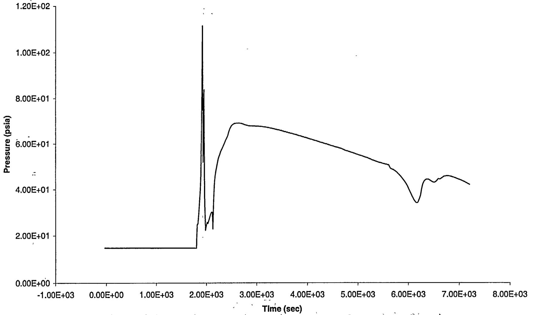
Figure A.6b-16: LOSP with Subsequent AFW Failure, Aggressive Cooling at 30 min - PRT
