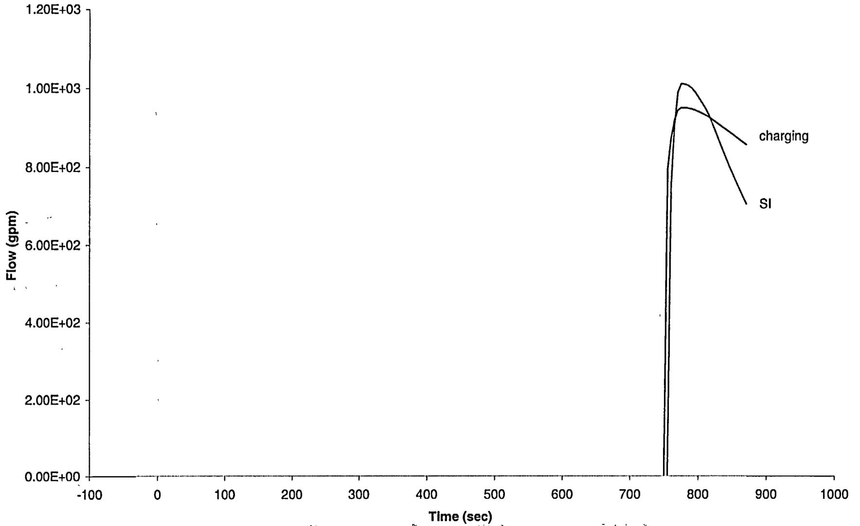
Figure A.4-6: Small-Small LOCA - Volumetric Flow at the Break
