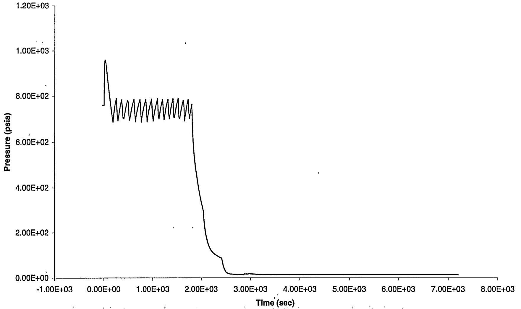
Figure A.6b-10: LOSP with Subsequent AFW Failure, Aggressive Cooling at 30 min - SG 1
