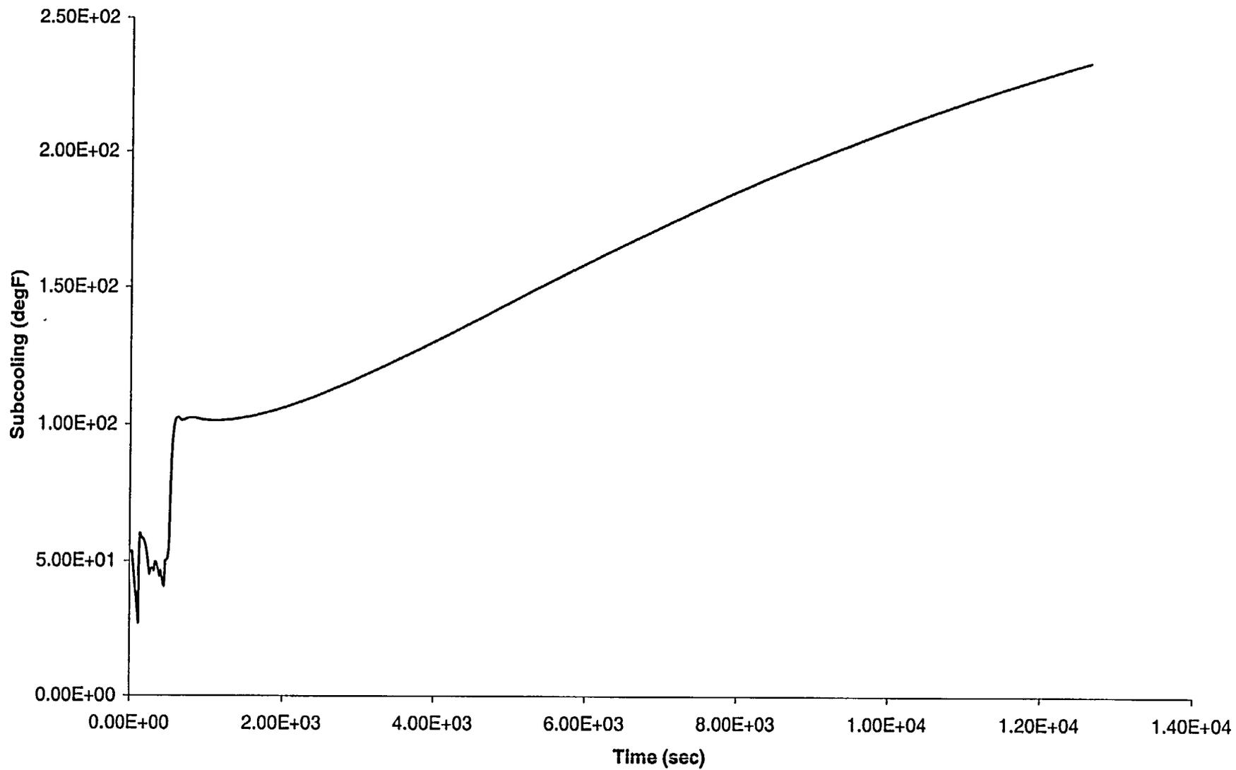
Figure A.7-13: PORV Falsely Lifts and Sticks Open - RCS Cooling Rate
