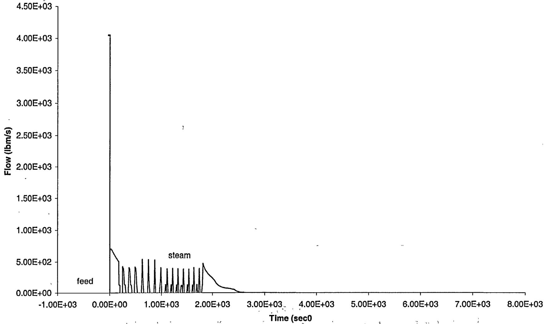
Figure A.6b-4: LOSP with Subsequent AFW Failure, Aggressive Cooling at 30 min - Charging
