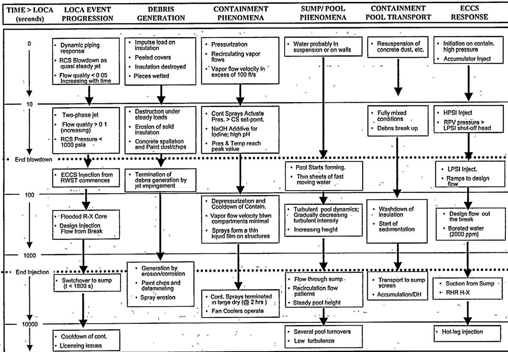
Figure 12 PWR LLOCA Accident Progression In a Large Dry Containment
