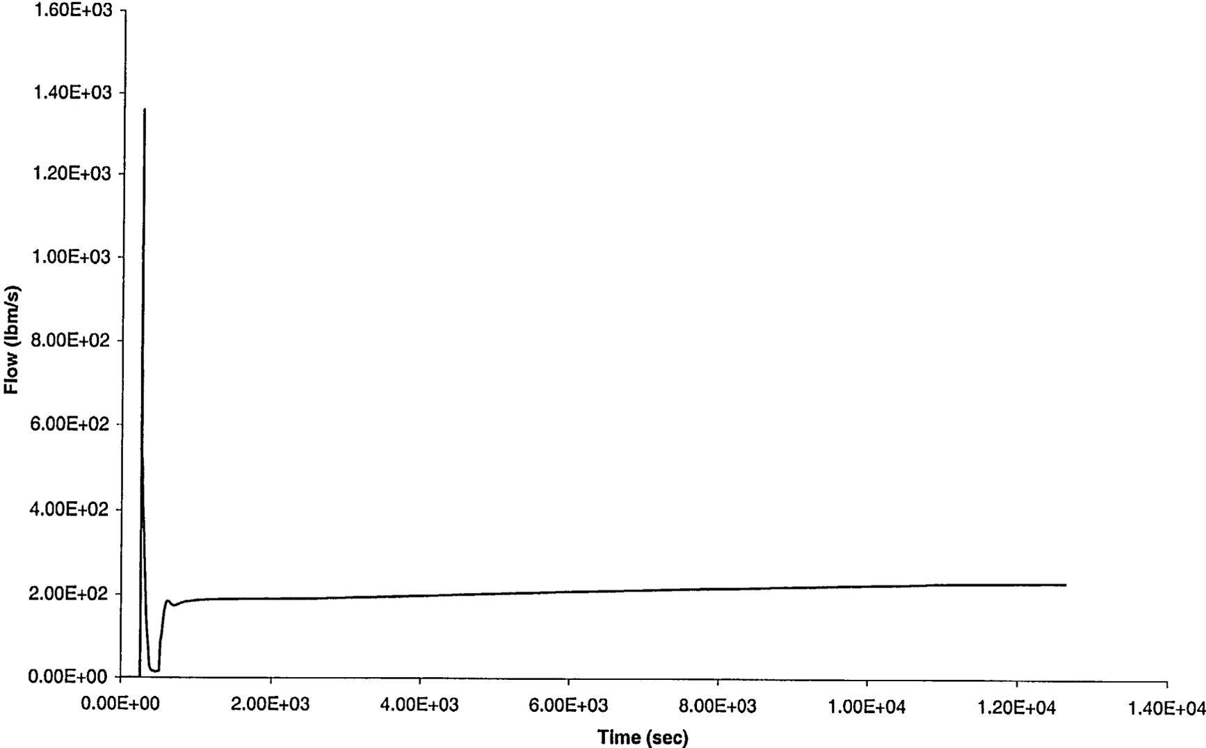
Figure A.7-17: PORV Falsely Lifts and Sticks Open - Burst Disk Flow Quality
