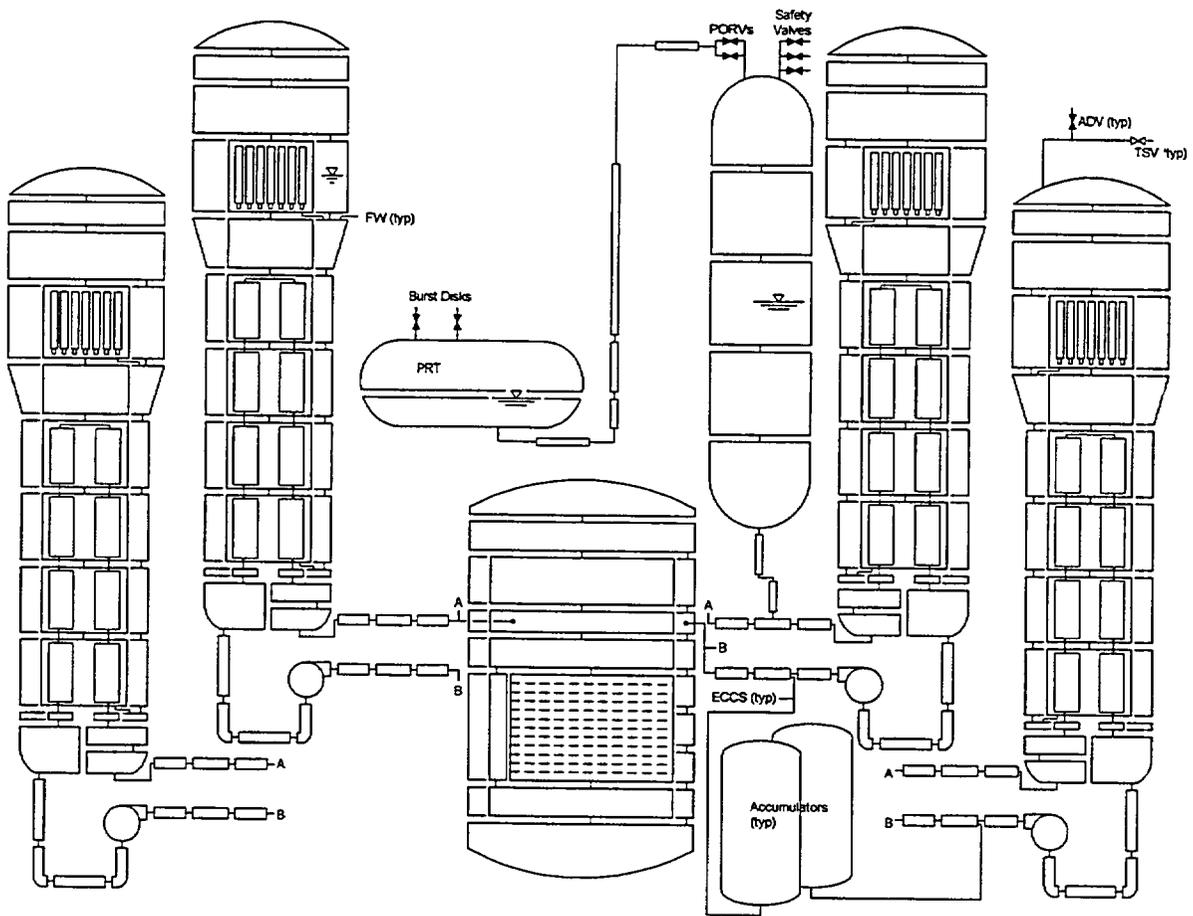
Figure 2 RELAP5 RCS Model Nodalization
