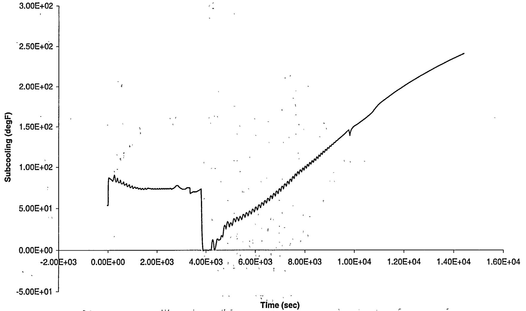
Figure A.6a-13: LOSP with Subsequent AFW Failure, 1 PORV Held Open when it First Lifts - RCS Cooling Rate
