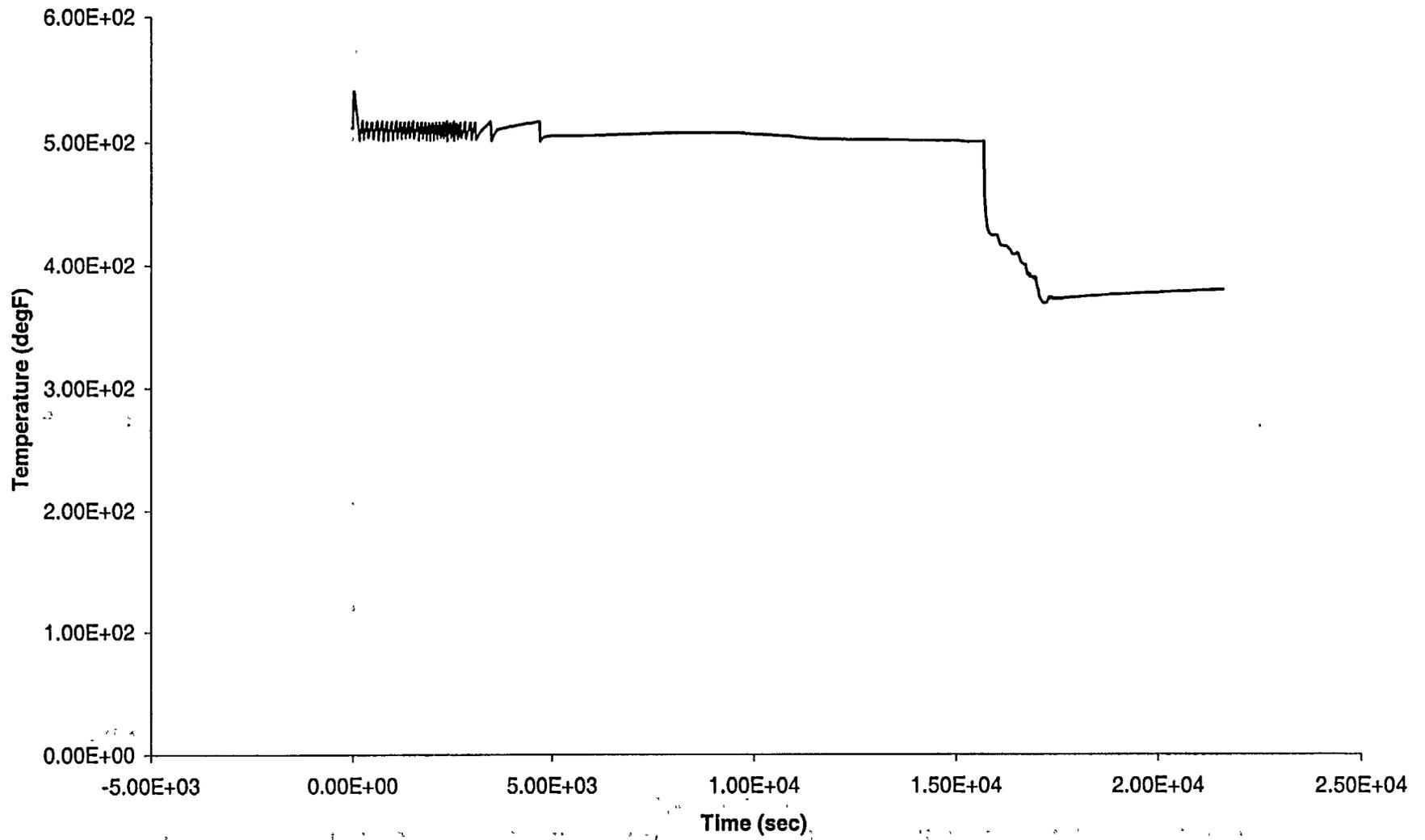
Figure A.6c-11: LOSP with Subsequent AFW Failure, No Operator Action for 2 hrs 30 min - RCP 1 Speed
