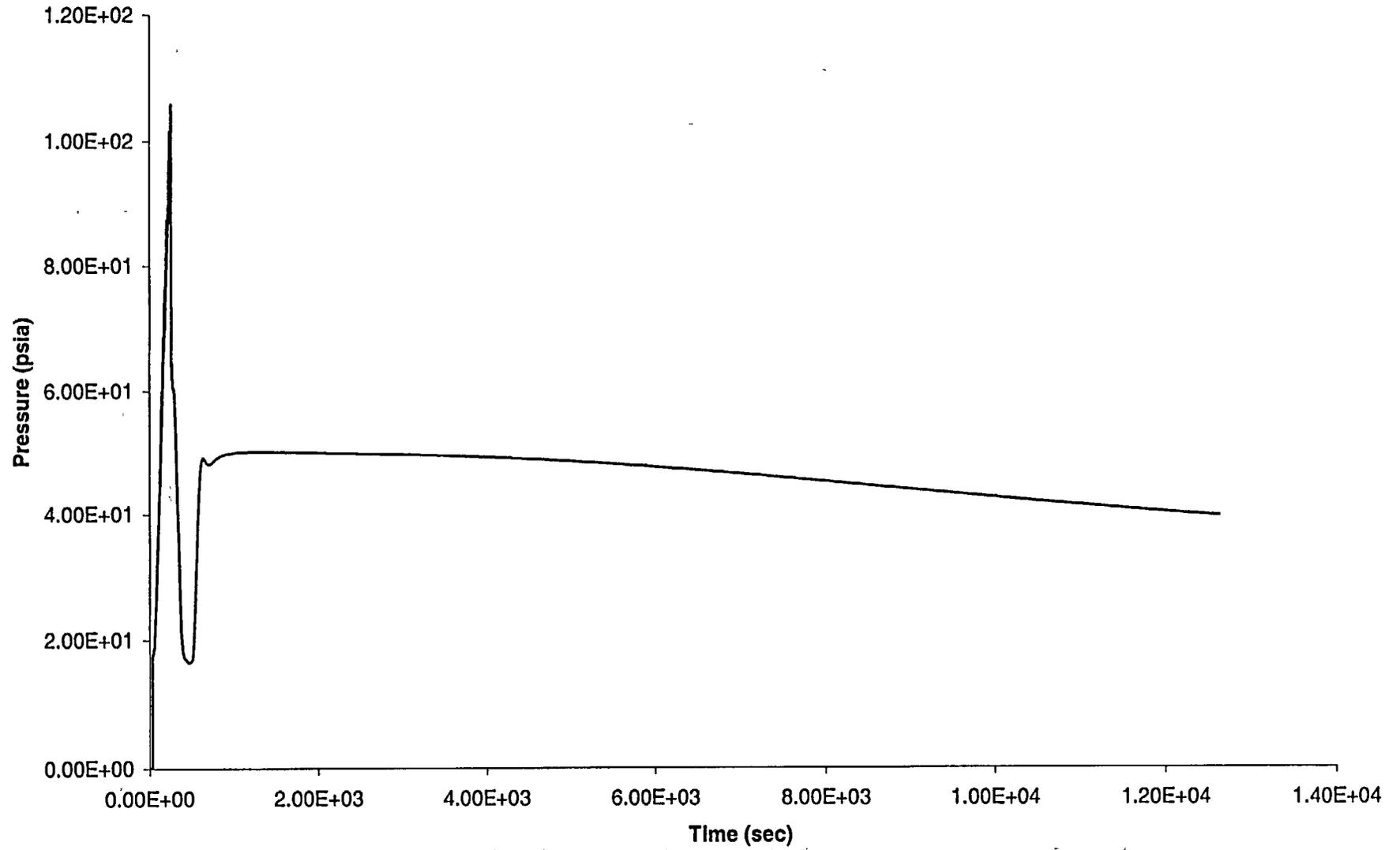
Figure A.7-16: PORV Falsely Lifts and Sticks Open - PRT Burst Disk Flow
