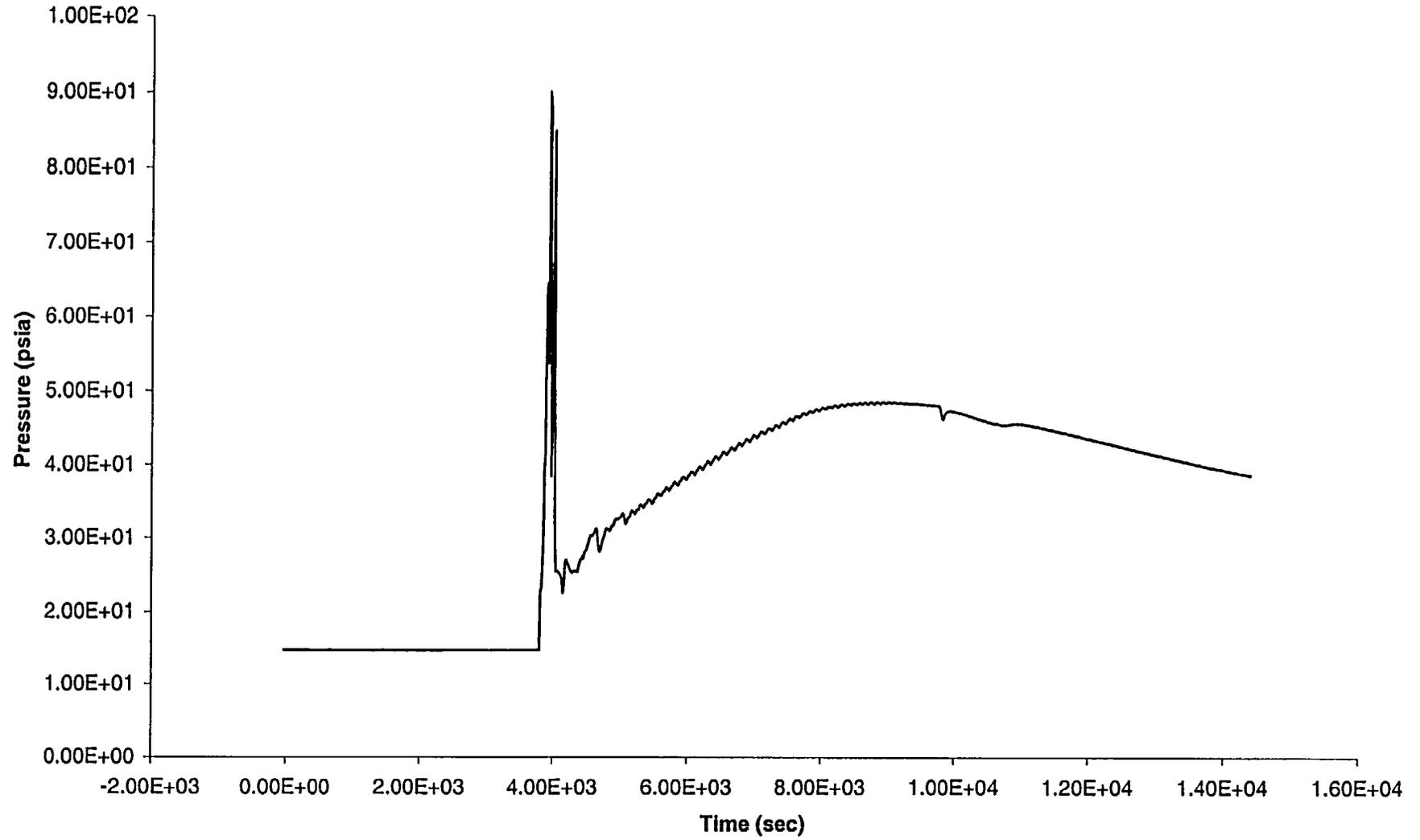
Figure A.6a-16: LOSP with Subsequent AFW Failure, 1 PORV Held Open when it First Lifts - PRT Burst Disk Flow
