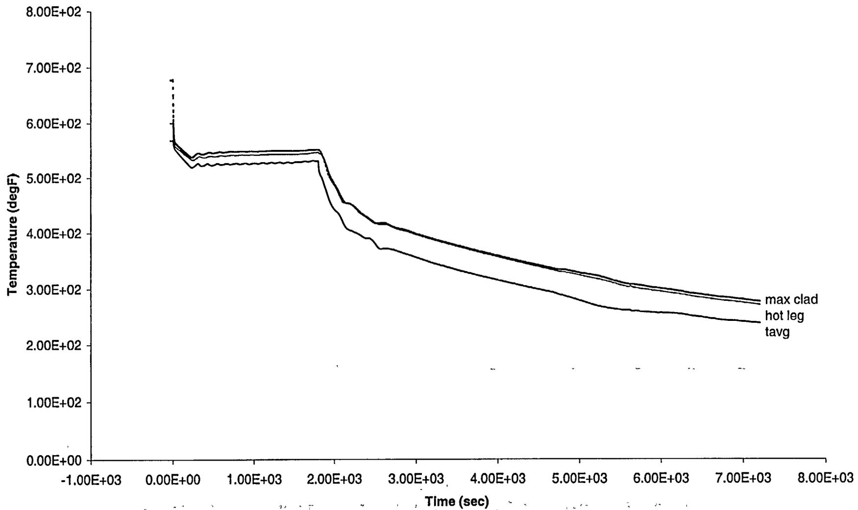
Figure A.6b-6: LOSP with Subsequent AFW Failure, Aggressive Cooling at 30 min - PRZR
