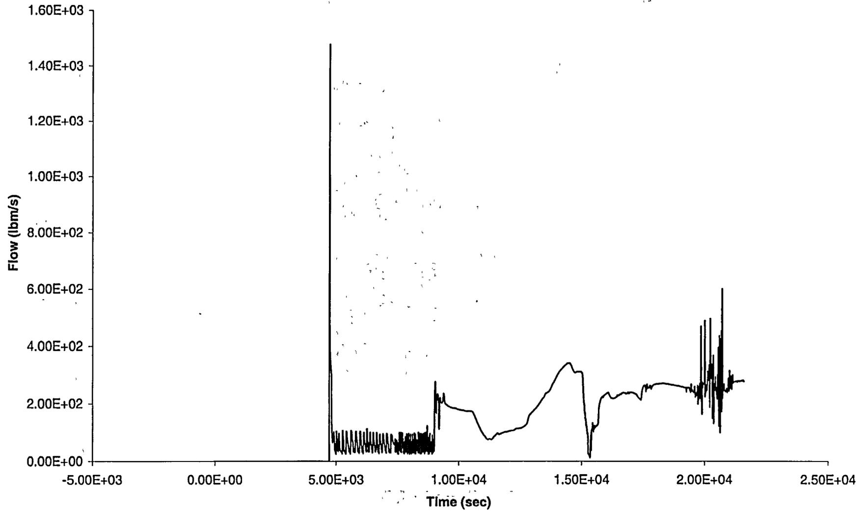
Figure A.6c-17: LOSP with Subsequent AFW Failure, No Operator Action for 2 hrs 30 min - Burst Disk Flow Quality
