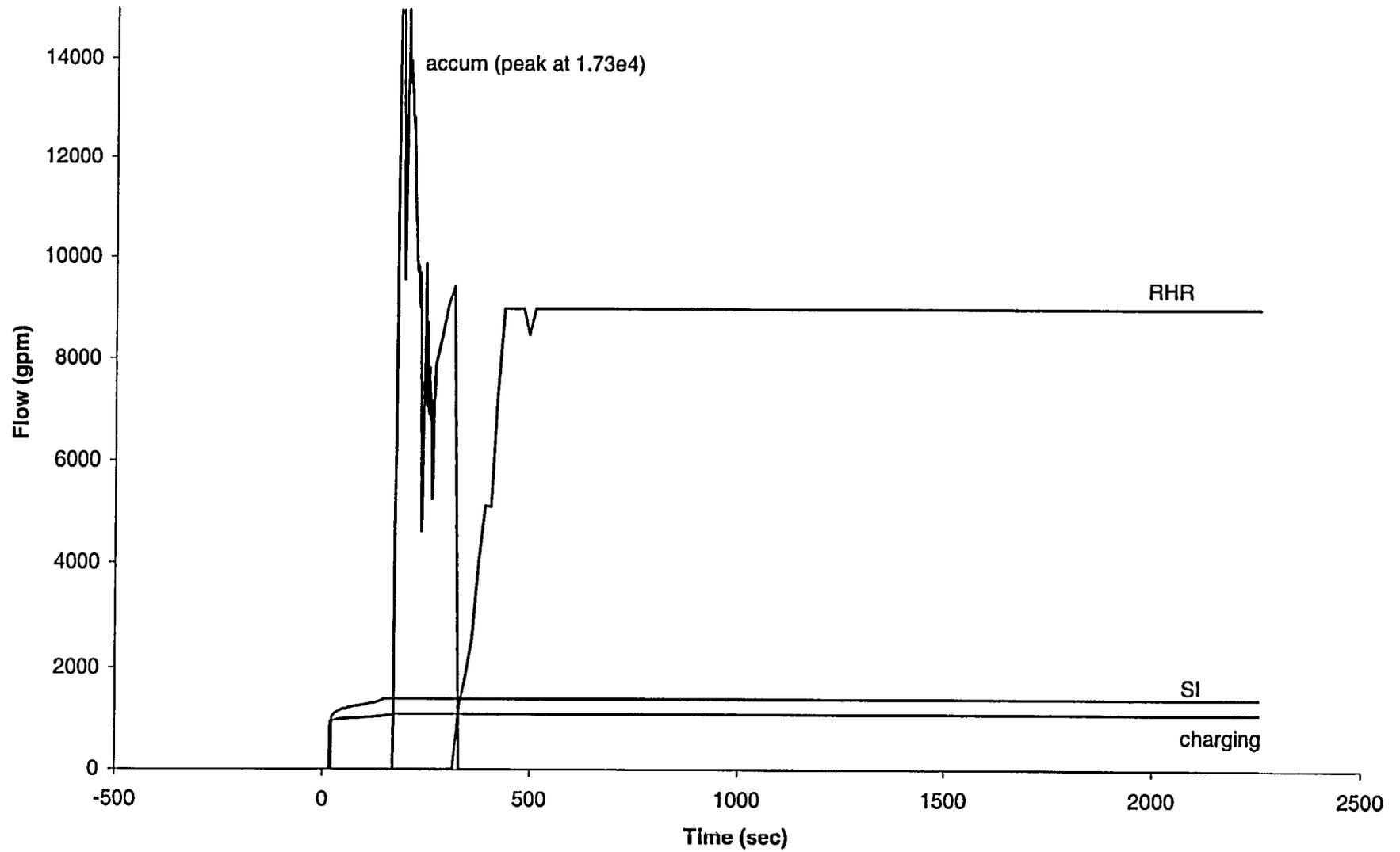
Figure A.5-6: Surge Line Break - Flow Rate at the Break
