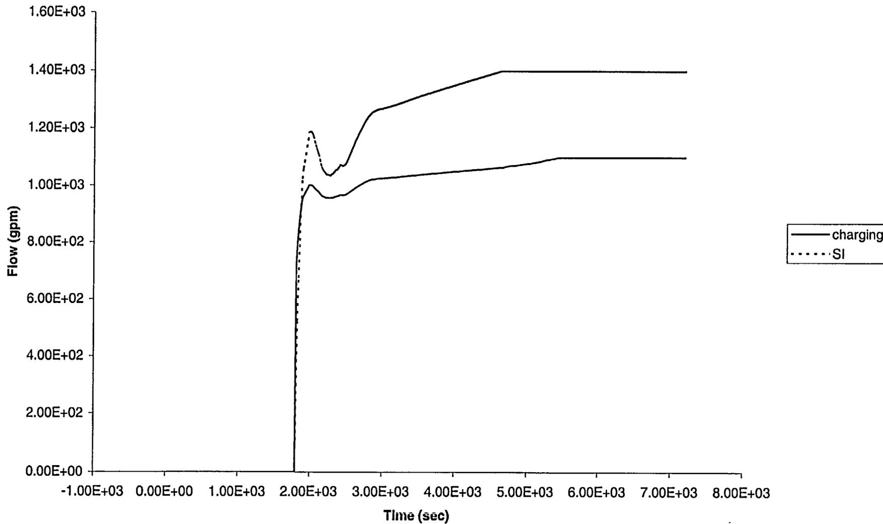
Figure A.6b-5: LOSP with Subsequent AFW Failure, Aggressive Cooling at 30 min - RCS
