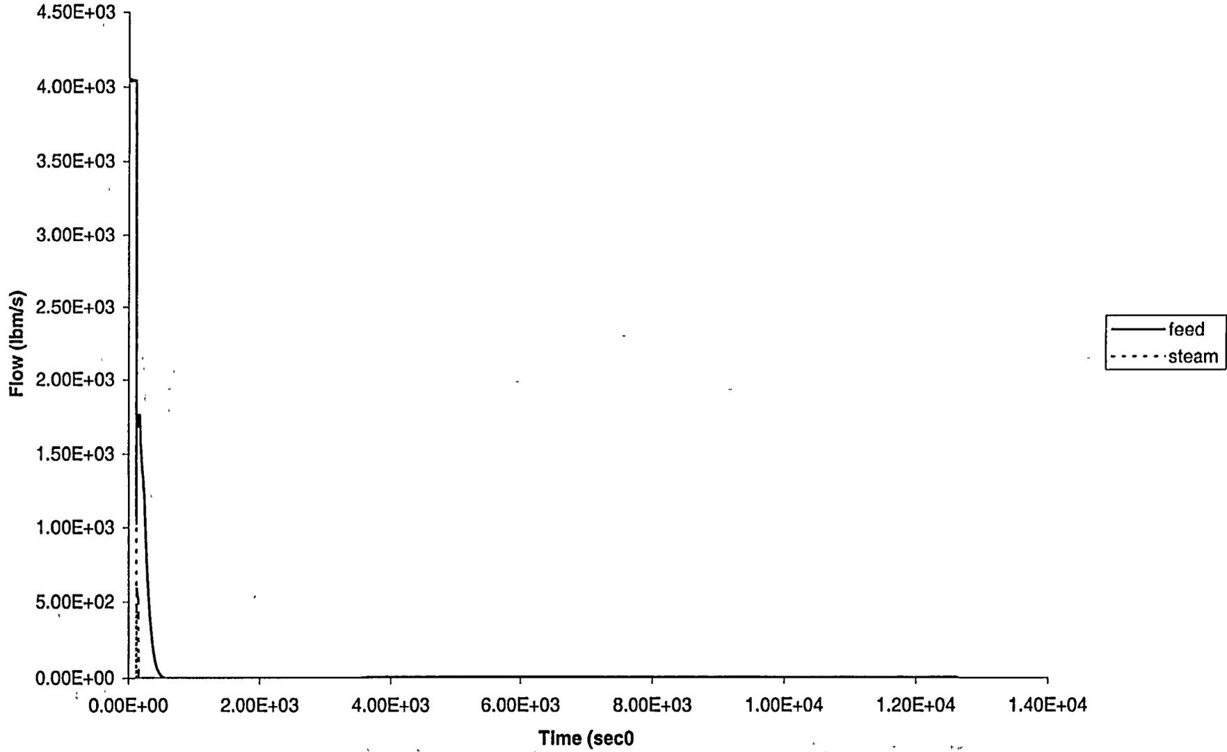
Figure A.7-4: PORV Falsely Lifts and Sticks Open - Charging and SI Flows
