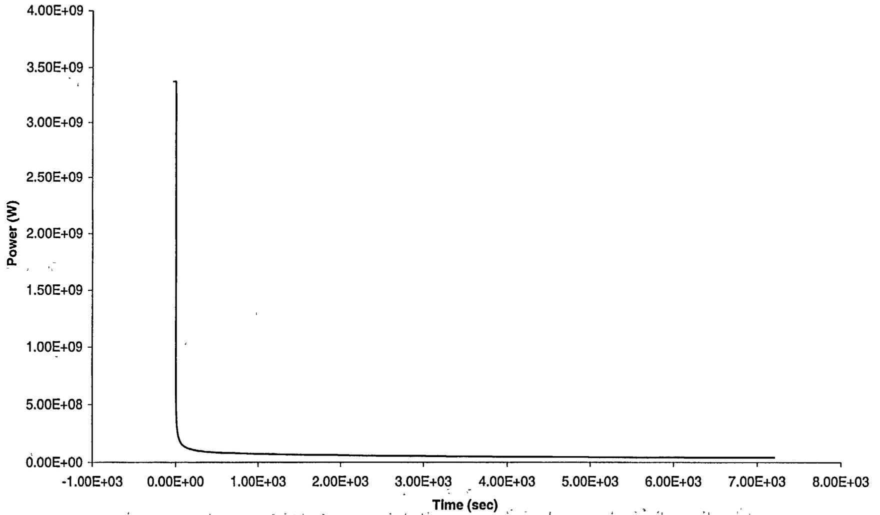
Figure A.6b-2: LOSP with Subsequent AFW Failure, Aggressive Cooling at 30 min - RCS
