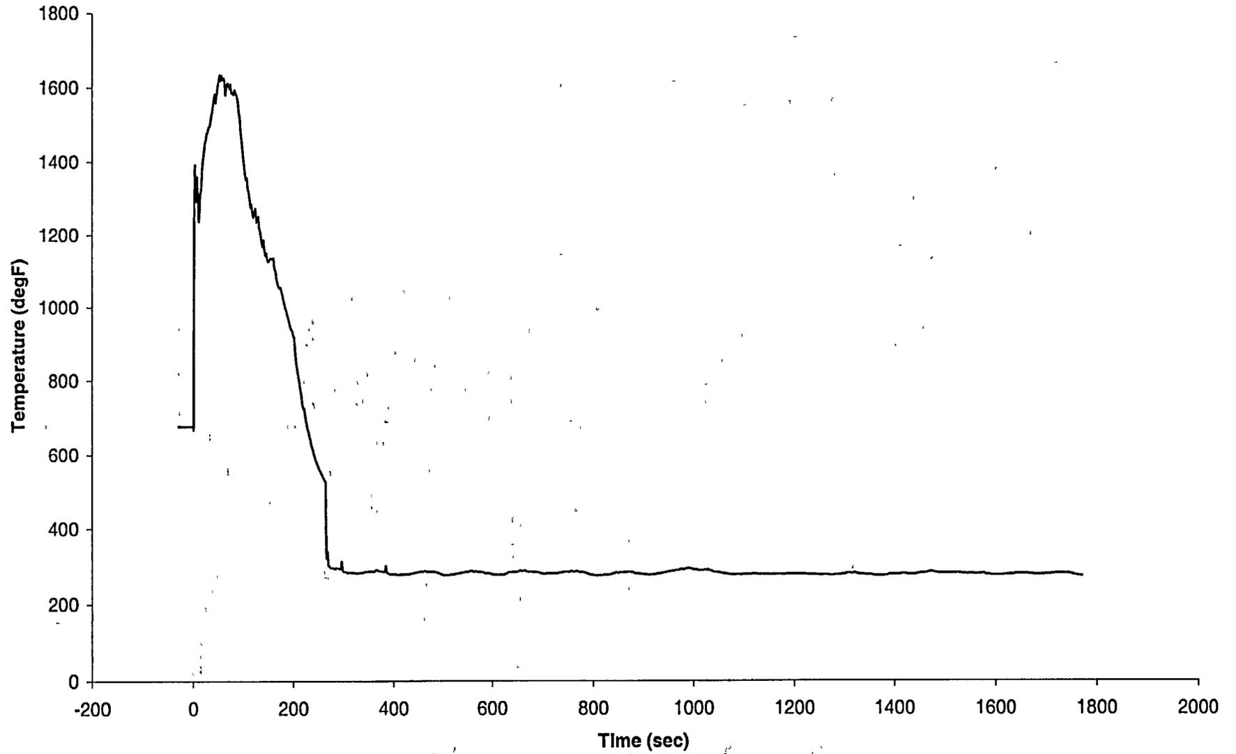
Figure A.1-4: Cold Leg DEGB - Core Void
