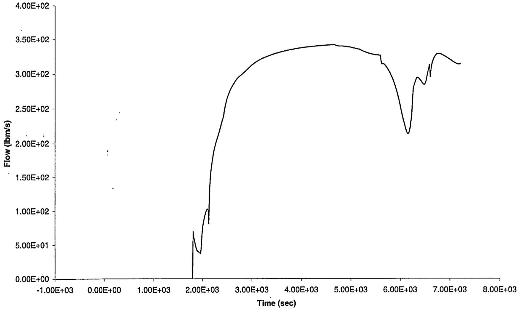
Figure A.6b-8: LOSP with Subsequent AFW Failure, Aggressive Cooling at 30 min - SG 1 WR Level
