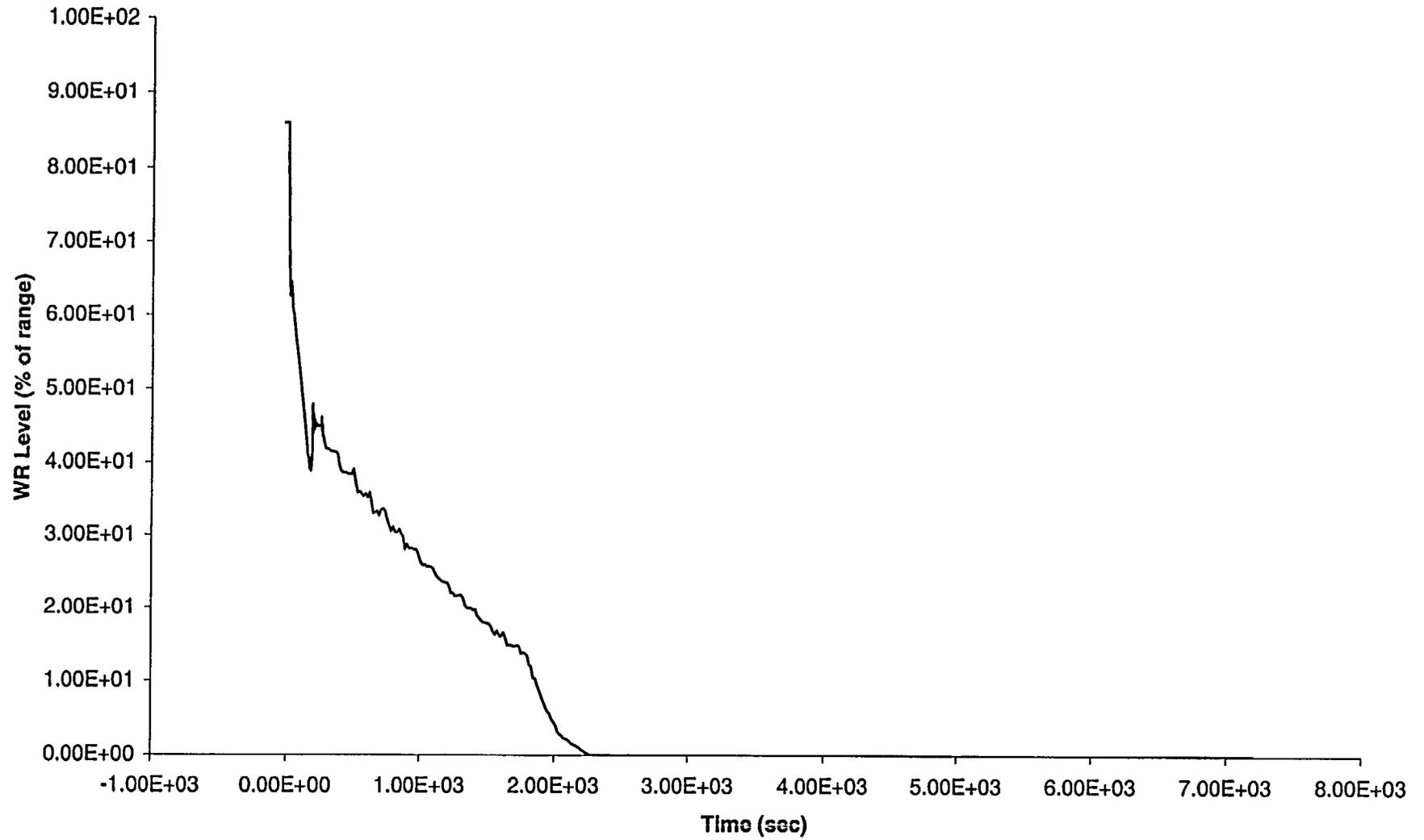
Figure A.6b-9: LOSP with Subsequent AFW Failure, Aggressive Cooling at 30 min - SG 1
