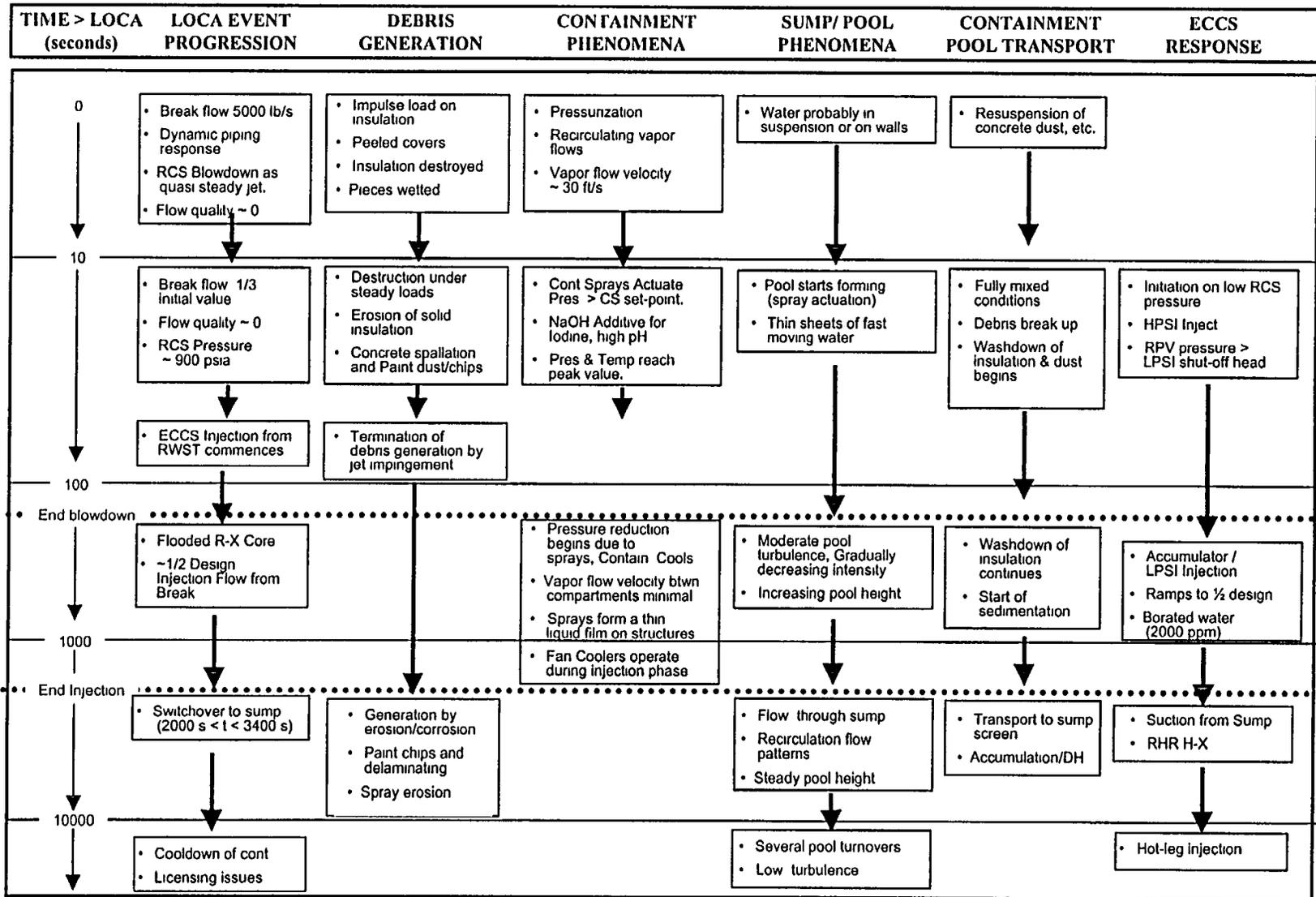
Figure 13 PWR MLOCA Accident Progression in a Large Dry Containment
