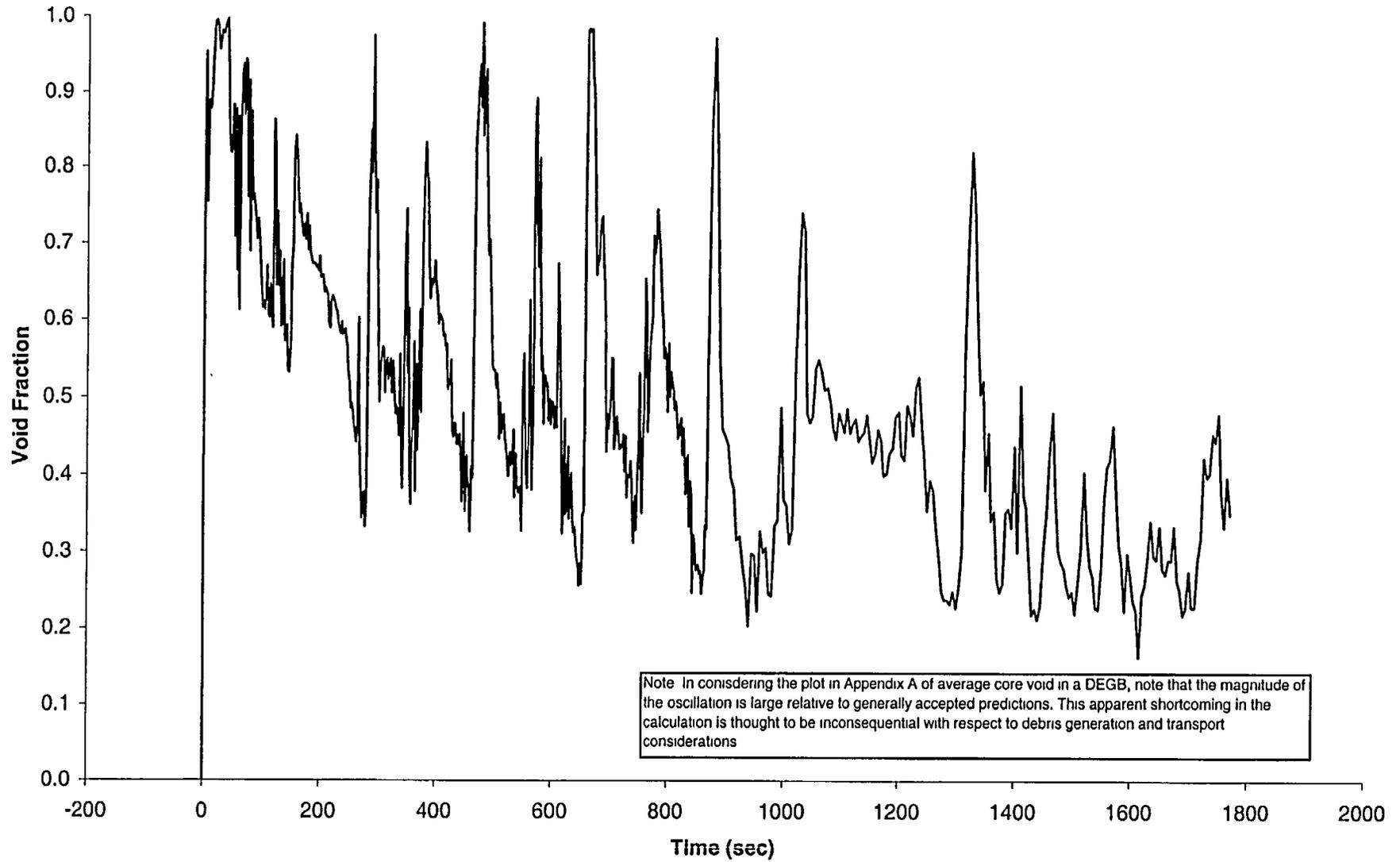
Figure A.1-5: Cold Leg DEGB - Injection
