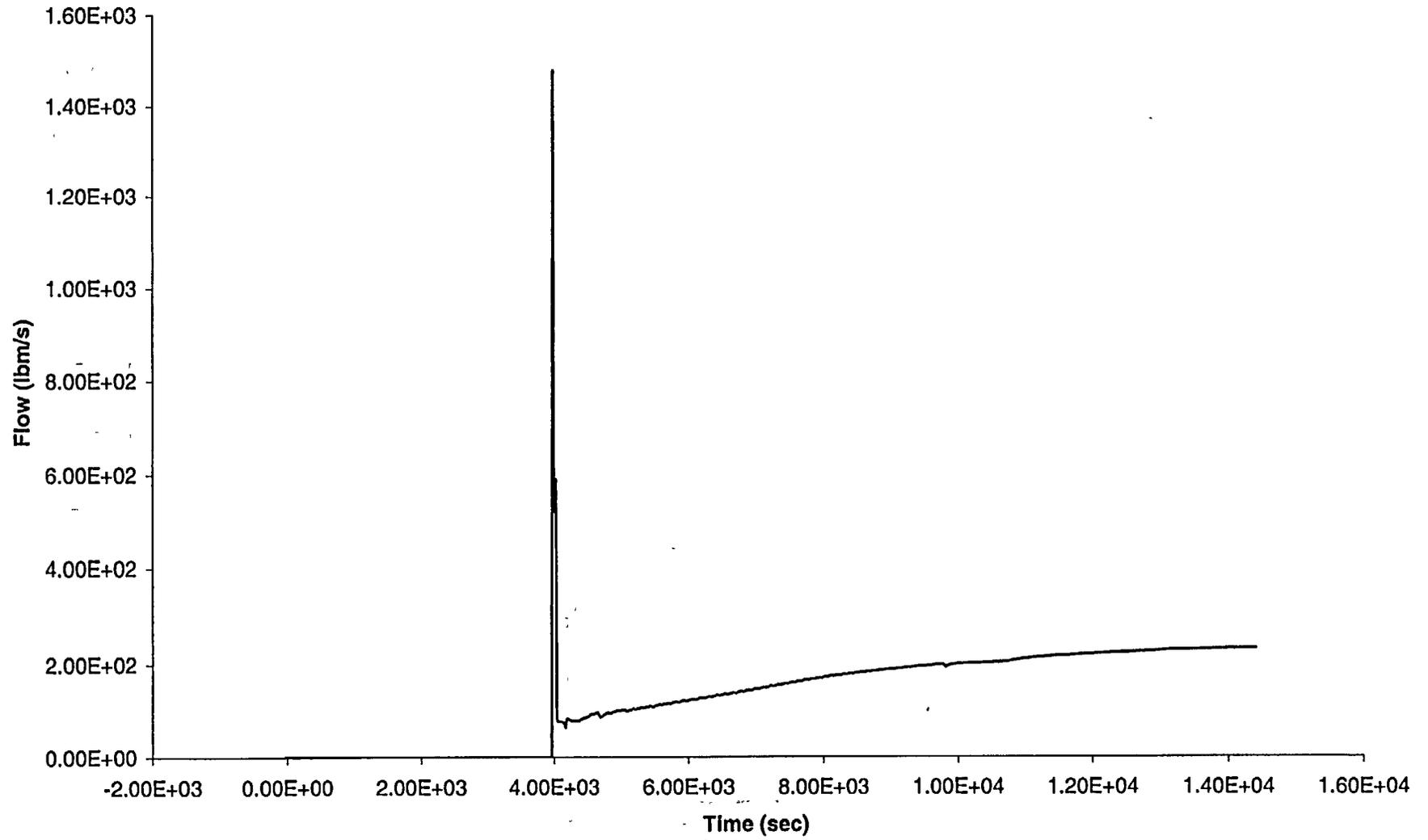
Figure A.6a-17: LOSP with Subsequent AFW Failure, 1 PORV Held Open when it First Lifts - Burst Disk Flow Quality
