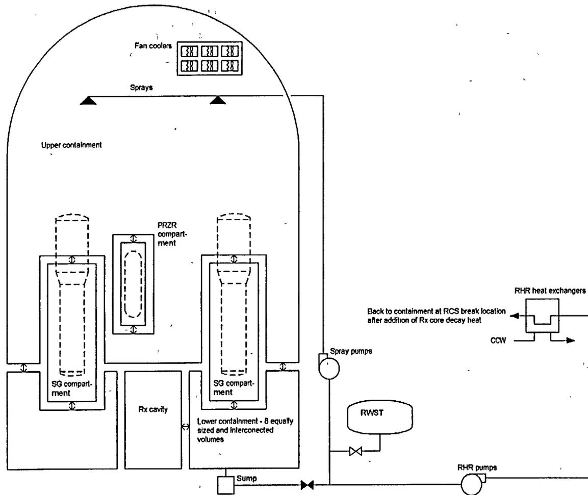
Figure 3 MELCOR Large Dry Containment Nodalization
