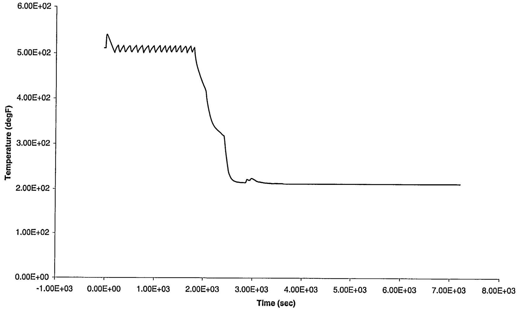
Figure A.6b-11: LOSP with Subsequent AFW Failure, Aggressive Cooling at 30 min - RCP 1
