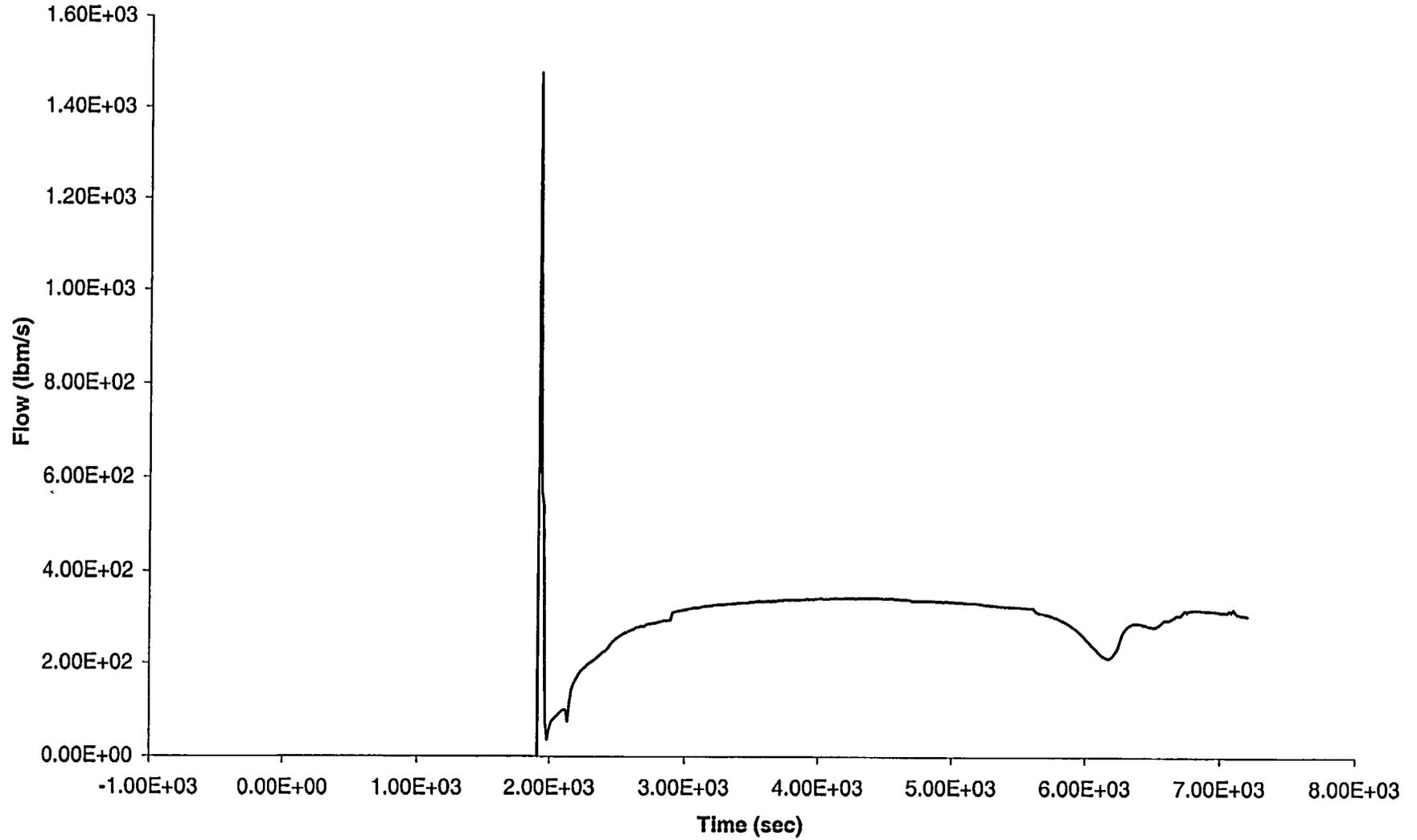
Figure A.6b-17: LOSP with Subsequent AFW Failure, Aggressive Cooling at 30 min - Burst Disk Flow Quality
