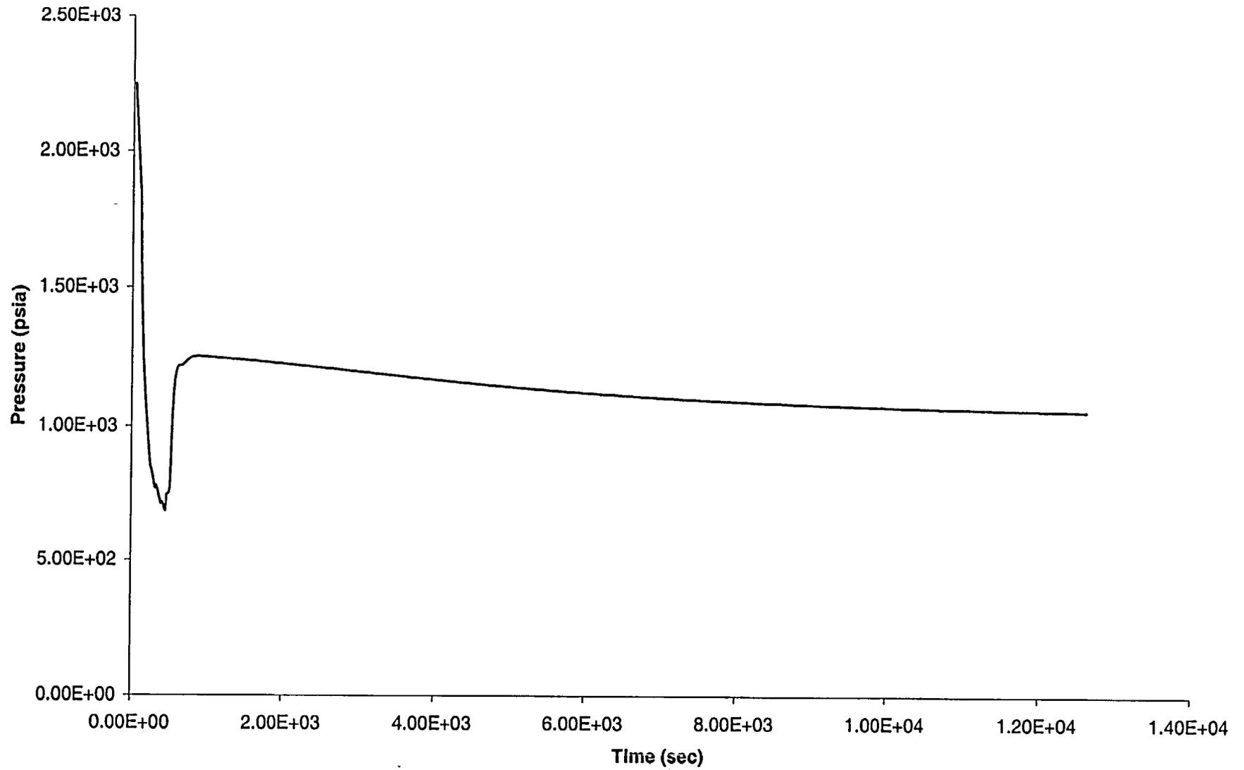
Figure A.7-3: PORV Falsely Lifts and Sticks Open - Feed/Steam Flows
