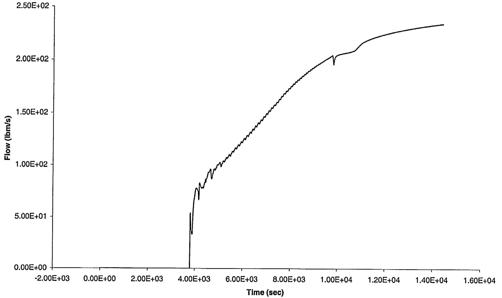
Figure A.6a-8: LOSP with Subsequent AFW Failure, 1 PORV Held Open when it First Lifts - SG
