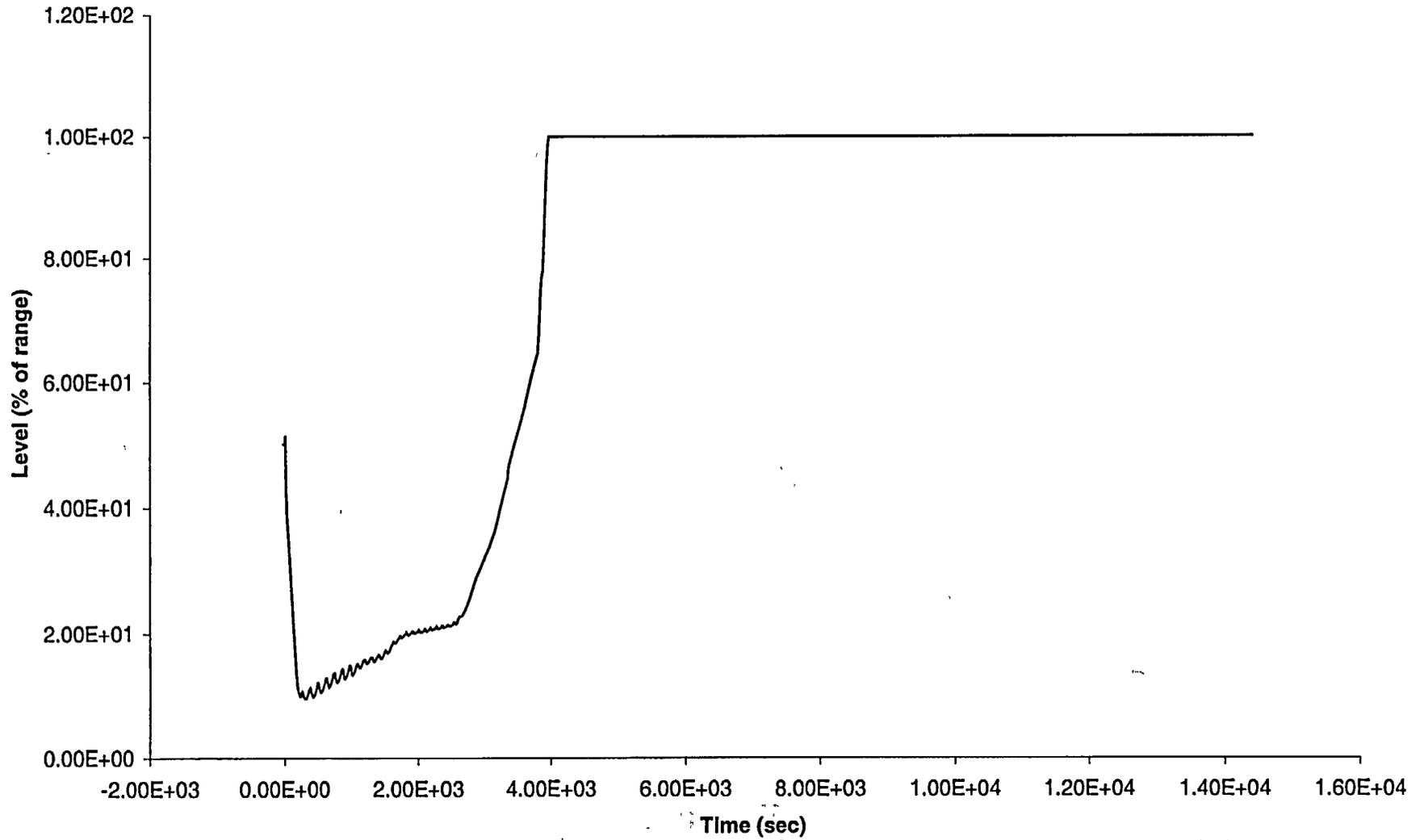
Figure A.6a-7: LOSP with Subsequent AFW Failure, 1 PORV Held Open when it First Lifts - PORV Flow
