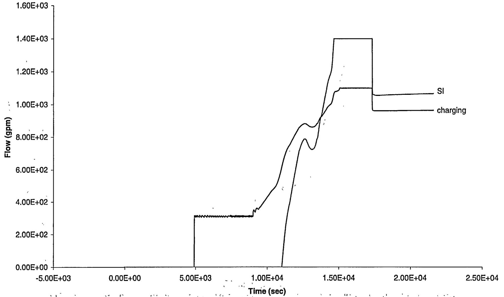
Figure A.6c-5: LOSP with Subsequent AFW Failure, No Operator Action for 2 hrs 30 min - RCS
