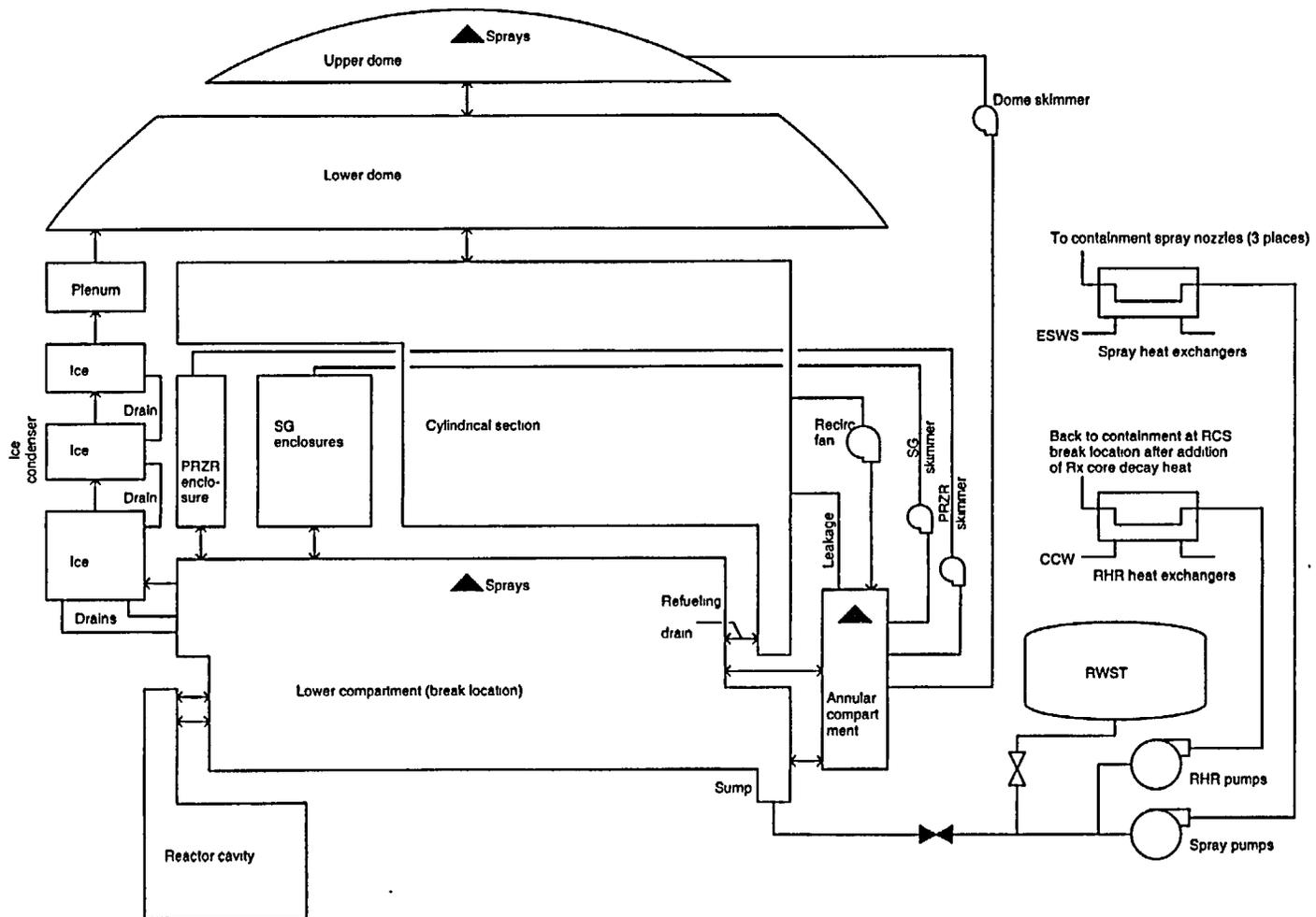
Figure 4 MELCOR Ice-Condenser Containment Nodalization
