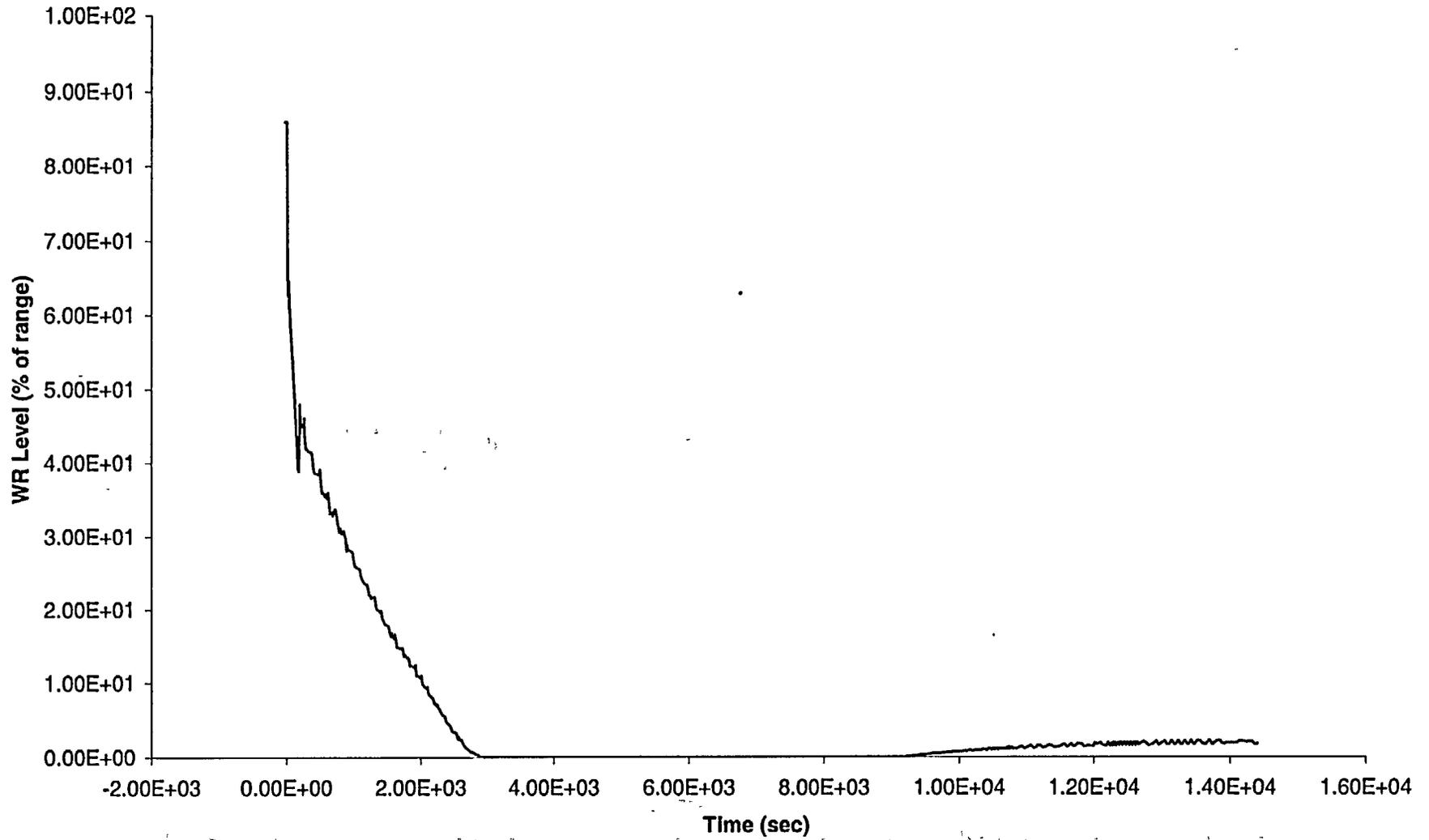
Figure A.6a-9: LOSP with Subsequent AFW Failure, 1 PORV Held Open when it First Lifts - SG
