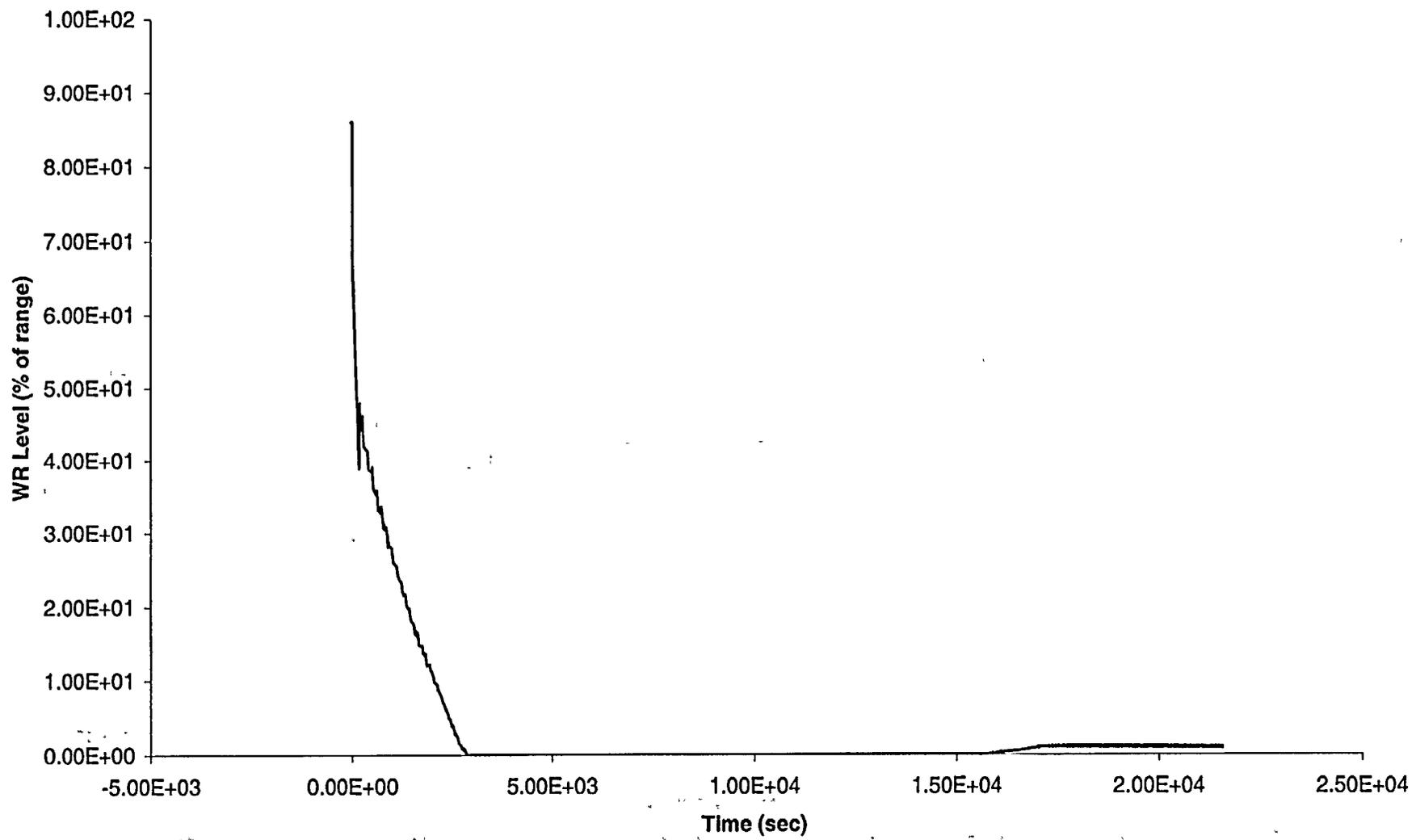
Figure A.6c-9: LOSP with Subsequent AFW Failure, No Operator Action for 2 hrs 30 min - SG
