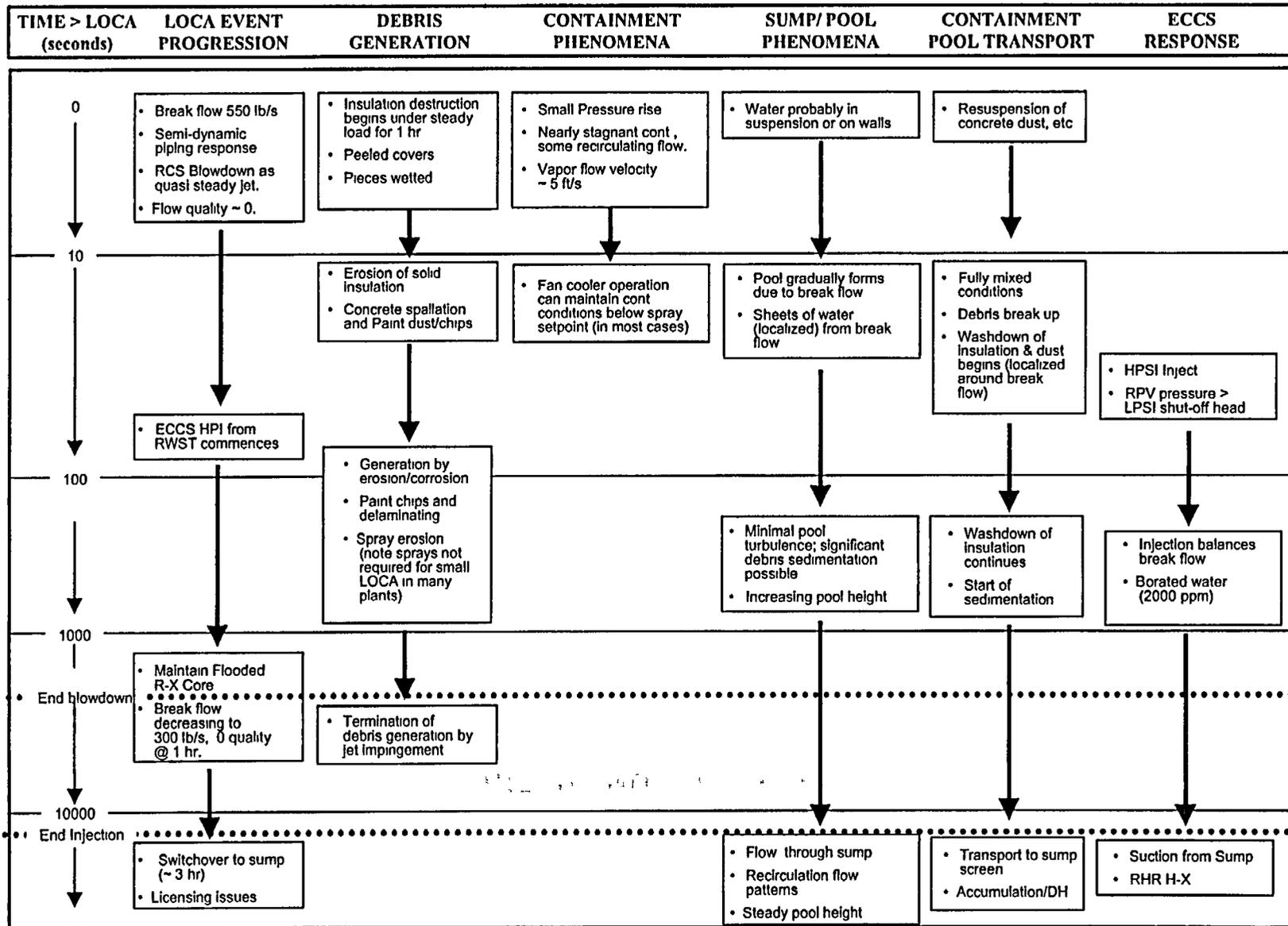
Figure 14 PWR SLOCA Accident Progression in a Large Dry Containment
