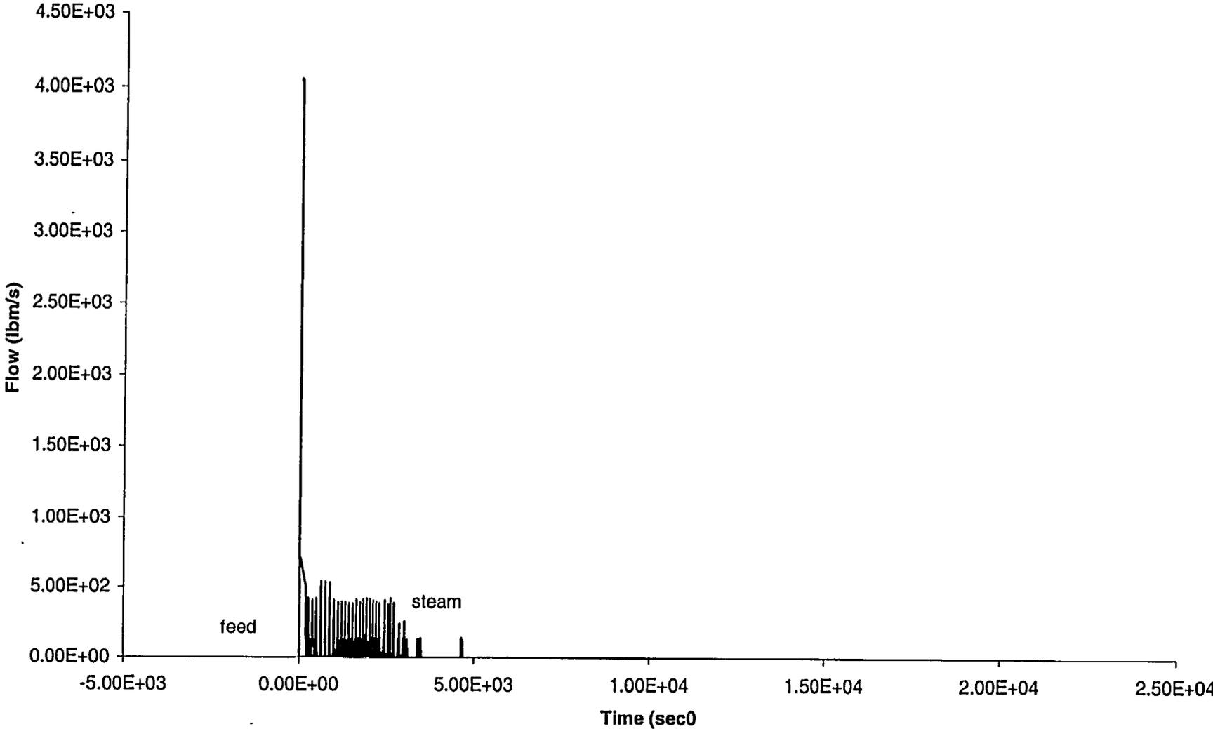
**Figure A.6c-4: LOSP with Subsequent AFW Failure, No Operator Action for 2 hrs 30 min -
