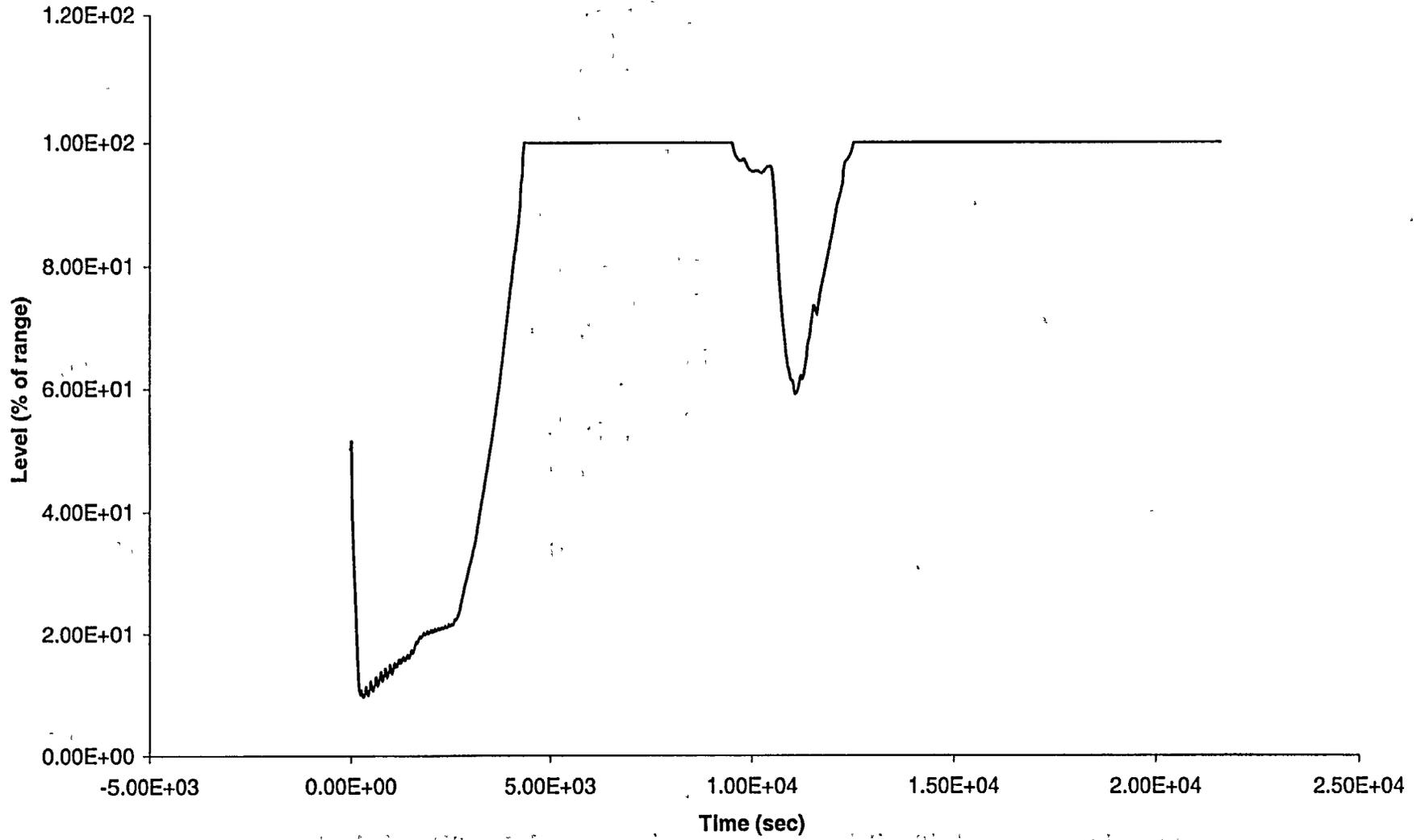
Figure A.6c-7: LOSP with Subsequent AFW Failure, No Operator Action for 2 hrs 30 min - PORV Flow
