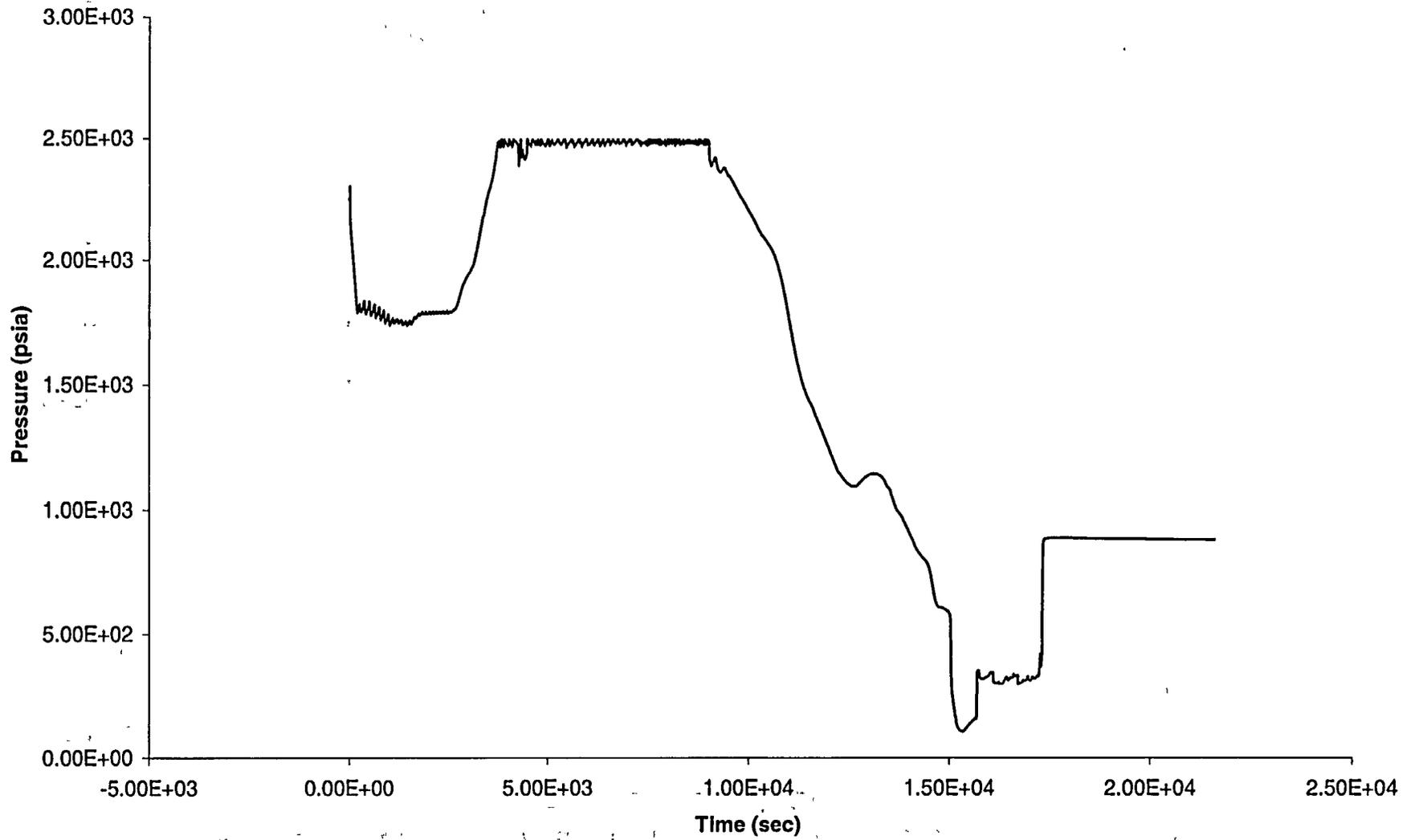
Figure A.6c-3: LOSP with Subsequent AFW Failure, No Operator Action for 2 hrs 30 min - Feed/Steam Flows
