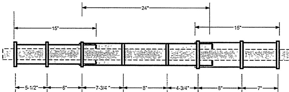
Figure A-4 Typical Band Configuration for Seam Offset Tests
