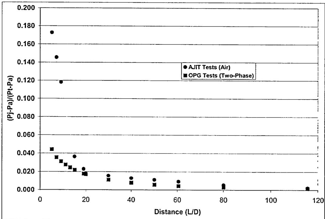
Figure 3-2 Comparison of OPG and AJIT Target Pressures
