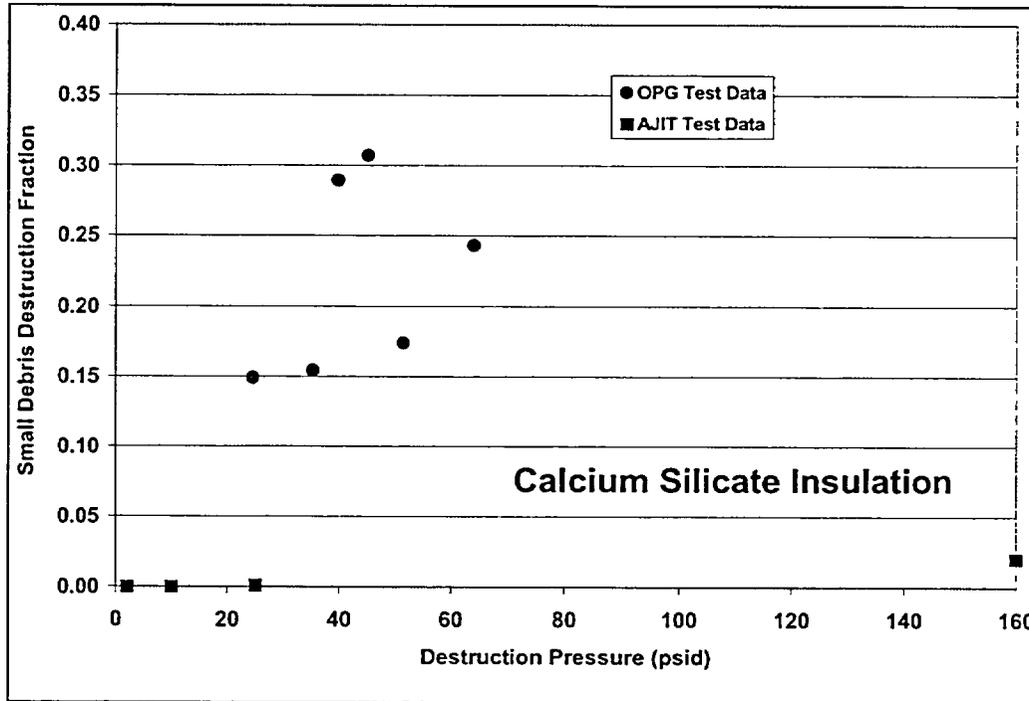
Figure 3-4 Small Debris Destruction Fractions for Calcium-Silicate Insulation
