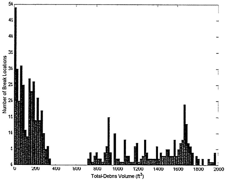
Figure 2-3 Frequency Distribution of Possible Breaks from Large-Pipe Breaks in the Volunteer Plant
