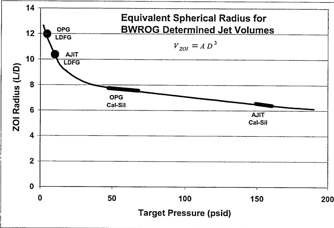
Figure 3-3 Equivalent Spherical Radius Dependence on Insulation Destruction Pressure
