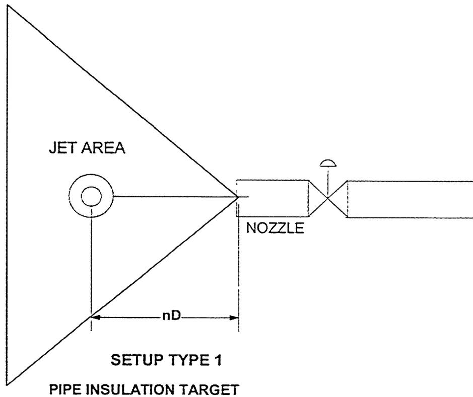
Figure A-3 Target Mount Geometry
