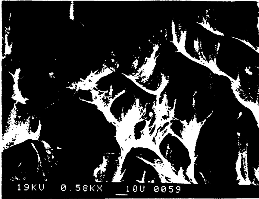
Fig. 3. SEM image of long fibers of mordenite in fracture from 1788 ft.
