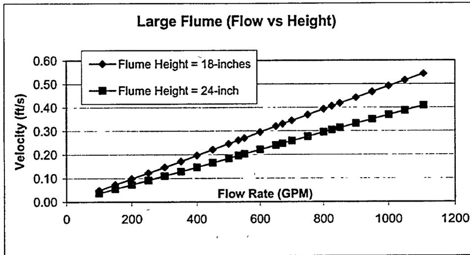
Figure A.17 Large Flume Flow Velocity Vs Volumetric Flow Rate
