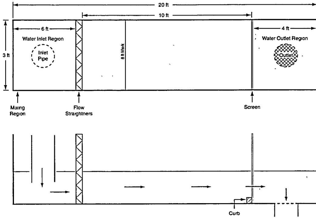
Schematic of the Converging Channel
