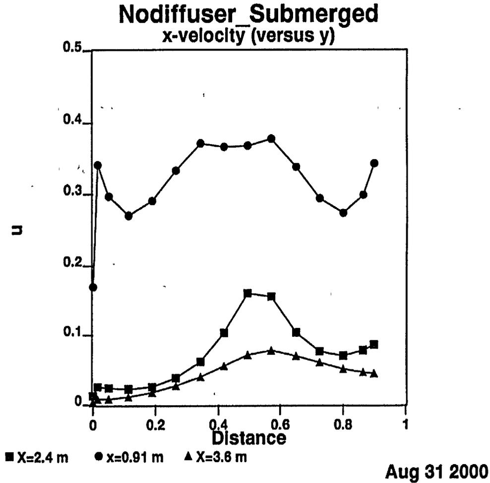
Figure F.3.8 UNM Flume Without Diffuser/With Inlet Submerged - Axial Velocity Just Up from the Floor of the Flume Versus Width at Different Axial Locations
