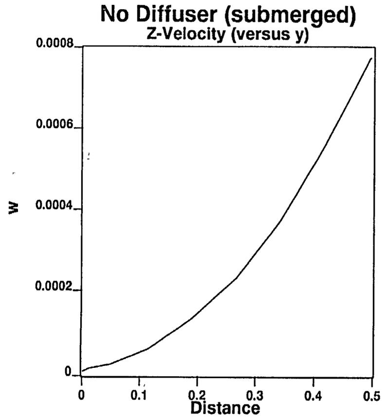
Figure F.3.9 UNM Flume Without Diffuser/With Inlet Submerged - Transverse (Y) and Vertical (Z) Velocities Near the Floor of the Flume Versus Width in Test Region
