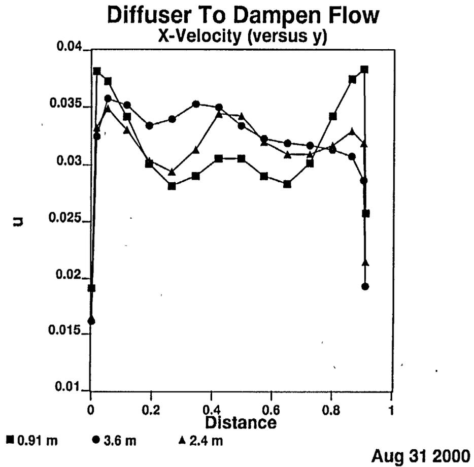
Figure F.1.6. UNM Flume With Diffuser - Axial Velocity Just Up from the Floor of the Flume Versus Width at Different Axial Locations
