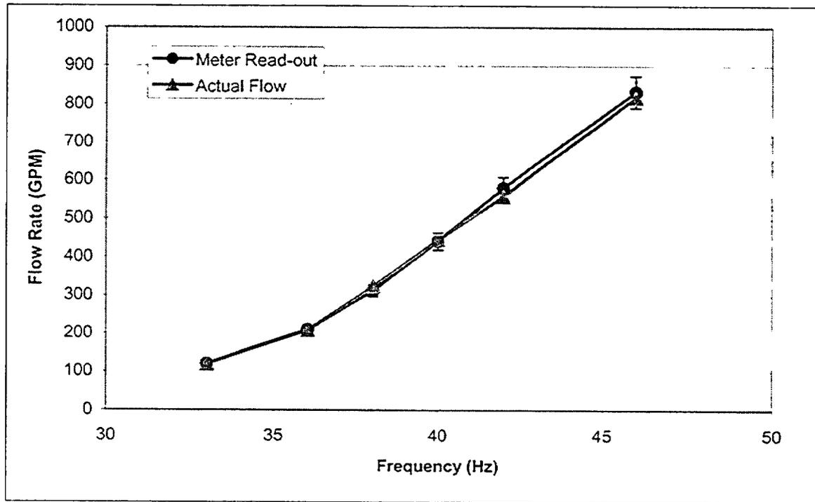
Figure E.1 Comparison of Meter Readout with Actual Flow Measurements
