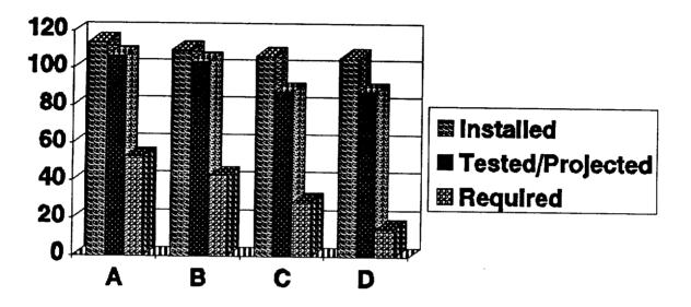
In the most limiting case, the C battery still has greater than 50 percent margin between the projected and required capacities. Therefore, the proposed change to battery capacity requirements does not involve a significant reduction in a margin of safety.
