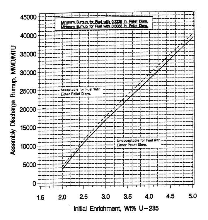
FIGURE 3.9-2 MINIMUM REQUIRED ASSEMBLY DISCHARGE BURNUP AS A FUNCITON OF INITIAL ENRICHMENT AND PELLET DIAMETER TO PERMIT STORAGE IN REGION 2
