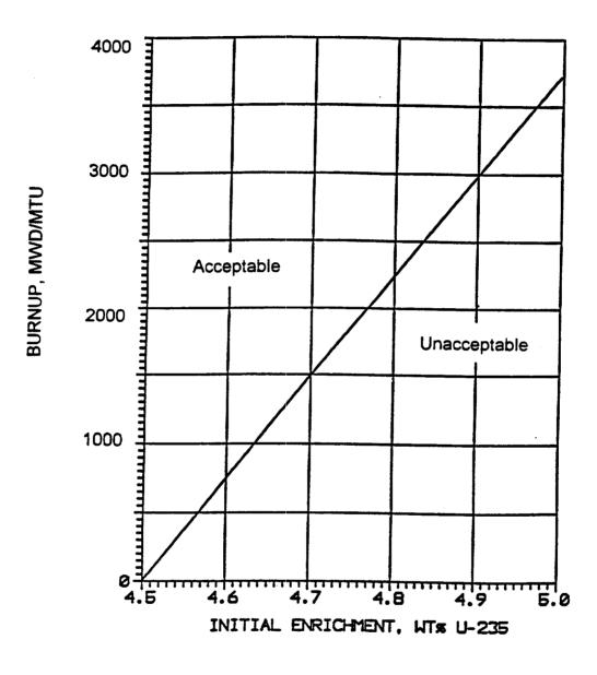
FIGURE 3.9-3 MINIMUM REQUIRED ASSEMBLY DISCHARGE BURNUP AS A FUNCTION OF INITIAL ENRICHMENT (NO IFBA) TO PERMIT STORAGE IN REGION 1
