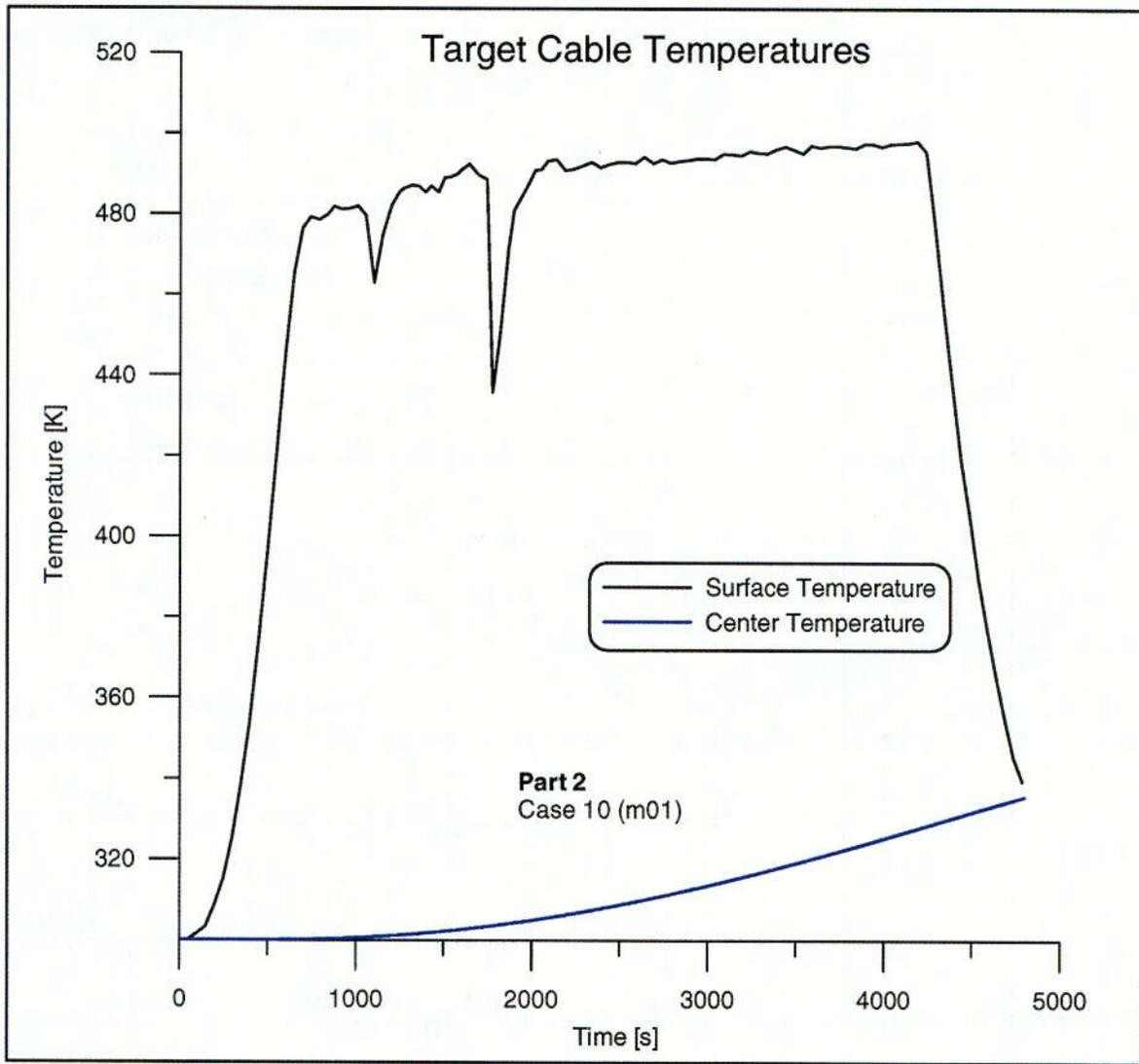
Fig. 27 Target temperatures over time for case 10
