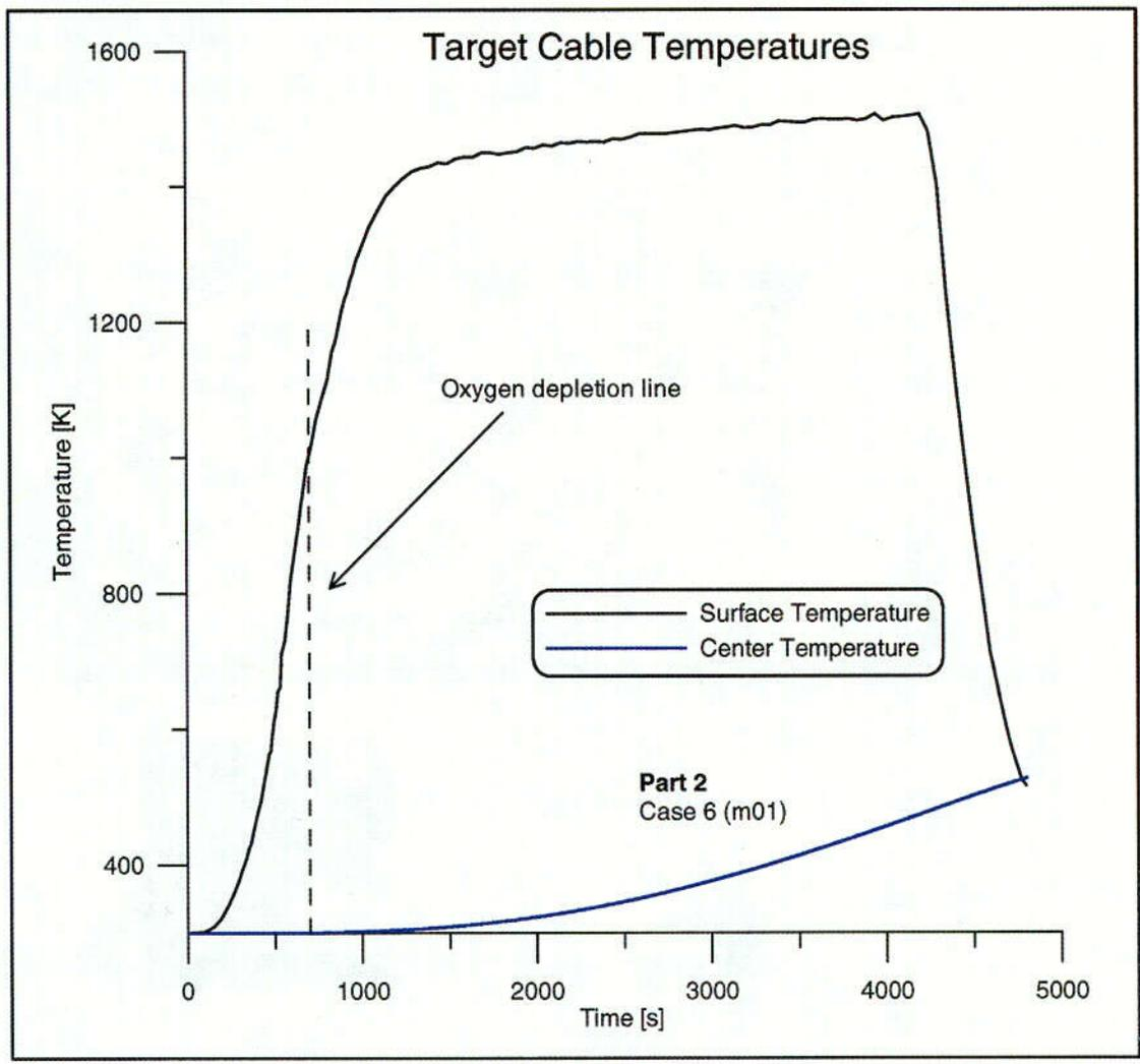
Fig. 22 Target cable temperatures for case 6
