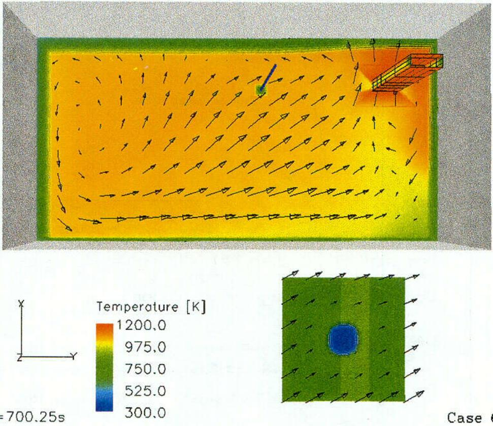
Fig. 21 Temperature distribution after 700 s for case 6
