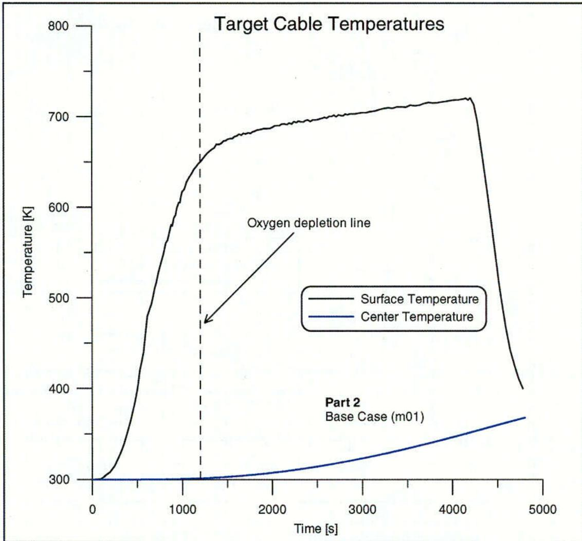
Fig. 20 Target cable temperatures during the base case of part 2
