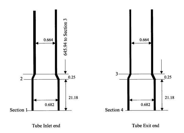
Figure 3 Dimensions of Un-sleeved Tube
