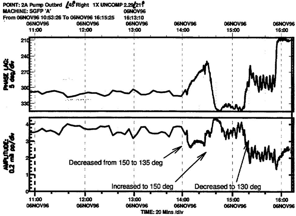
Figure 7. Varying Seal Water Temperature - 2A SGFP
