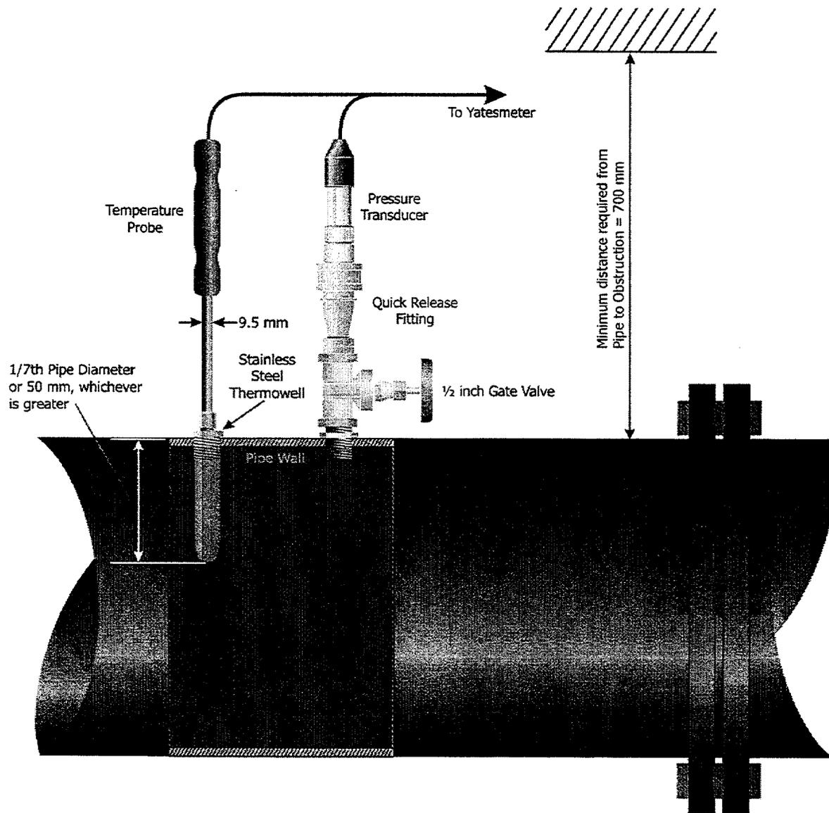
Figure 6 Contaminated Pumps Tapping Method
