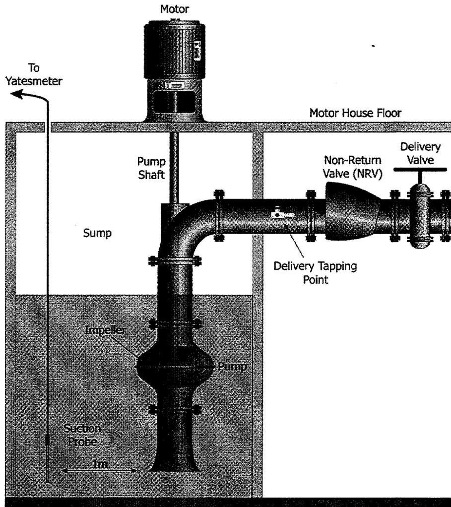
Figure 5 Vertical Wet Well Pump Tapping Arrangement
