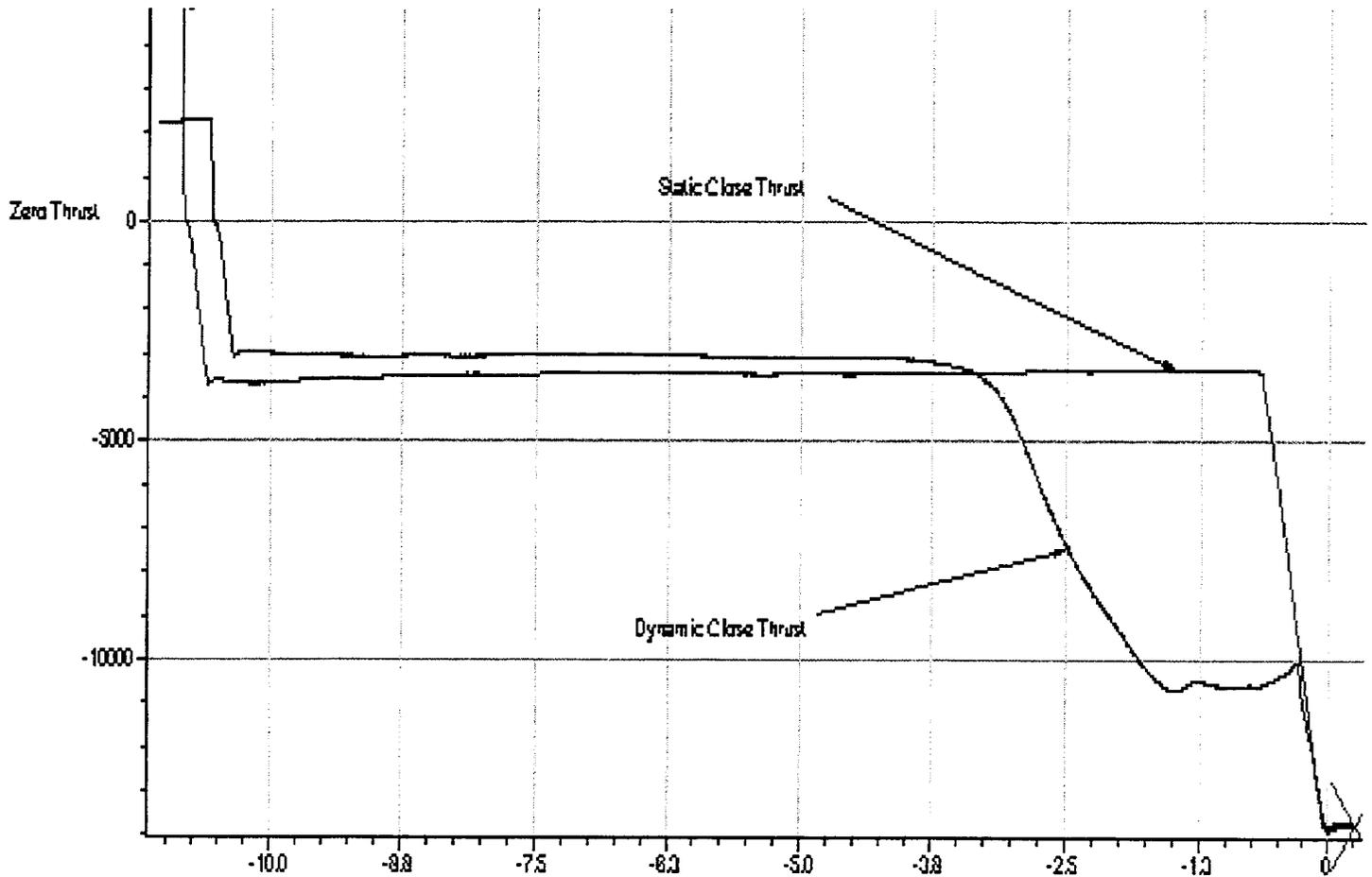
**Stem Torque Overlay (Static and Dynamic)**
