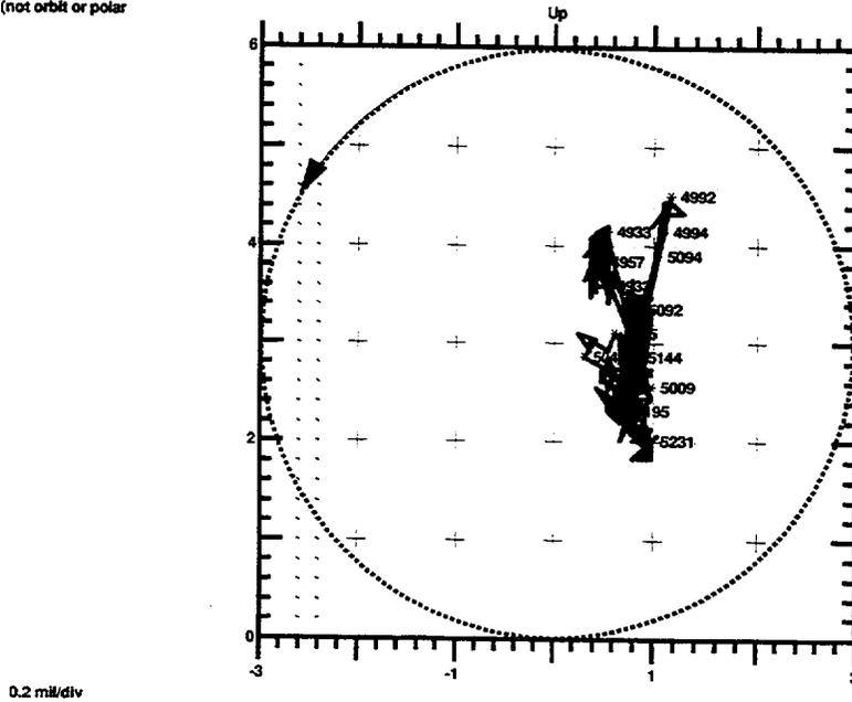
Figure 6. Shaft Centerline Plot During Step Change in Vibration - 2B Outboard Bearing
