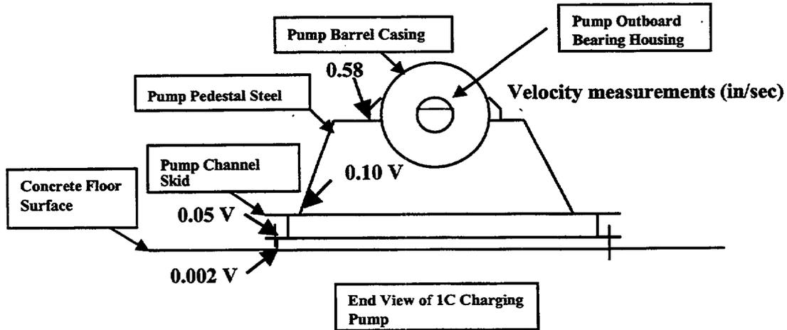
Figure 3. Vibration at FNP CCP Bolted Connections
