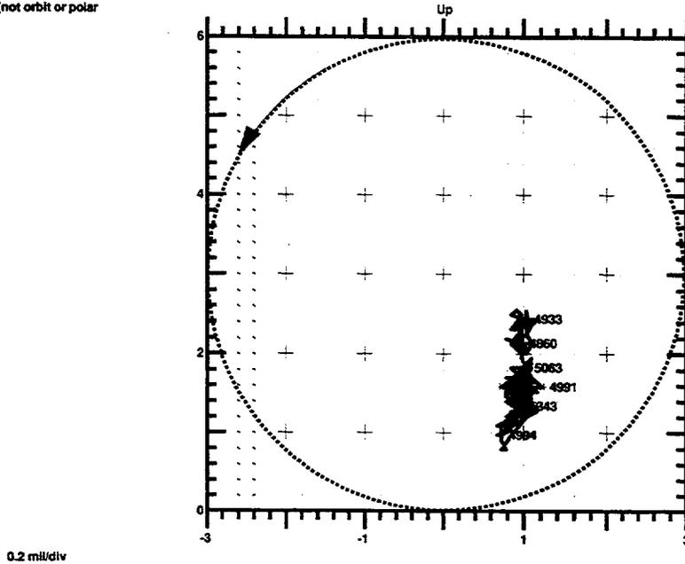
Figure 5. Shaft Centerline Plot During Step Change in Vibration - 2B Inboard Bearing
