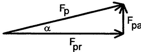
From VOTES test data..  $F_{pa} := 25lbf$  (Typical of the "low" close direction axial packing friction noted in MOV testing.)
