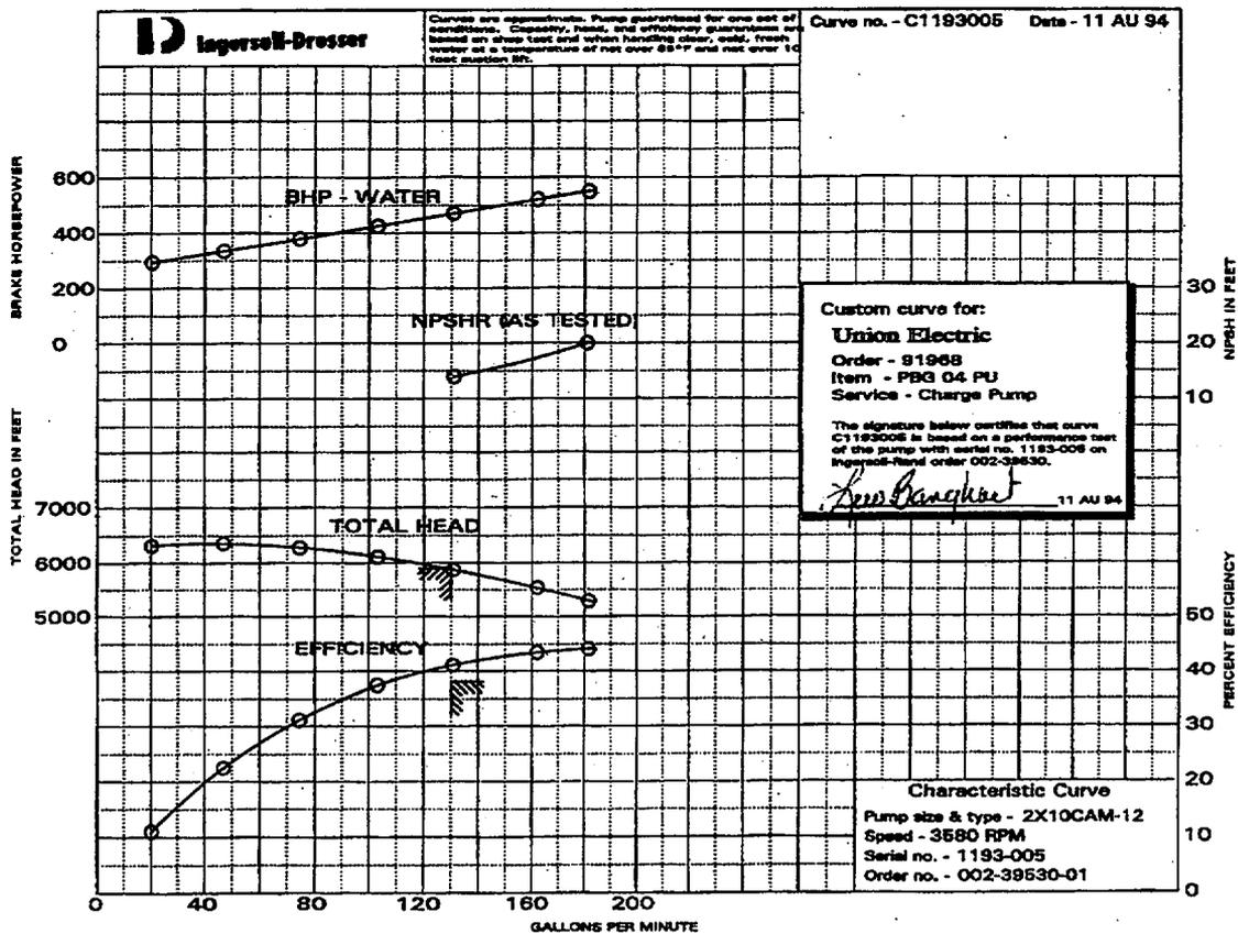
Figure 4. Typical Performance Curve for Normal Charge Pump, model 2X10CAM-12.
