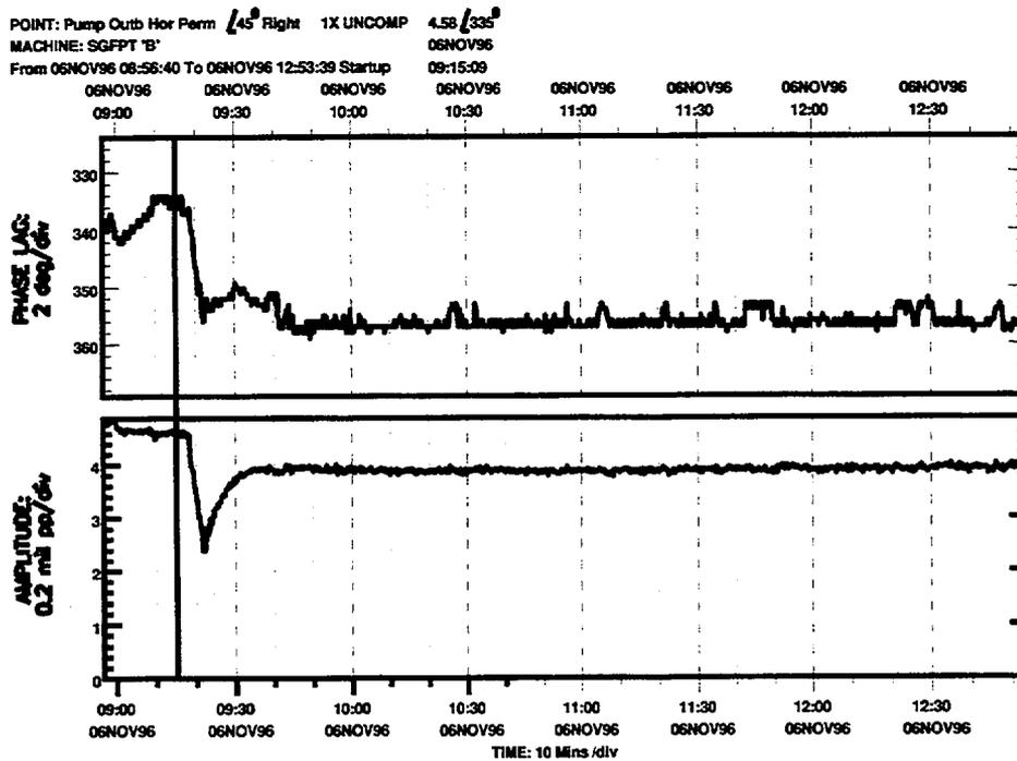
Figure 4. Reducing 2B SGFP Seal Water Temperature
