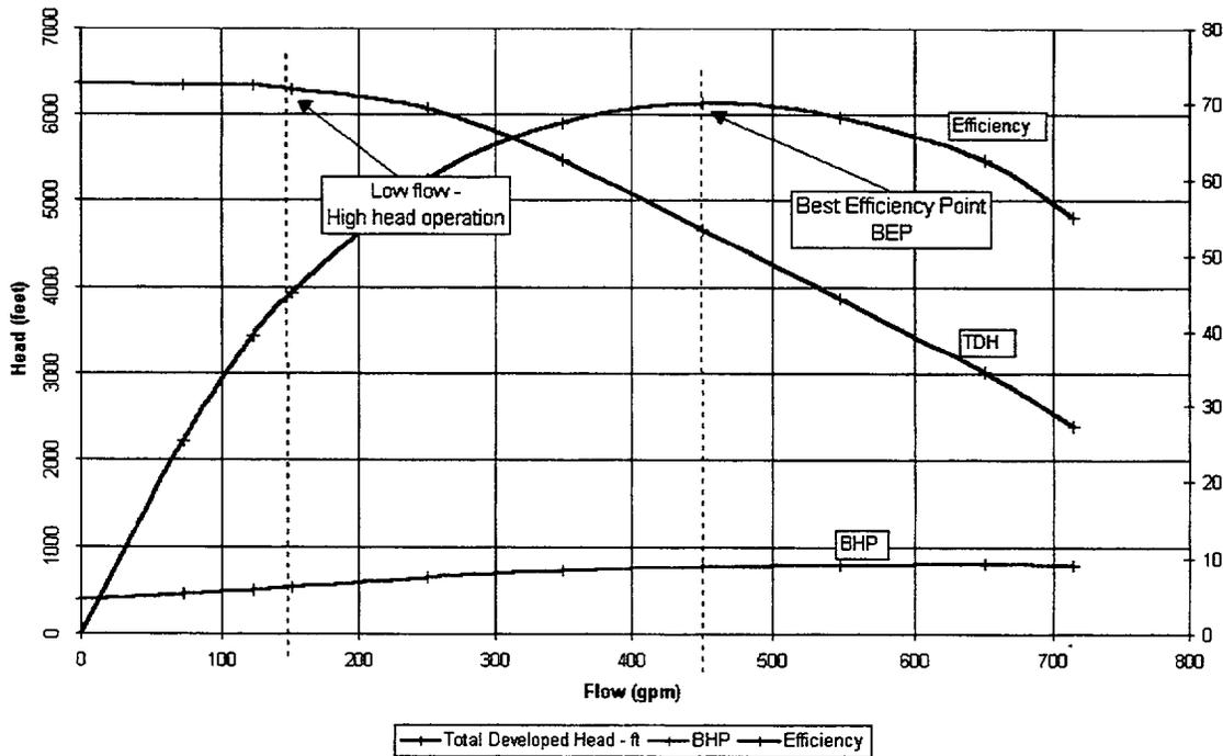
Figure 2. Typical Performance Curve for 900 horsepower Centrifugal Charge Pump, model 25RLIJ-11.
