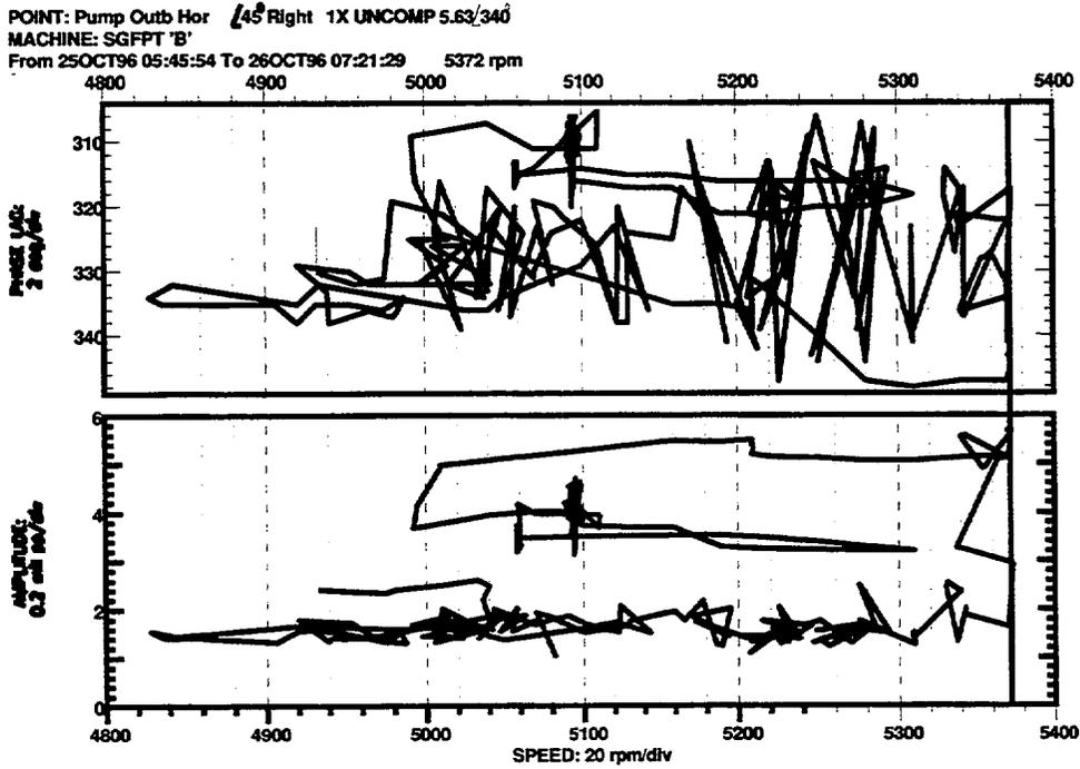
Figure 1. Speed Plot of Step Increase - 2B SGFP Outboard Horizontal Probe
