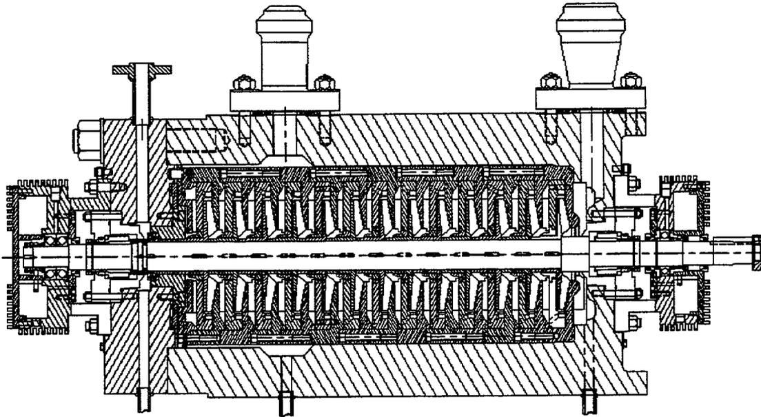
Figure 3. Cross Sectional drawing of Normal Charge Pump (NCP), model 2X10CAM-12.
