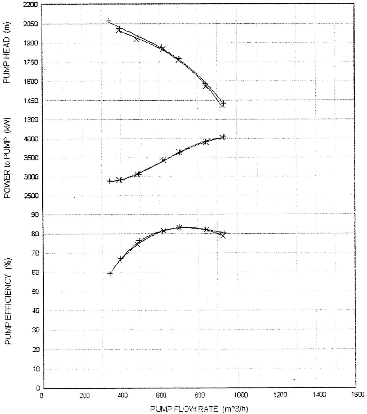
Figure 10. Sea Water Injection Pump
