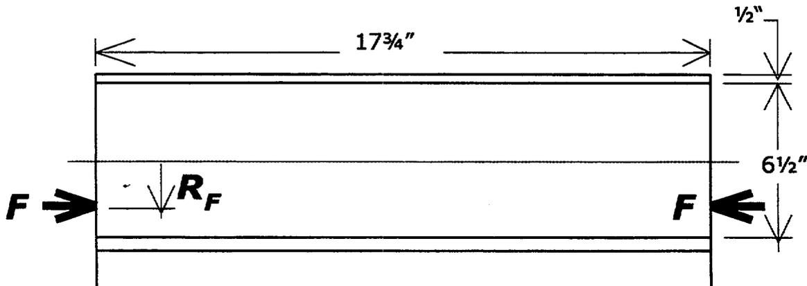
Bowing (Bending) Deflection Over Sleeved Section Of Shaft:
