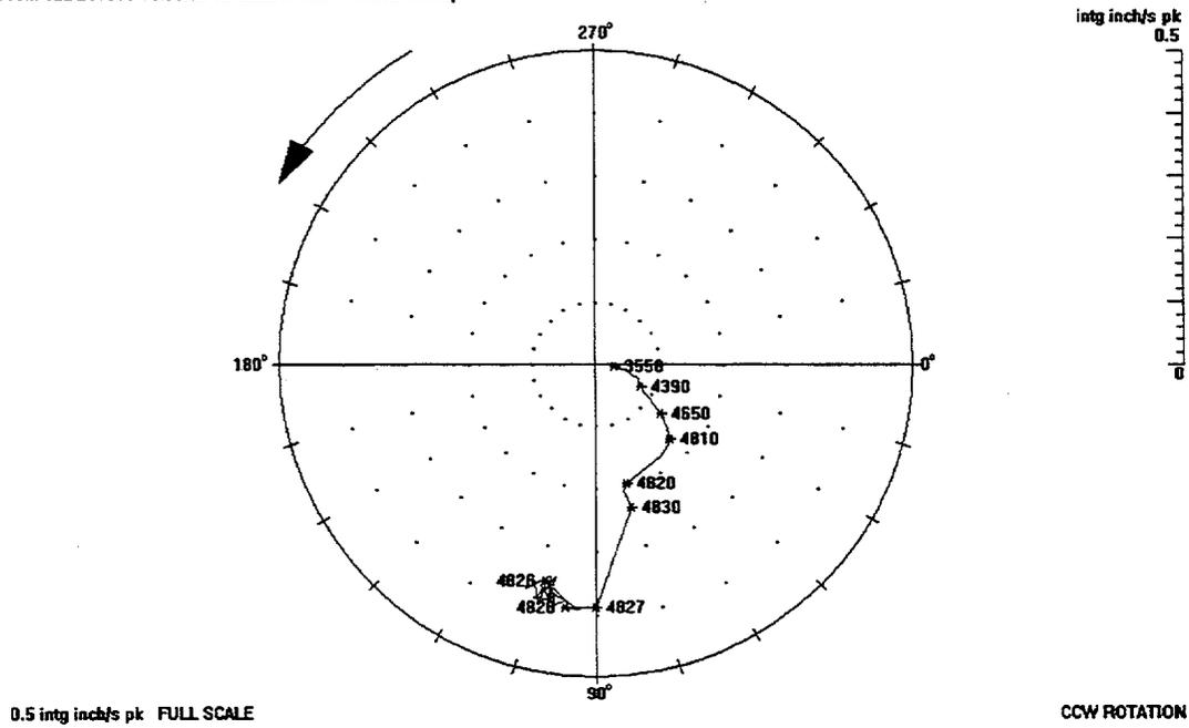
Figure 2. FNP charging pump outboard bearing housing vibration indicating unbalance response
