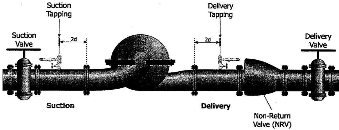
Figure 3 Horizontal Split Case Pump Tapping Arrangement
