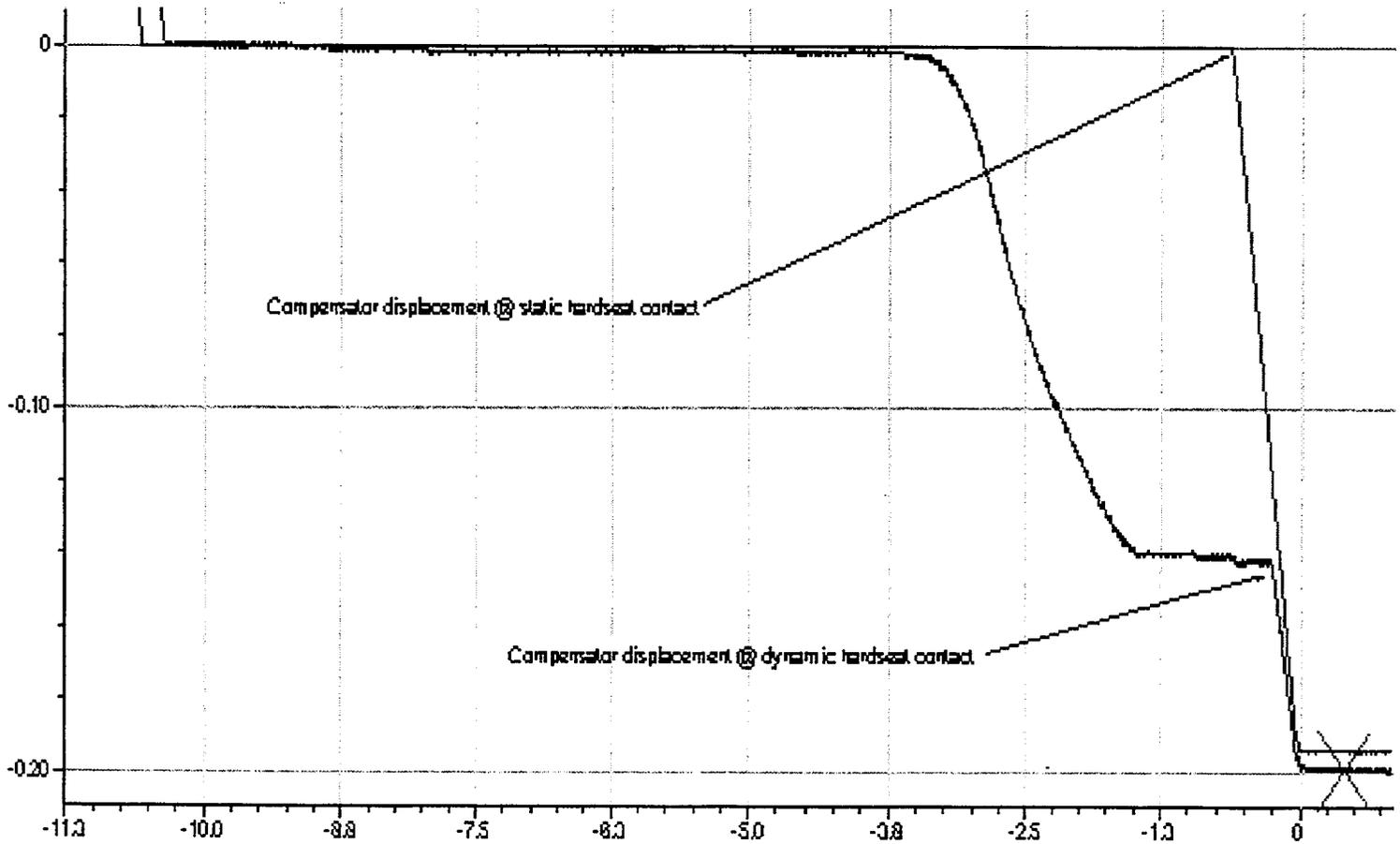
In this case, the total static compensator displacement exceeded the dynamic effect, indicating a proper static setup. Had the compensator movement caused by the dynamic effect been greater than the total static compensator movement, then the valve would not have fully closed.
