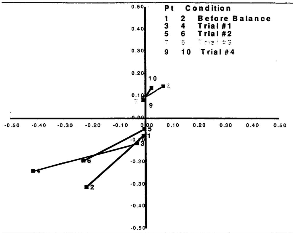
Figure 9. Affect of Trail Balance Weights on Synchronous Vibration
