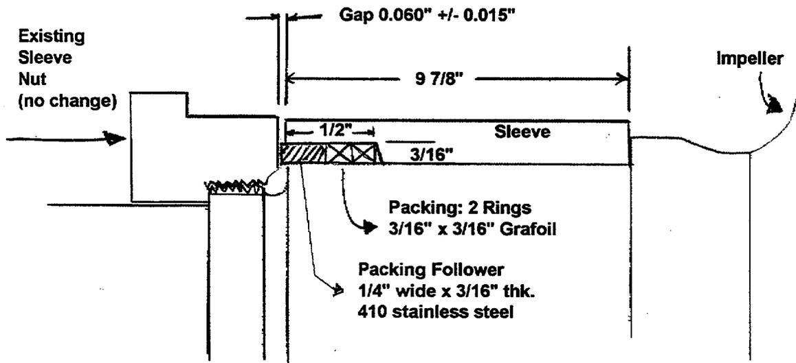
Figure 11. Proposed Modification for Shaft Sleeve and Sleeve Lock Nut
