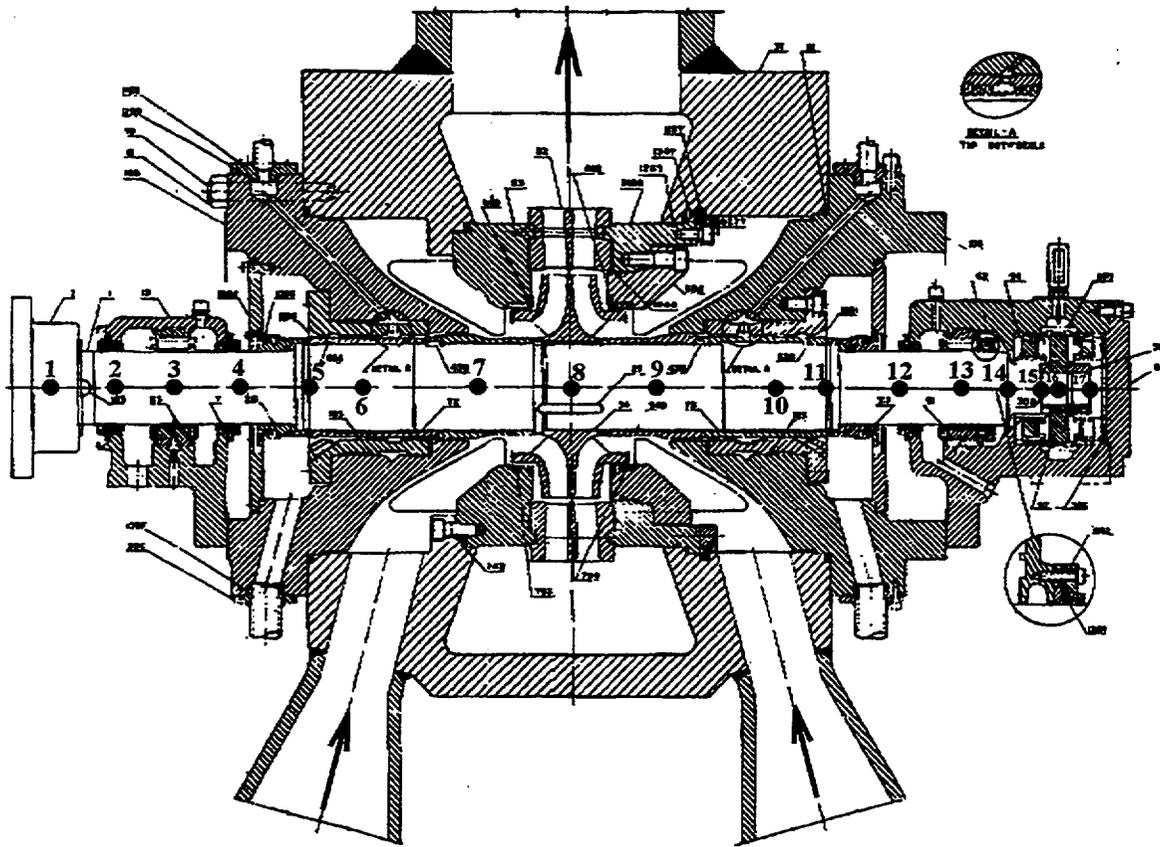
Figure 9. Vogtle feed water pump configuration
