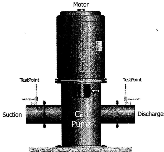
Figure 4 Vertical Can Pump Tapping Arrangement
