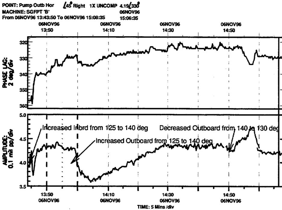
Figure 8. Varying Seal Water Temperature - 2B SGFP
