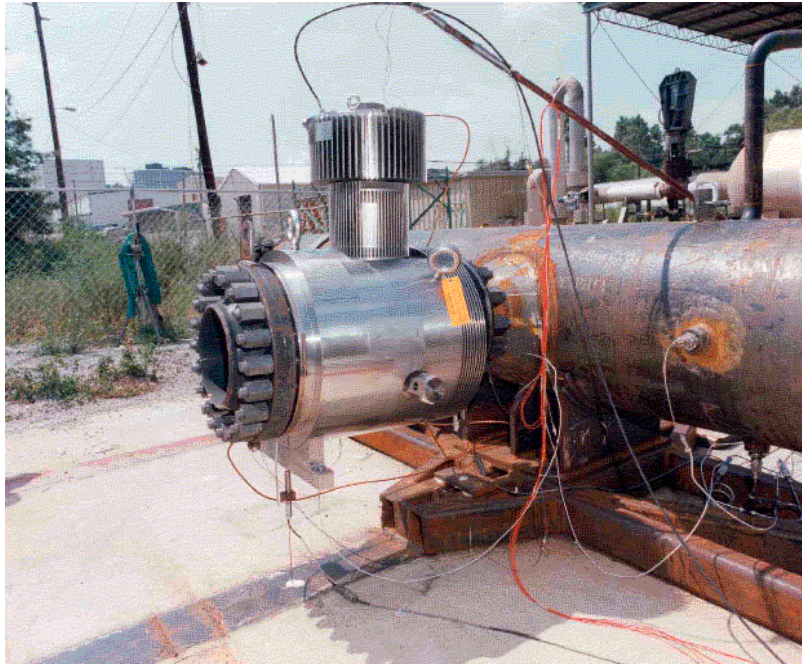
Reactor Depressurization Valve in the Test Facility
