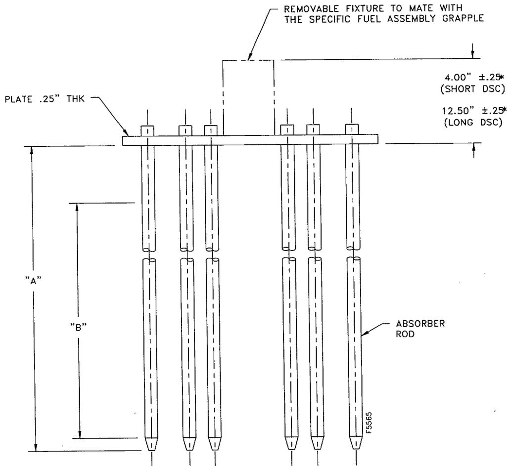
\* THESE DIMENSIONS ARE FOR USE WITH WESTINGHOUSE 17x17 FUEL ASSEMBLIES. DIMENSIONS WILL VARY AS REQUIRED BY FUEL ASSEMBLY TYPE.
