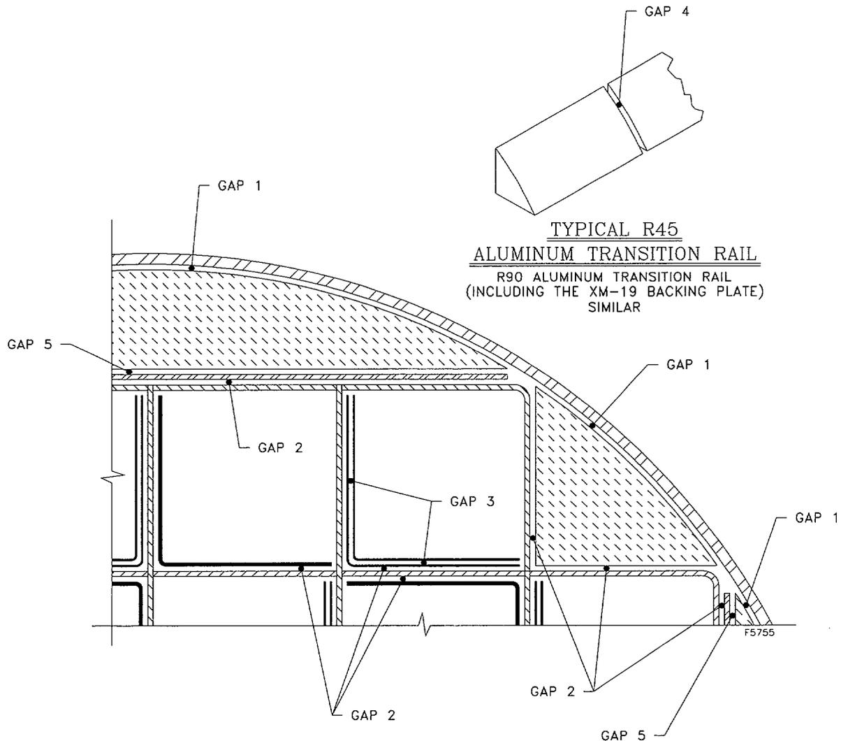
All heat transfer across the gaps is by gaseous conduction. Other modes of heat transfer are conservatively neglected. *Radiation heat transfer is considered in the gap between the DSC shell and aluminum rails only for the 70 °F ambient storage in HSM case.* Heat is transferred through the basket support rails via conduction.
