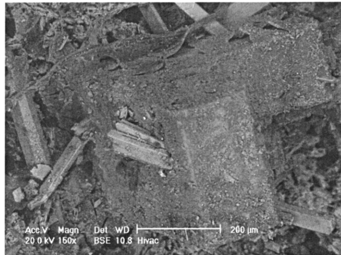
Figure 11.2-7. Photomicrograph of Fracture Minerals in the Karaha-Telaga Bodas System, Indonesia
