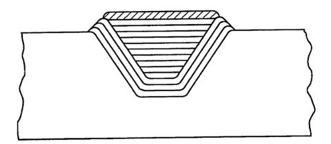
GENERAL NOTE: For ferritic filler metals the completed weld shall have at least one layer of weld reinforcement deposited. This reinforcement shall be removed by mechanical means, so that the finished surface of the weld is essentially flush with the surface of the component surrounding the repair.
