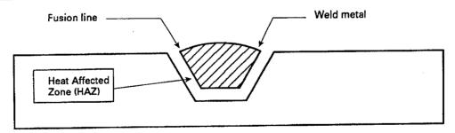
GENERAL NOTE: Base metal Charpy impact specimens are not shown. This figure illustrates a similar-metal weld.
