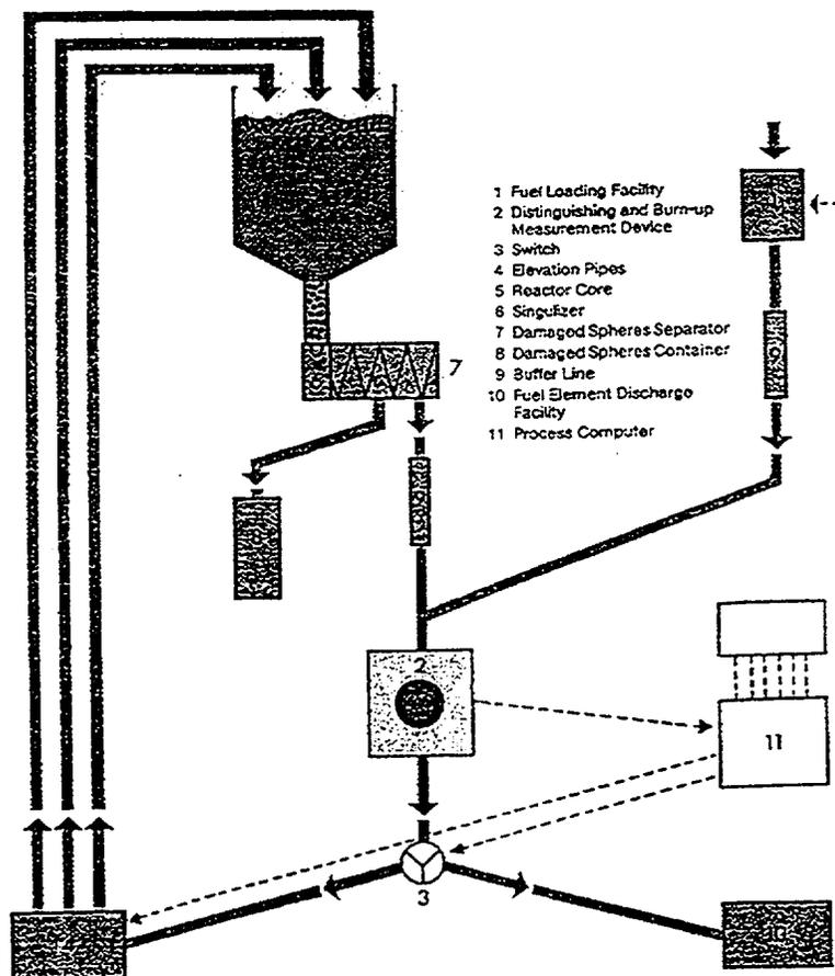
FIG. 2. THTR fuel circulating system
