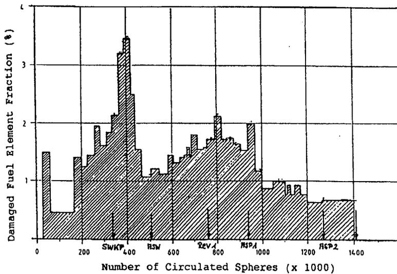
Fig. 10 Fraction of mechanically damaged fuel elements at core exit (measured after size separator)
