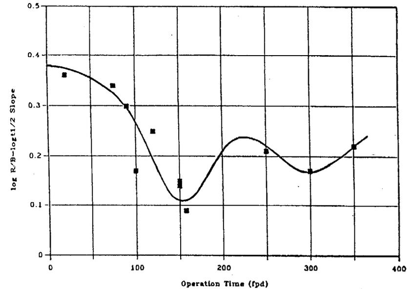
Fig. 8 Development of the  $\log R/B - \log t_{1/2}$  slope during THTR operation
