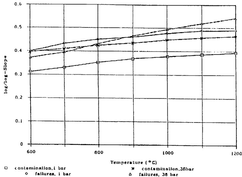
Fig. 5 Slope of log R/B versus log  $t_{1/2}$  of the release models for contamination and failed particles (averaged for all nuclides between  $t_{1/2} = 190$  s and  $t_{1/2} = 6.3$  d)
