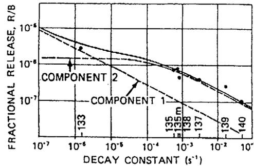
Fig. 2 Calculated and measured xenon release from THTR fuel elements in irradiation experiments at 700 °C, 1 bar (uranium contamination:  $3.0 \cdot 10^{-4}$ )
