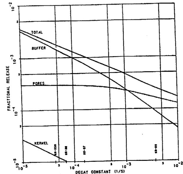
Fig. 4 Calculated krypton release from failed particles in THTR fuel elements at 700 °C, 38 bar
