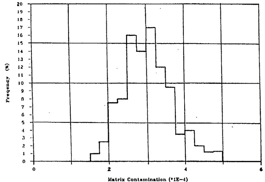
Fig. 1 Distribution of the uranium contamination data for the fuel elements of the THTR initial core (n = 770)
