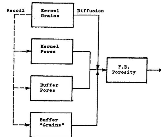
Fig. 3b Gas release from failed fuel particles
