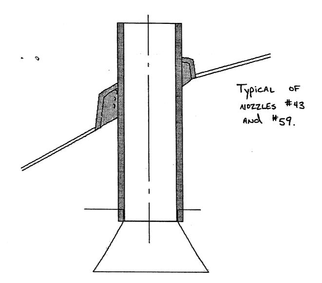
Elevation View of UT Reflectors on ANO-2 Nozzles 43 and 59
