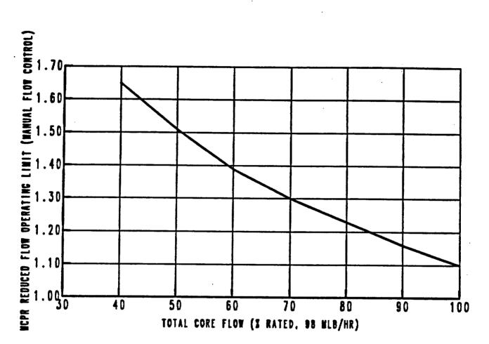
MCPR LIMIT FOR REDUCED TOTAL CORE FLOW
