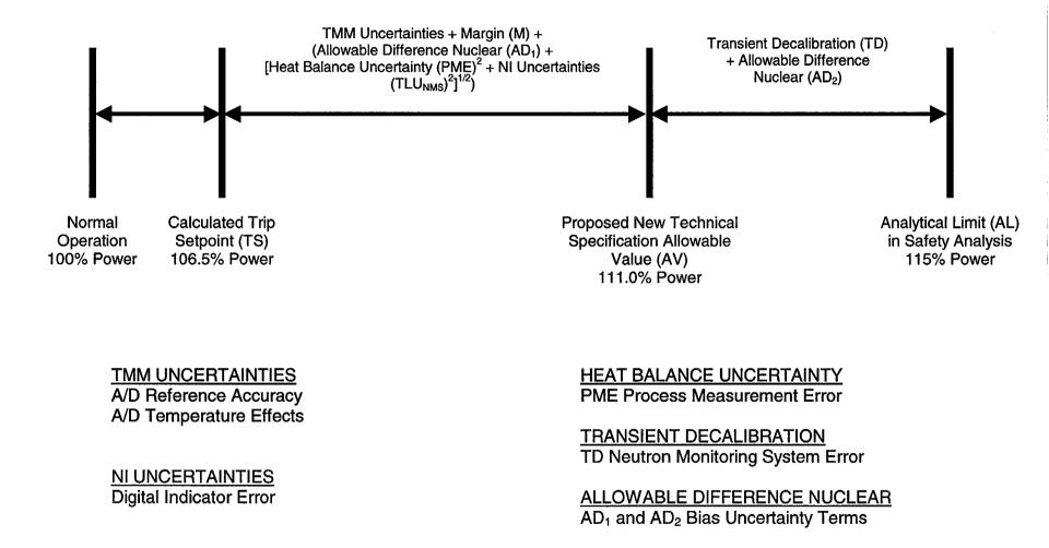
FIGURE 2: Current VHP Trip Calculated Setpoint, and Technical Specification Allowable Value
