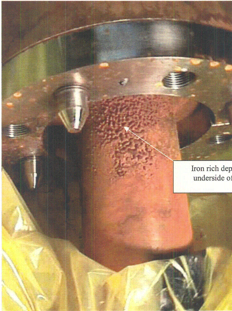
Figure 38. Boric Acid Deposits with Heavy Iron Concentration on Underside of Nozzle 3 (13RFO)
