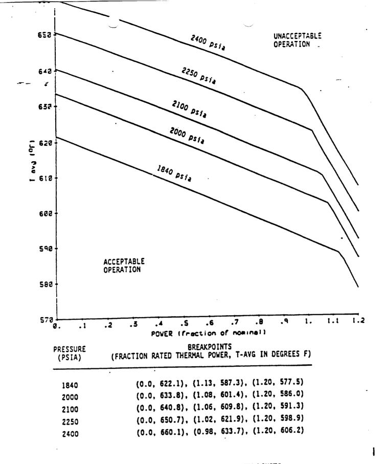
FIGURE 2.1-1 REACTOR CORE SAFETY LIMITS
