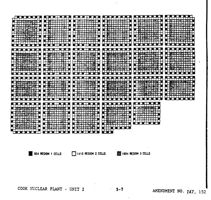
FIGURE 5.6-1: Normal Storage Pattern (Mixed Three Zone)
