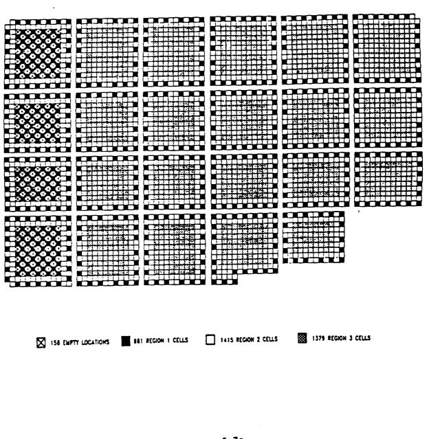
Figure 5.6-2: Interim Storage Pattern (Checkerboard)
