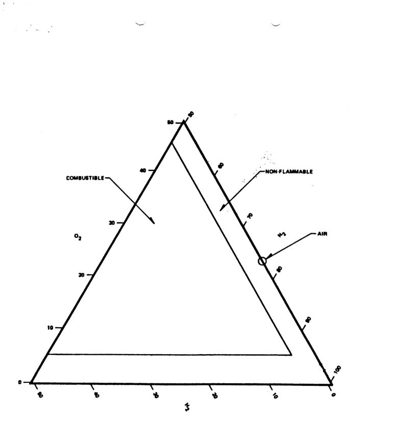
Figure 1. CONCENTRATION OF H<sub>2</sub> AND O<sub>2</sub> REQUIRED FOR COMBUSTION IN A NITROGEN ENVIRONMENT
